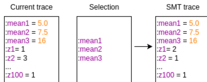
Figure 4.4: Illustration of partial trace optimization, where a selection of variables from the current trace is held fixed and modeled as constraints, while the remaining variables are optimized via SMT
