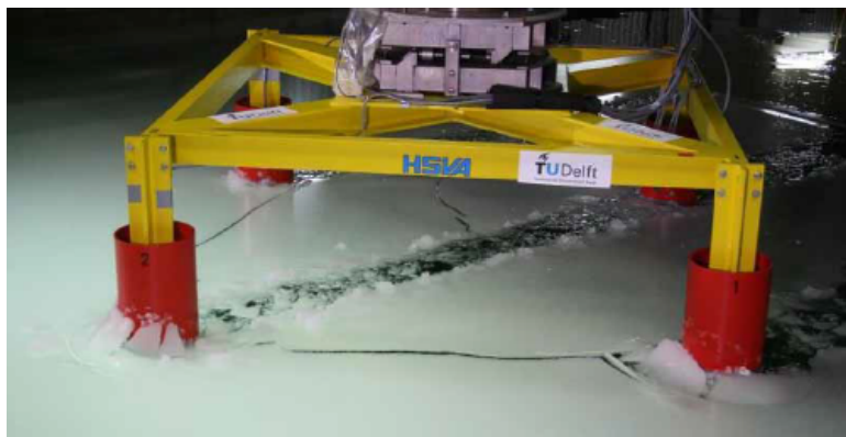
Figure 2.15: Ice splitting during model tests (Hoving et al., 2013).
