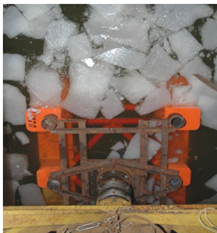
(a) Frontal ice jam of semi-submersible, Q/w \approx 3.9 .
