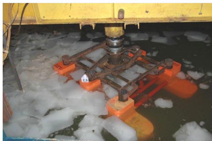
(b) Frontal and central ice jam of semi-submersible.
