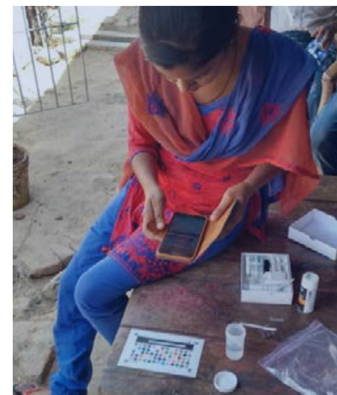
Figure 26, Local households perform strip test with smartphone app. (Picture by A. Mink, 2017).
