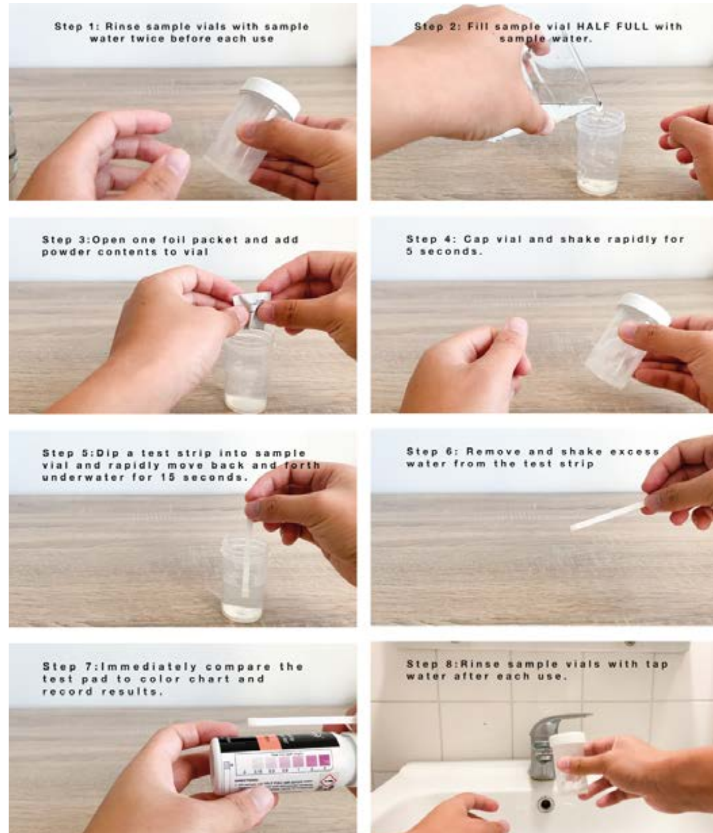
Figure 14, steps of doing HACH IRON test
