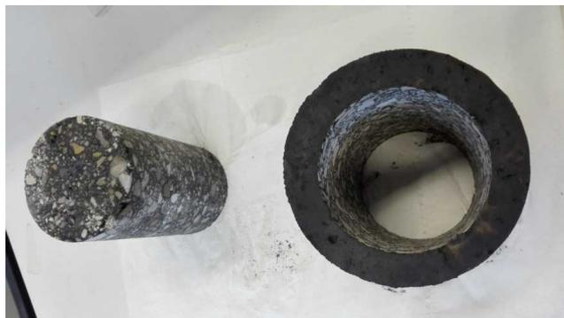
Figure E.1: Cored sample with the remaining outer shell
