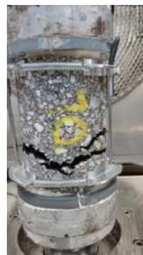
Figure E.5: Specimen 10 after fatigue testing
