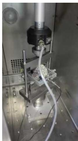
Figure 2.9: MTS CY-ITT test setup with specimen
