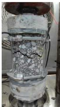
Figure E.4: Specimen 5 after fatigue testing
