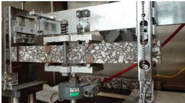
Figure 2.5: TU Delft 4PB test setup
