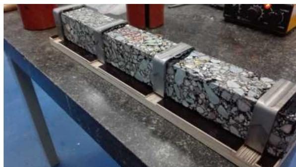
Figure 2.3: 4PB specimen with glued clamps
