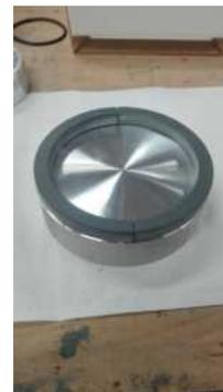
Figure E.3: Aluminium cap and plastic rings
