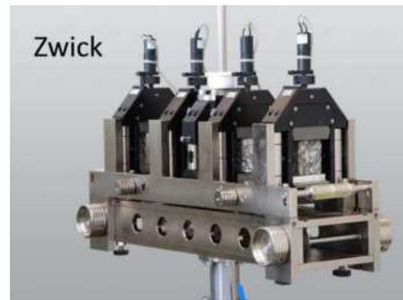
Figure 2.6: Zwick-Roell 4PB test setup
