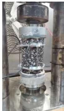
Figure E.2: Test sample installed in the Uni-axial setup
