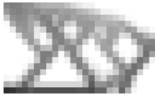
(a) Result from filtering approach for mid loaded cantilever beam with compliance value: 474.55; Volume fraction: 0.24; Number of iterations: 98
