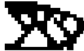
(c) Filtered black-white structure with compliance: 53.88; Volume fraction: 0.5
