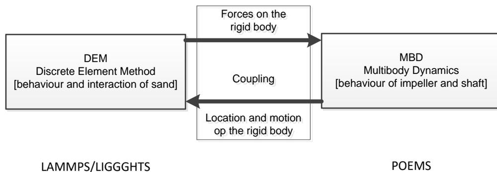
Figure 26. Coupling DEM with POEMS
