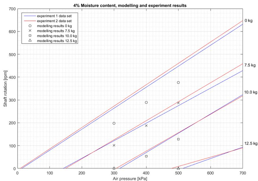
**Figure 37. Comparing modelling and experiment results for 4% moisture content**
