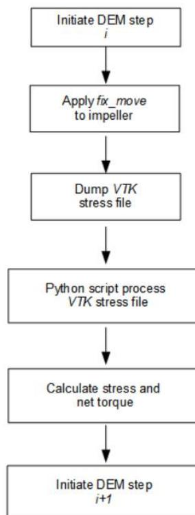
Figure 29. General computational process of the DEM-Rigid body modelling
