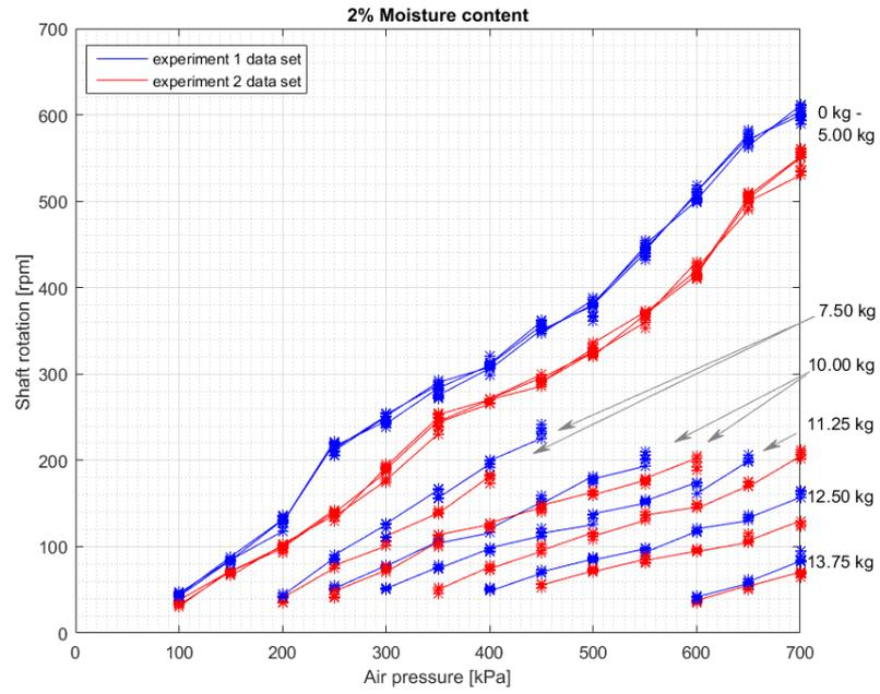
Figure 15. Results for the experiments at 2% moisture content
