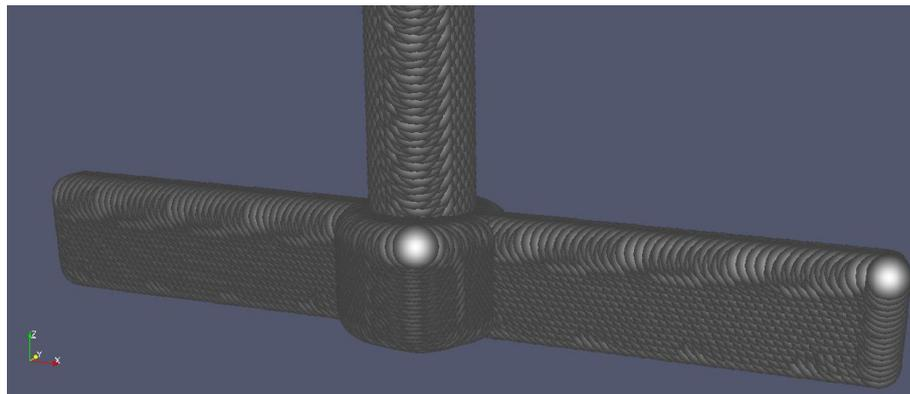
Figure 27. Impeller simulated as spheres
