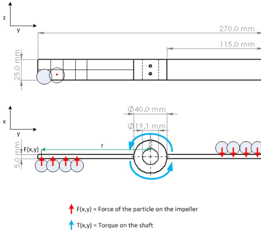
Figure 30. Particles and impeller interaction resulting in torque
