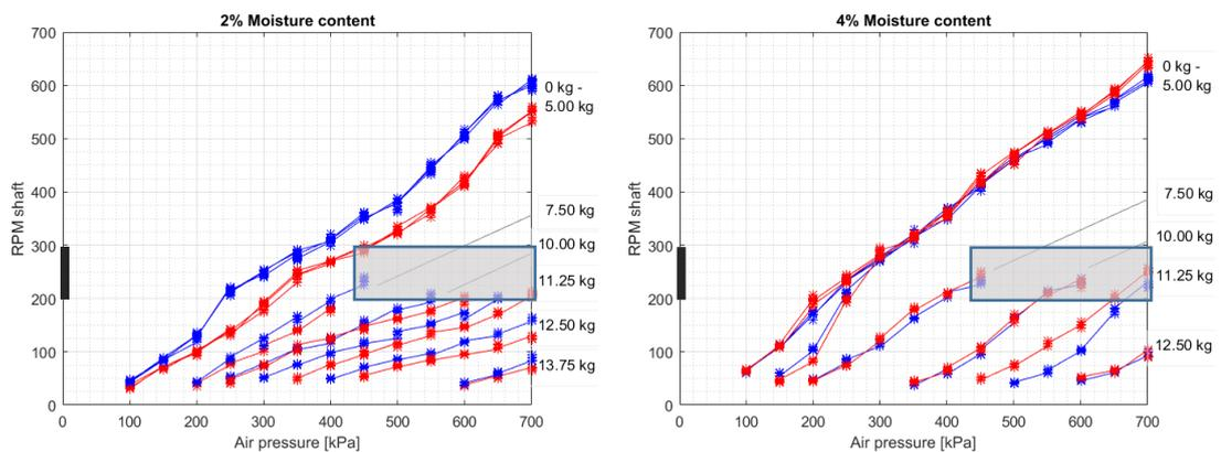
Figure 18. Boxed area where the rotation of the impeller dries the sand for moisture content 2 and 4%
