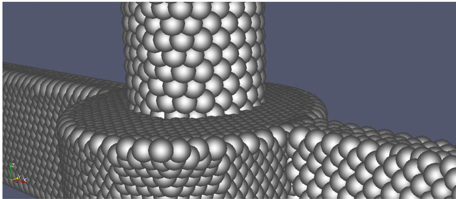
Figure 28. Rigid body formation of the impeller using spheres
