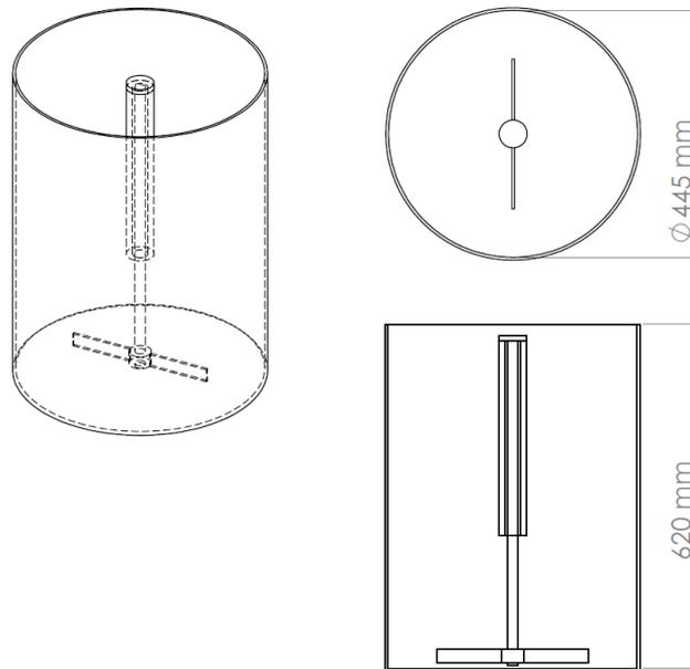
Figure 3. Solidworks 2D drawing of the experimental setup
