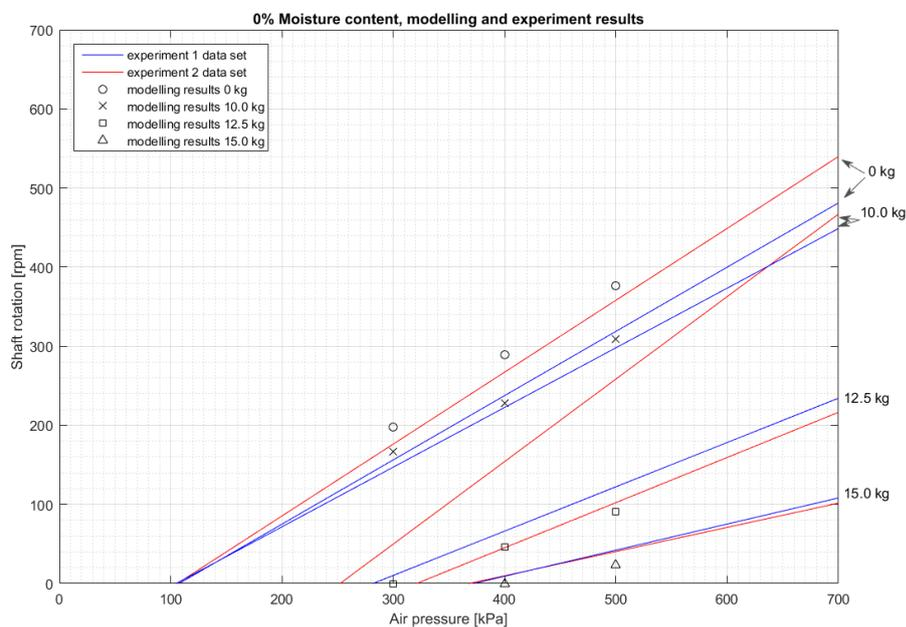
**Figure 35. Comparing modelling and experiment results for 0% moisture content**
