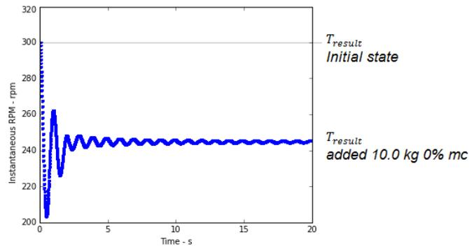
Figure 33. Rpm drop in the steady states at 10.0 kg 0% mc
