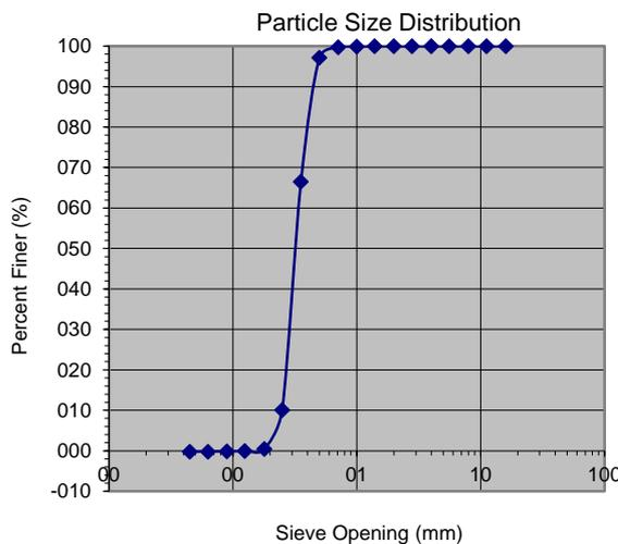
Figure 9. Sand PSD test 1
