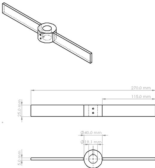
Figure 1. Solidworks Impeller drawing
