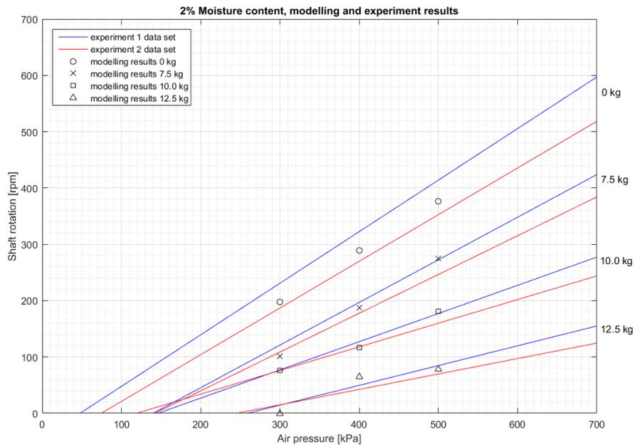
**Figure 36. Comparing modelling and experiment results for 2% moisture content**
