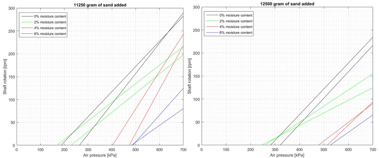
Figure 24. Trendlines for 11250 gram and 12500 gram added sand per moisture content
