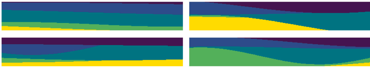
Fig. 4. Synthetic models simulating subsurface layering variability with simple sub-horizontal layering, steep angles, irregular layers, indentations, and complex geometries with lenses and old channels.
