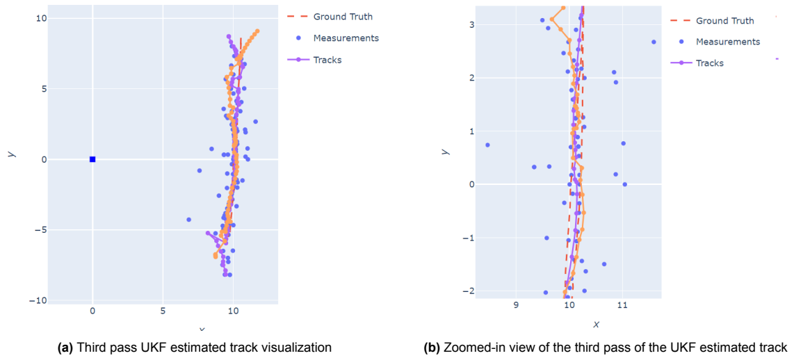
Figure 5.8: Estimated UKF track of a tangential flight, the third pass.
