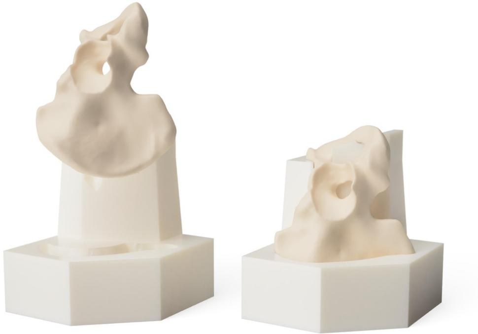
Figure 17: Rendered images of the mould for cyclic testing with the placement of the Sawbones hemipelves.
