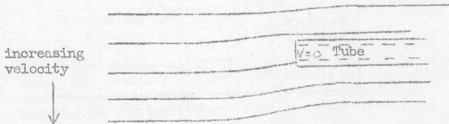
streamline which intersects the mouth of the tube. This stagnation streamline, therefore, does not come from a position far upstream coaxial with the pitot tube, but from a position displaced towards the region of higher velocity.
