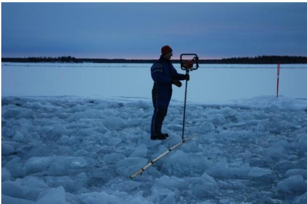
Figure 10-6 Drilling of holes to determine brash ice channel profiles. Extracted from (Westerberg, 2013).
