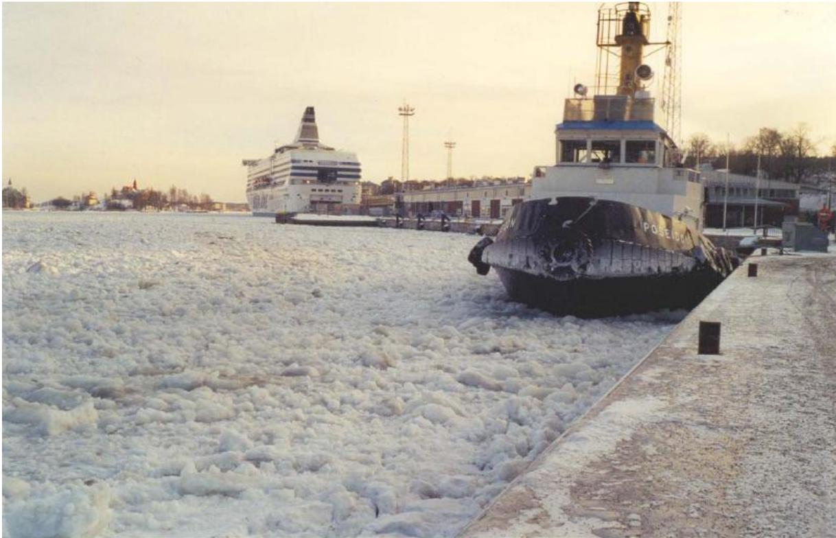
Figure 2-2 Helsinki port, Brash Ice conditions in Helsinki harbour in winter 2003 with 1000 FDD, (Saarinen, Suojanen, & Eranti, 2011)
