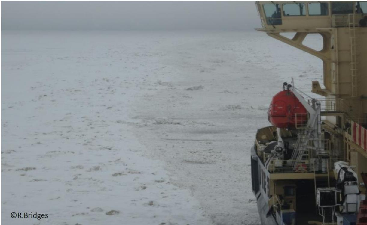
Figure 2-14 Occasionally large broken ice floes pulled from the channel edge into the centre, from the icebreaker and ship wake
