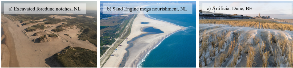
Figure 2.1.: Three dune intervention projects with varying objectives: Five foredune notches at National Park Zuid-Kennemerland excavated to reintroduce dune dynamics (a), the 21 Mm 3 Sand Engine mega nourishment, constructed to stimulate dune development (b) and artificial dune constructed in front of an existing seawall to limit sand nuisance (c).
