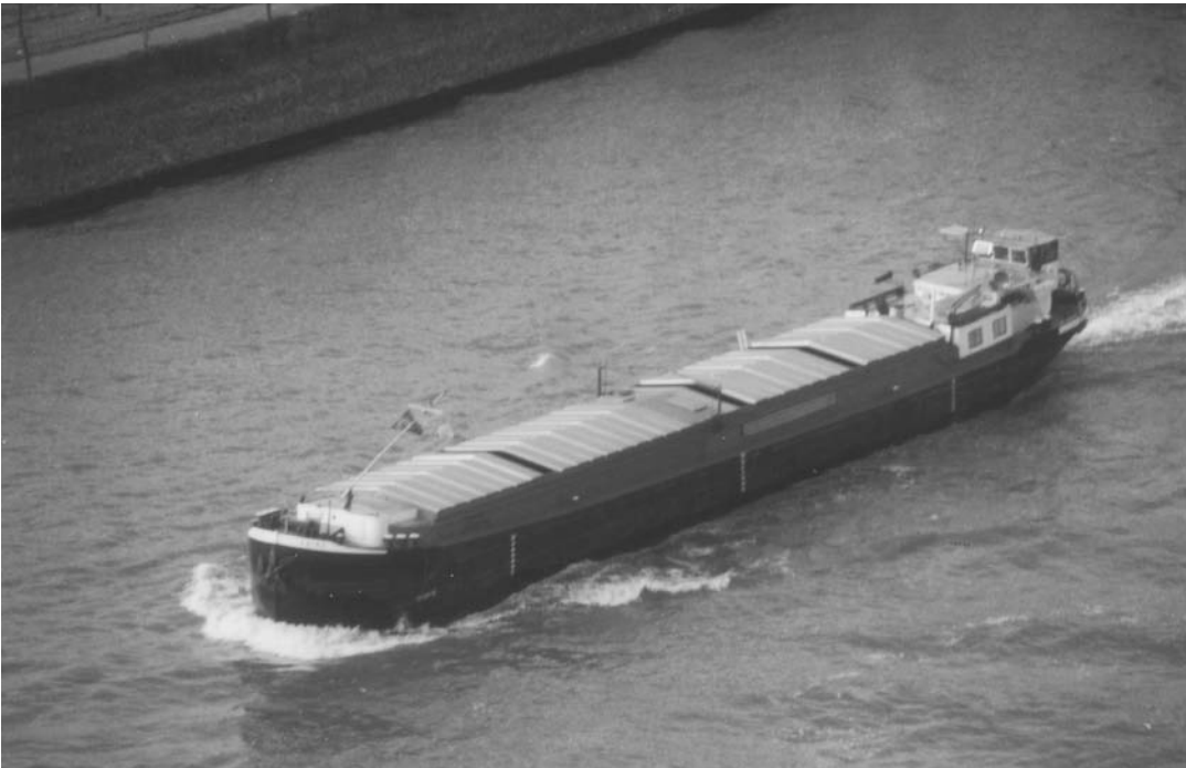
Photo 4.7 Motor cargo vessel CEMT class II (Kempenaar - Campinois)
