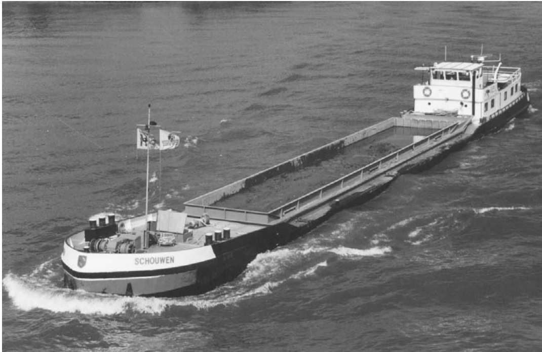
Photo 4.8 Sand/ballast barge CEMT class IIa
