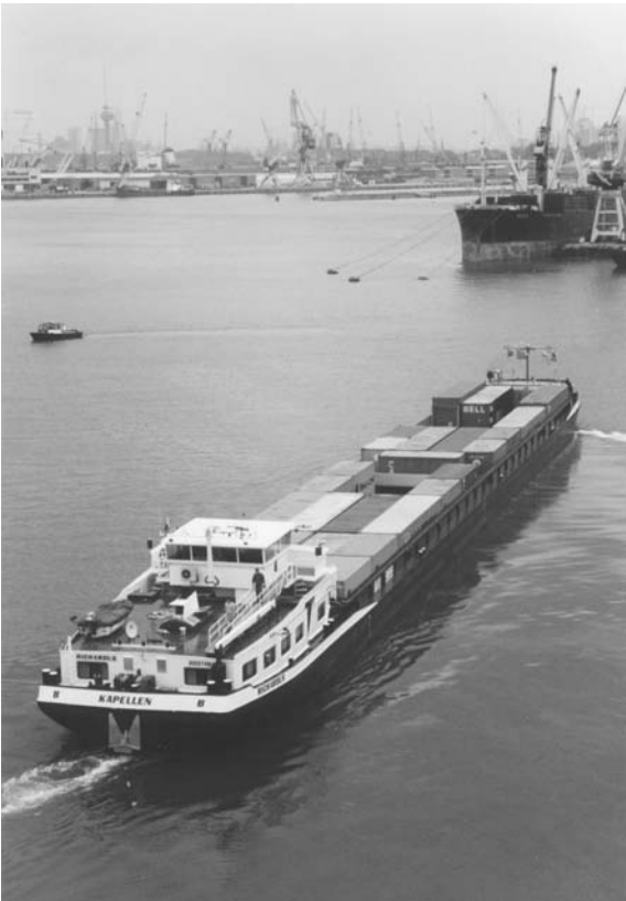
Photo 4.15 Container vessel CEMT class Va (Big Rhine barge)
