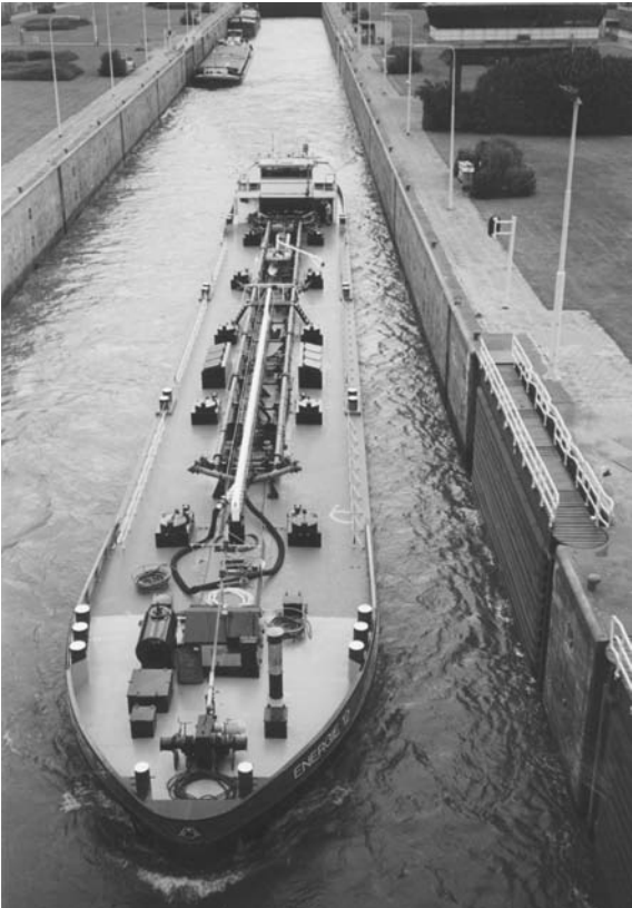
Photo 4.14 Motor tanker CEMT class IV
