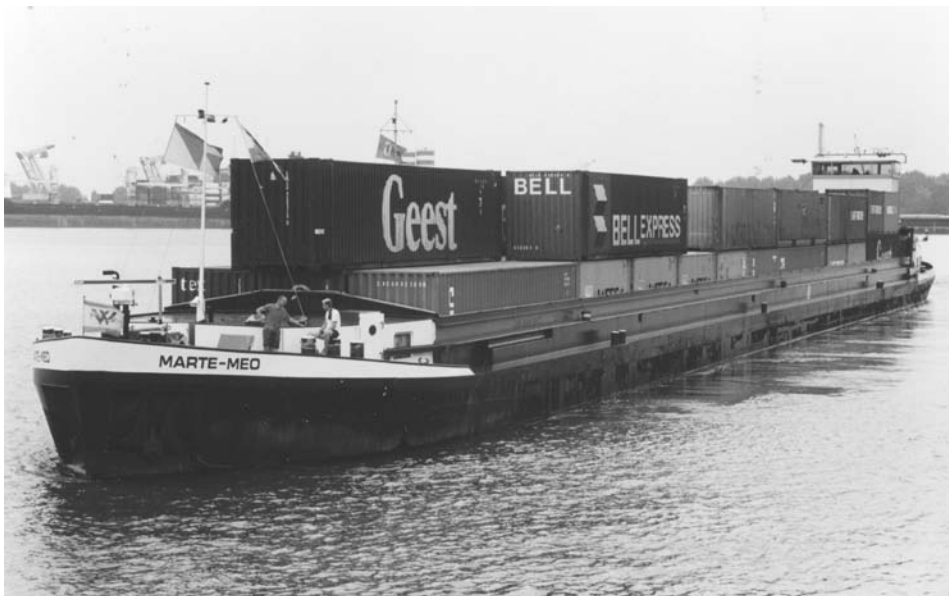
Photo 4.11 Container vessel CEMT class IIIa
