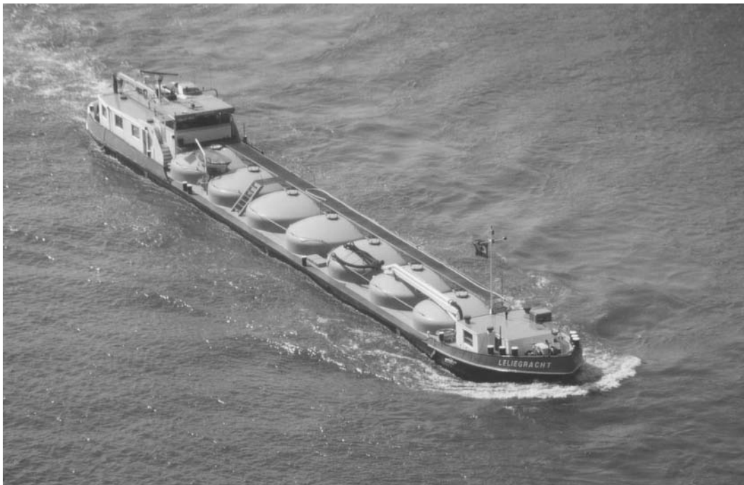
Photo 4.9 Cement tanker CEMT class IIa
