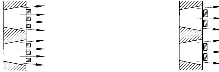
Vertical energy dissipating bars (horizontal cross section) Vertical energy dissipating bars (horizontal cross section)
