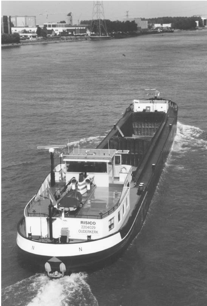
Photo 4.10 Motor cargo vessel CEMT class III (Dortmund-Ems-Canal)
