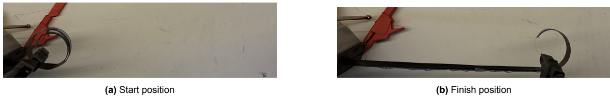
Figure 5.13: Start and finish positions of the single-wire spacer setup
