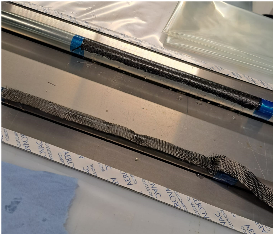
Figure 4.8: Springs three and four during layup demonstrating tape-down and folding technique
