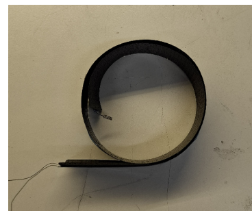
(b) Stable rolled configuration when spacer tape is applied to a curved tape spring
