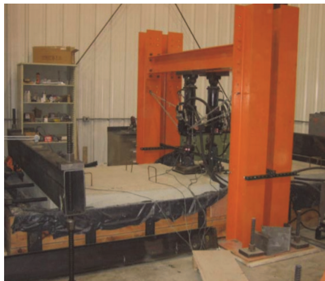
Figure 2. Large scale test set up for evaluating load transfer efficiency [19]
