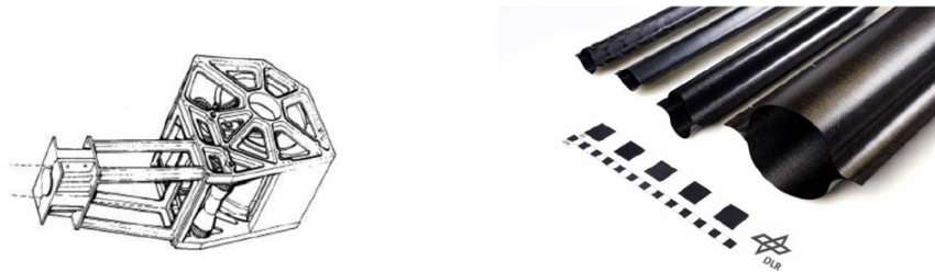
Figure 3.21: Coiled composite boom (Left) and composite boom designs (Right) [52]
