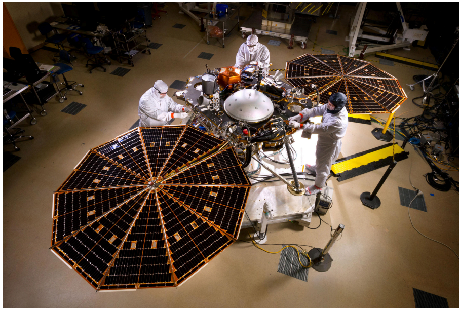
Figure 3.11: Image of the Insight lander with its two Ultraflex solar arrays. Photo courtesy of NASA/JPL-Caltech/Lockheed Martin
