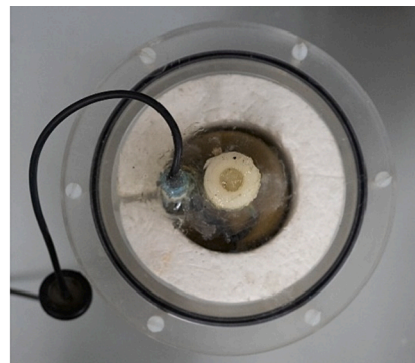
Fig. 3. Calorimetric unit of JAF60 isothermal calorimeter.
