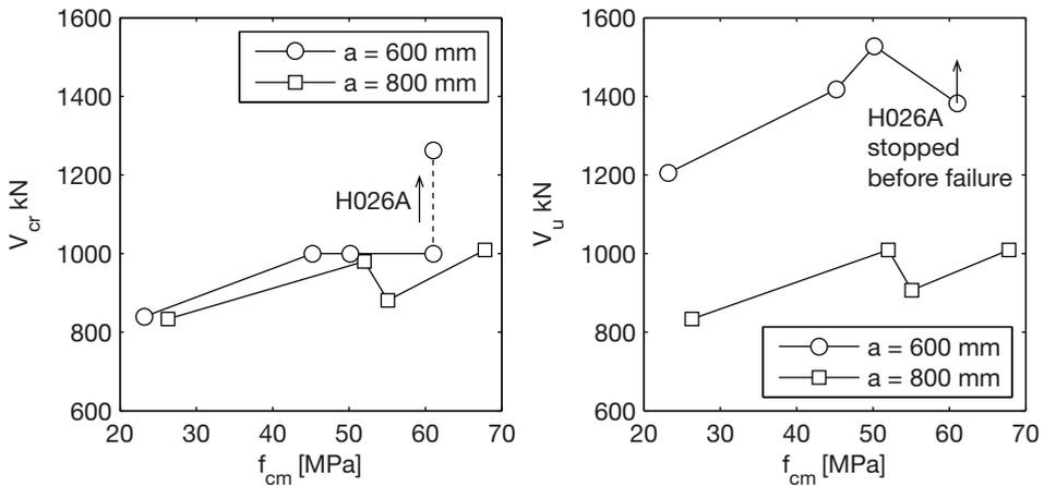
**Fig. 6.21.** Relationship between concrete mean strength  $f_{cm}$  and inclined cracking force  $V_{cr}$  (left) and ultimate shear capacity  $V_u$  (right).
