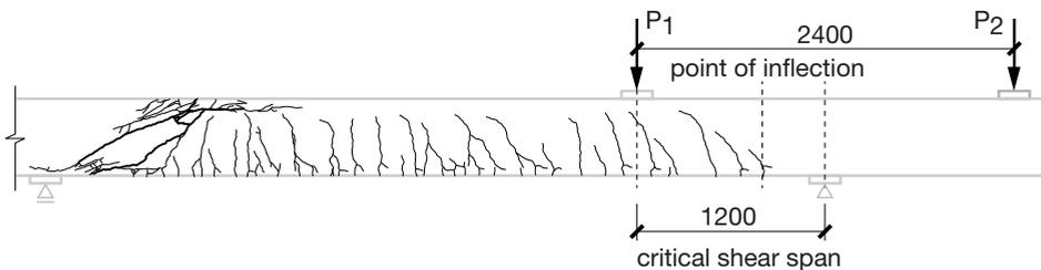
**Fig. 6.4.** Crack pattern of C11b123 before loading.
