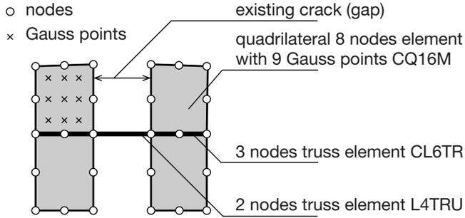
**Fig. 3.15.** Detail of elements at the existing crack, the name of the elements being defined in Diana, see Diana Manual (TNO-DIANA 2011).
