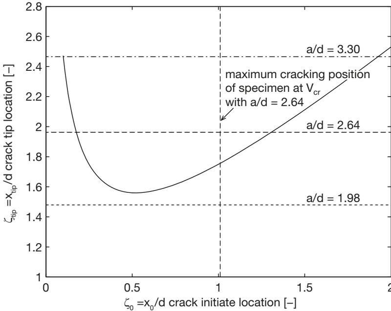
**Fig. 3.42.** Relationship of crack tip location and crack initiation location according to Eq. (3.19).
