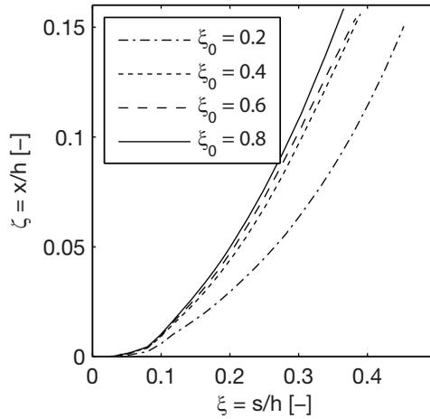
**Fig. 3.24. Influence of existing crack height  $\xi_0$  to the crack path.**
