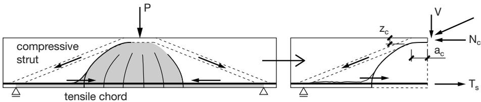
**Fig. 3.39.** Load bearing structure of a beam after inclined crack developed.
