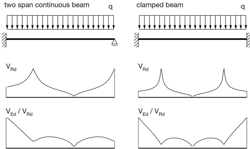
**Fig. 5.19.** Distribution of  $V_R$  and  $V_E/V_R$  under statically indeterminate beams.
