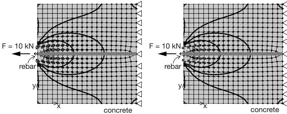
**Fig. 3.4.** Comparison of principal stress distribution of reinforcement-concrete interaction with perfect bond model (left) or with the bond mode model according to (fib 1993) (right), calculated by Atena2D.
