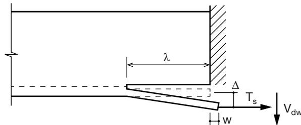
Fig. 3.37. Detachment of a tension bar attached to a deep beam.
