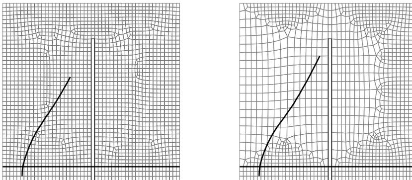
**Fig. 3.17.** Influence of mesh size to simulated crack paths from SLA ( $x_0 = 600$  mm).
