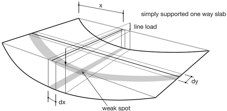
**Fig. 6.26.** Simplified model to consider the influence of weak spot in a one way slab.
