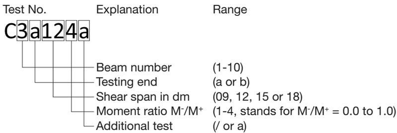
Fig. 5.9. Illustration of test identifying rules.
