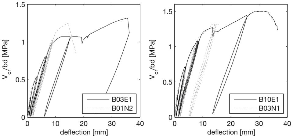
**Fig. 6.16.** Comparison of shear stress - deflection relationships between old and new beams.
