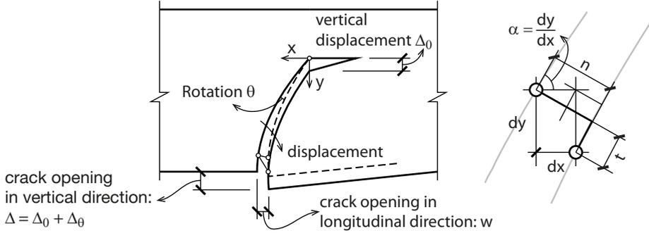
**Fig. 3.26. Kinematic conditions of a crack.**
