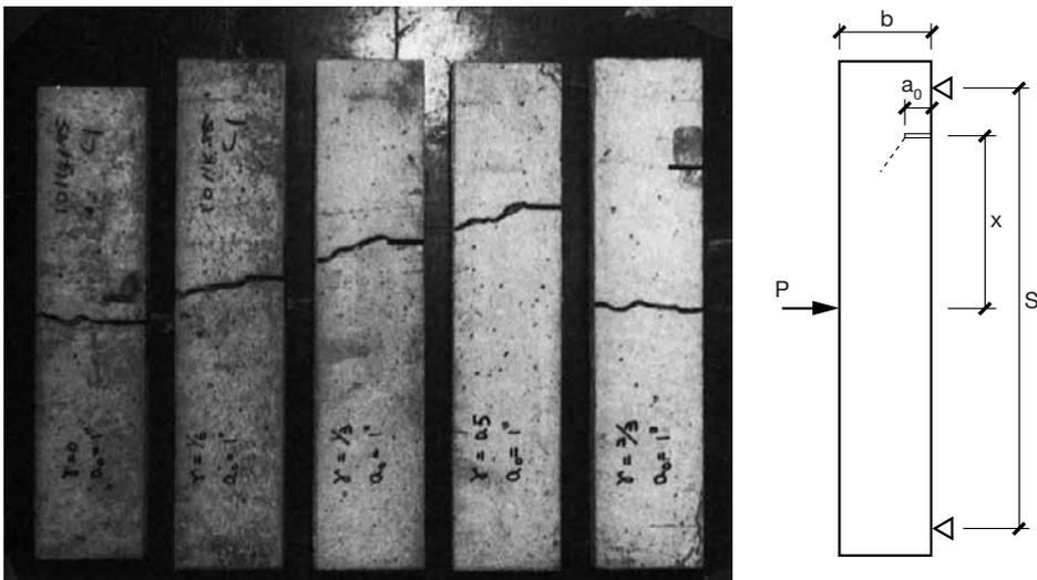
Fig. 3.7. Crack patterns of specimens with different crack initiating location in Jenq and Shah's tests (Jenq & Shah 1988). The notations of the dimensions are according to the original paper. The values of them can be found in the original paper.
