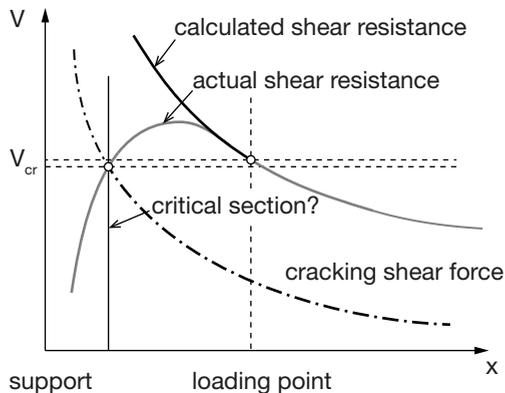
**Fig. 7.1.** Determination of the critical section in a span with relatively small shear slenderness ratio.
