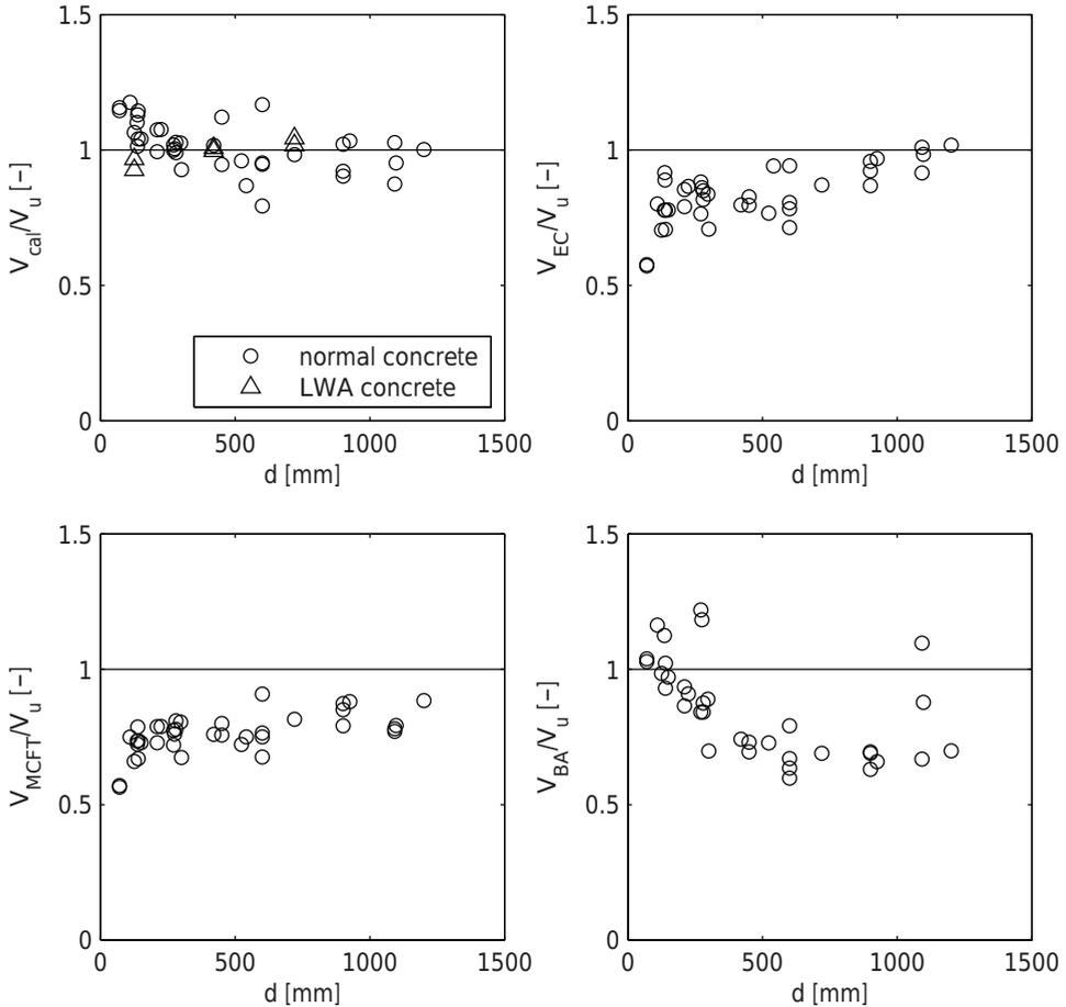
**Fig. 4.32.** Influence of beam depth on model prediction accuracy (top left: Present Theory; top right: Eurocode; bottom left: Modified Compressive Field Theory; bottom right: Bažant's formula).
