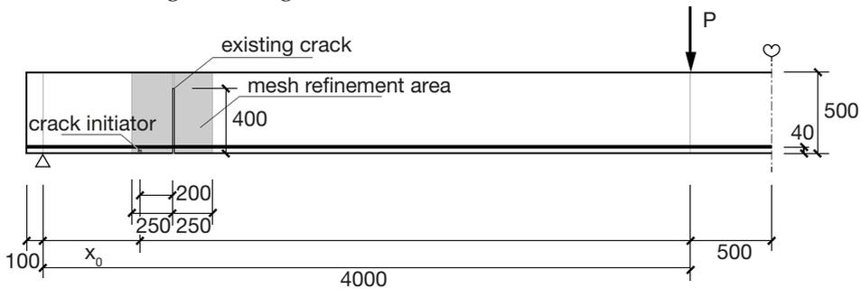
Fig. 3.14. Sketch of the model configuration.
