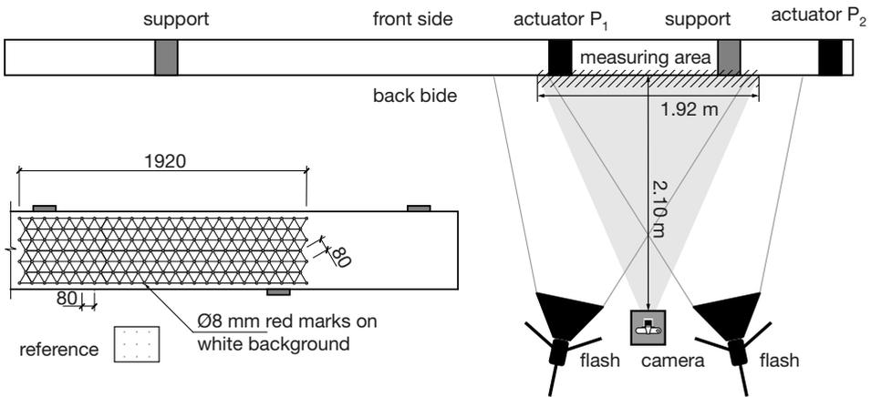
Fig. 5.8. Setup of photogrammetry measurement and mesh arrangement.
