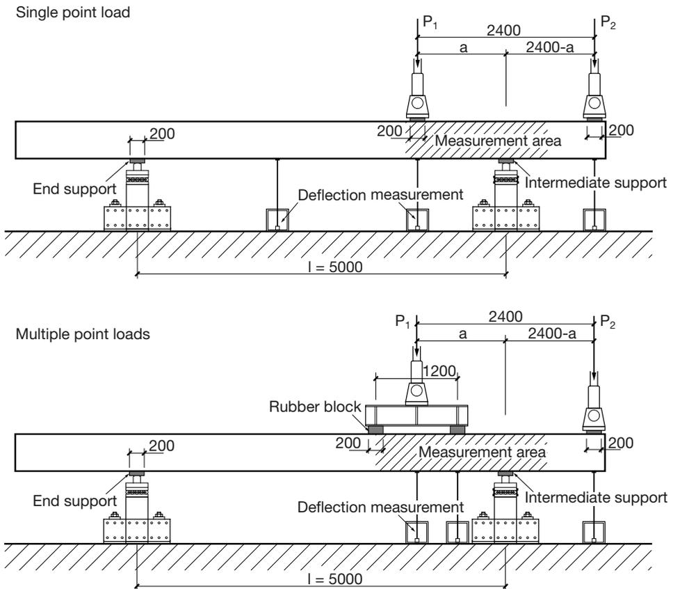
Fig. 5.5. Sketches of test setups with single point load and multiple point loads.
