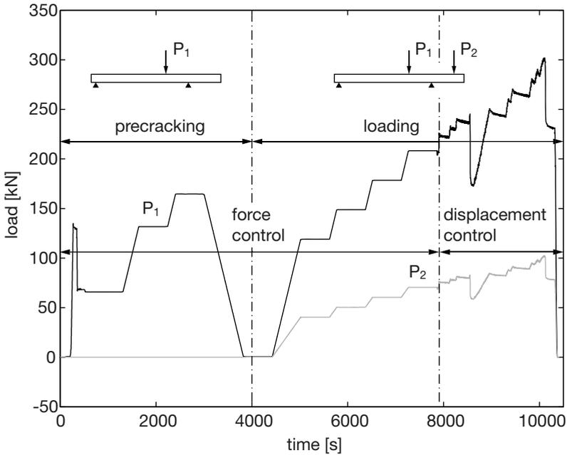
Fig. 6.5. Loading procedure of test C16b123.
