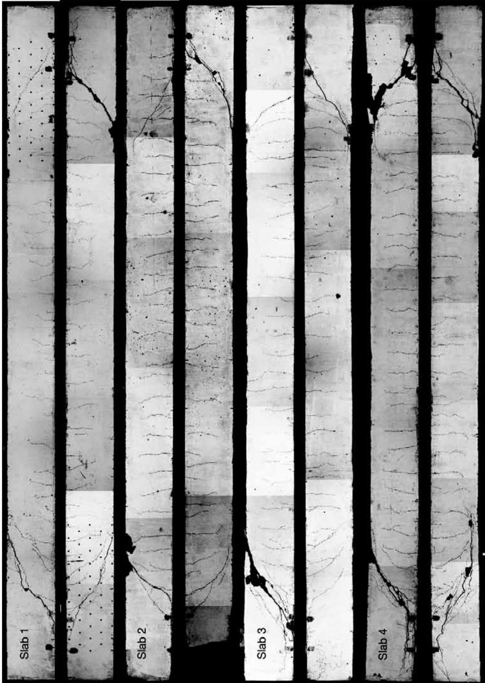
Fig. 6.25. Comparisons of crack patterns of side surfaces of slab 1-4 after failure.
