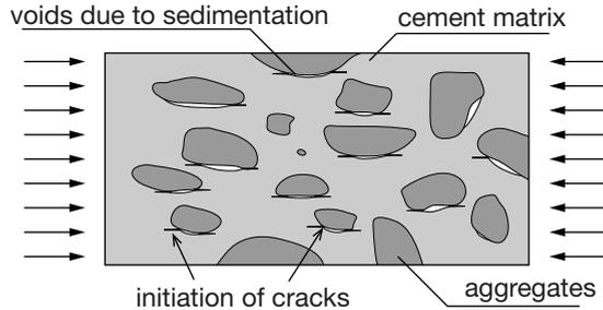
**Fig. 6.13.** Cracks generated by sedimentation voids under aggregates during compressive tests.
