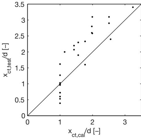
**Fig. 5.33.** Comparison of measured critical section and critical section used in the calculation.
