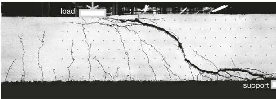
**Fig. 3.34.** Crack pattern of a concrete beam with  $M/Vd = 3.0$  after failure. Specimen C2b151 from continuous beam tests, from (Yang & den Uijl 2011).
