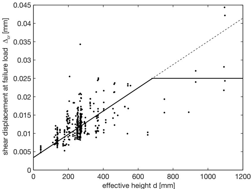
Fig. 4.11. Calculated critical vertical displacement against effective height.
