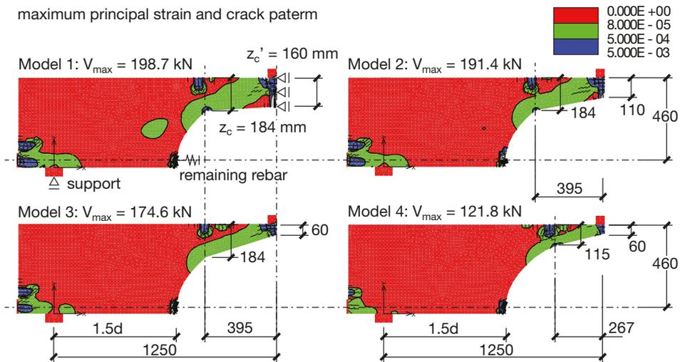
**Fig. 3.41.** Maximum principal stress distributions and crack patterns of FEM models of arch structure with different horizontal crack branches profiles.
