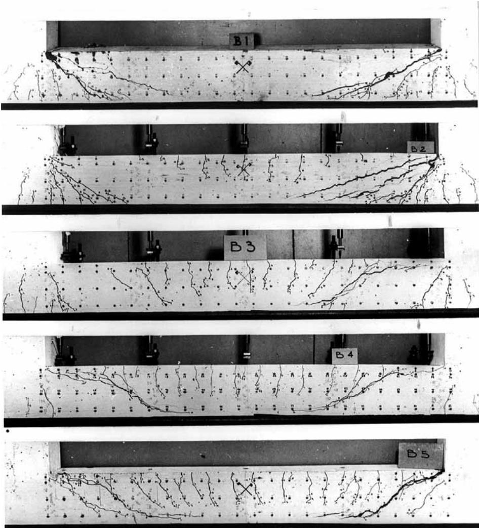
**Fig. 5.35.** Crack pattern of test series B after failure.  $l = 1350$  mm, from B1 to B5,  $m = 0.00, 0.25, 0.50, 0.75$  and  $1.00$  respectively (IBBC-TNO 1985).
