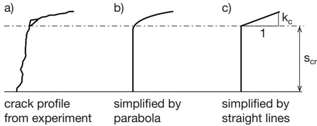
**Fig. 4.2.** Crack profile simplifications, based on the crack profile found in test D18a121 (see Fig. 5.13).
