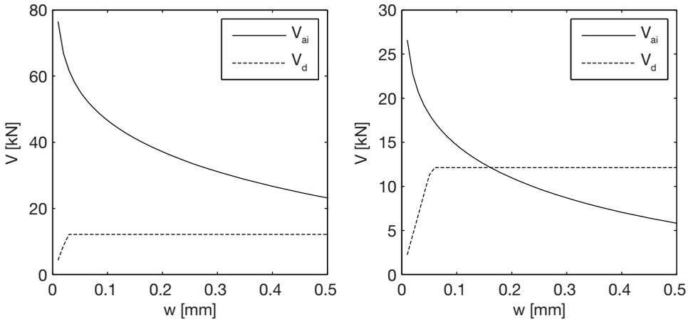
Fig. 3.32. Relationship between crack width and shear force carried by aggregate interlock  $V_{ai}$  and dowel action  $V_d$  (left:  $M/Vd = 1.0$ , right:  $M/Vd = 2.0$ ).
