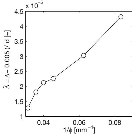
**Fig. 4.21.** Relationship between rebar diameter and critical shear displacement  $\Delta_{cr}$ .
