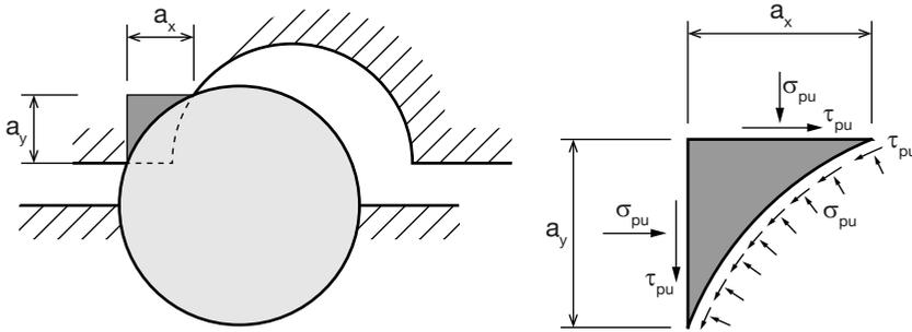
**Fig. 2.5.** Schematic model for the mechanism of aggregate interlock (Walraven 1981).
