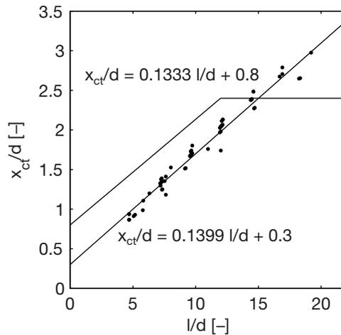
**Fig. 5.24.** Comparison between the calculated critical sections based on tests reported in (Leonhardt & Walther 1962; Krefeld & Thurston 1966) marked as dots with the simplified model and the regression formula Eq. (5.9).
