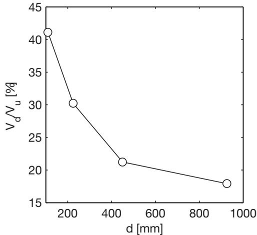
**Fig. 4.28.** The influence of beam depth on the contribution of dowel action in the ultimate capacity as reported by (Collins & Kuchma 1999).
