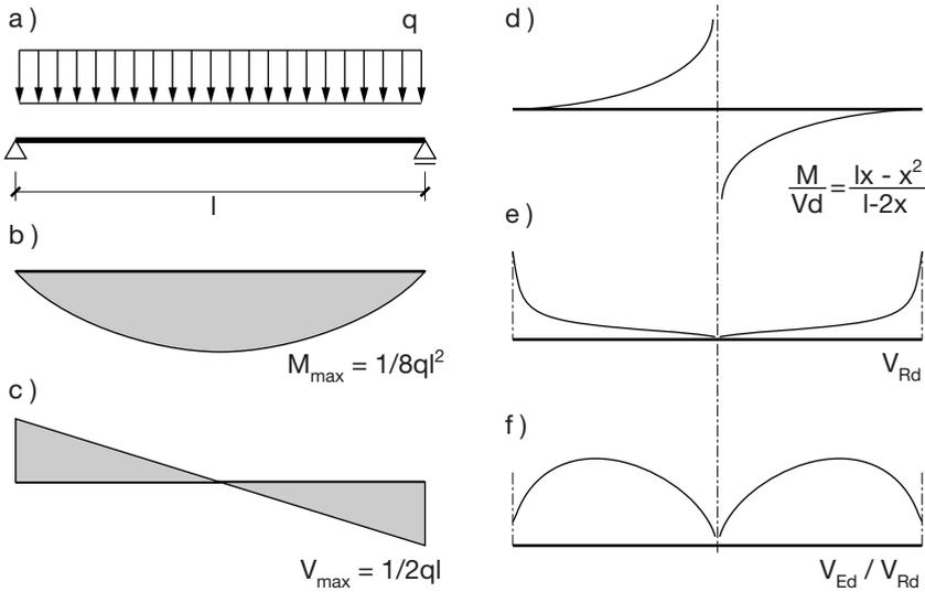
**Fig. 5.17.** Calculation of shear capacity along simply supported beam loaded by a uniformly distributed load. (a) Boundary conditions. (b) Moment distribution. (c) Shear force distribution. (d)  $M/Vd$  distribution. (e) Shear resistance assuming straight crack path. (f) Shear force over shear resistance.
