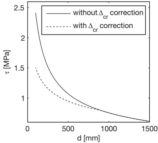
**Fig. 4.30.** Influence of  $\Delta_{cr}$  correction on the size effect relationship ( $f_{cm} = 40$  MPa,  $M/Vd = 3.0$ ,  $\rho_s = 0.9\%$  with 3 rebars).
