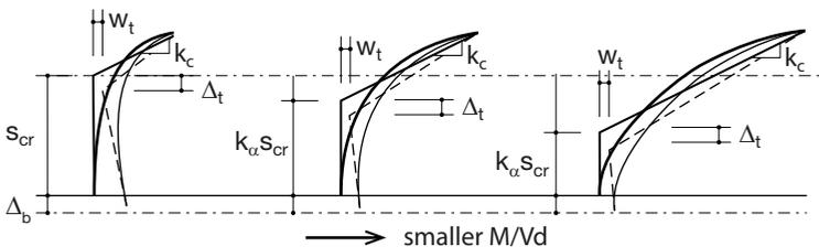
Fig. 5.22. Simplifying curved crack profile by bilinear profile with vertical major crack.
