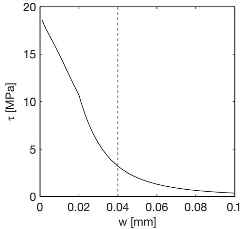
**Fig. 4.8.** Shear stress as a function of crack width  $w$  at  $\Delta = 0.02$  mm.
