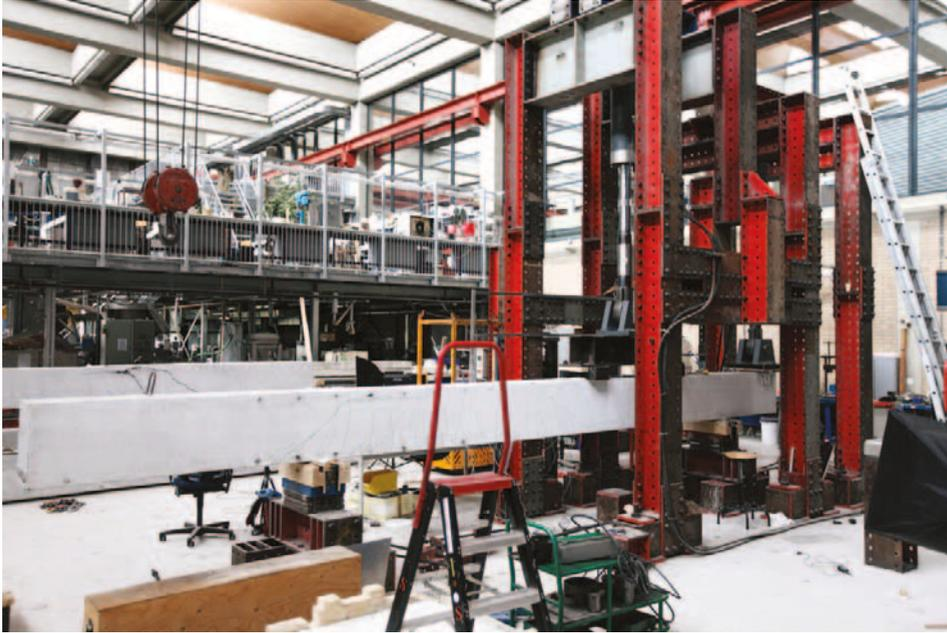
**Fig. 5.4.** Photo of the test setup with multiple point loads in the main span.
