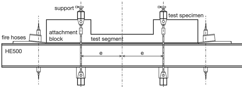
**Fig. 5.31.** Test setup of TNO shear tests under uniformly distributed load. Adapted from (IBBC-TNO 1977c).
