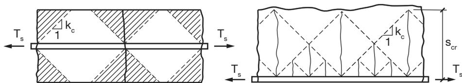
**Fig. 3.3.** Stress lines and crack patterns of tension members with reinforcing bars in the middle (left) and at the bottom (right).
