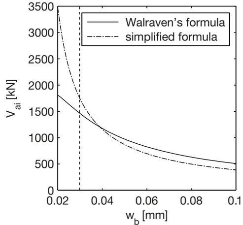
Fig. 4.10. Relationship between  $V_{ai}$  and  $w_b$  derived from Walraven's formula and simplified formula at  $\Delta = 0.02$  mm.
