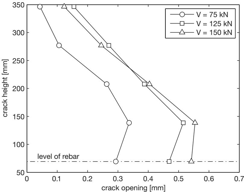
Fig. 4.7. Crack profile measured by photogrammetric measurement (Crack marked in Fig. 4.6)
