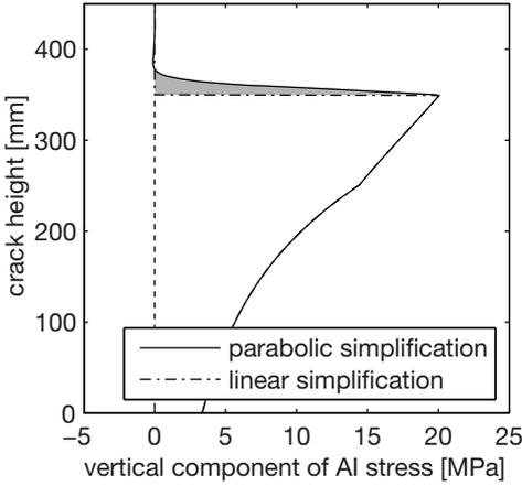
**Fig. 4.3.** Distribution of vertical component of  $V_{ai}$  along the height direction.
