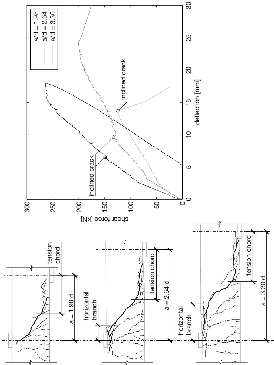
**Fig. 3.40.** Formation of arch structure by inclined cracks in beams with different shear span, and their influence to the load-deflection relationship. The specimens are C2b151 (see also Fig. 3.5 and Fig. 3.34), C3b121 and C4b091 from the continuous beam test series.
