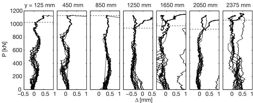
**Fig. 6.22.** Load-vertical displacement relationship at different locations in width direction of test M038B
