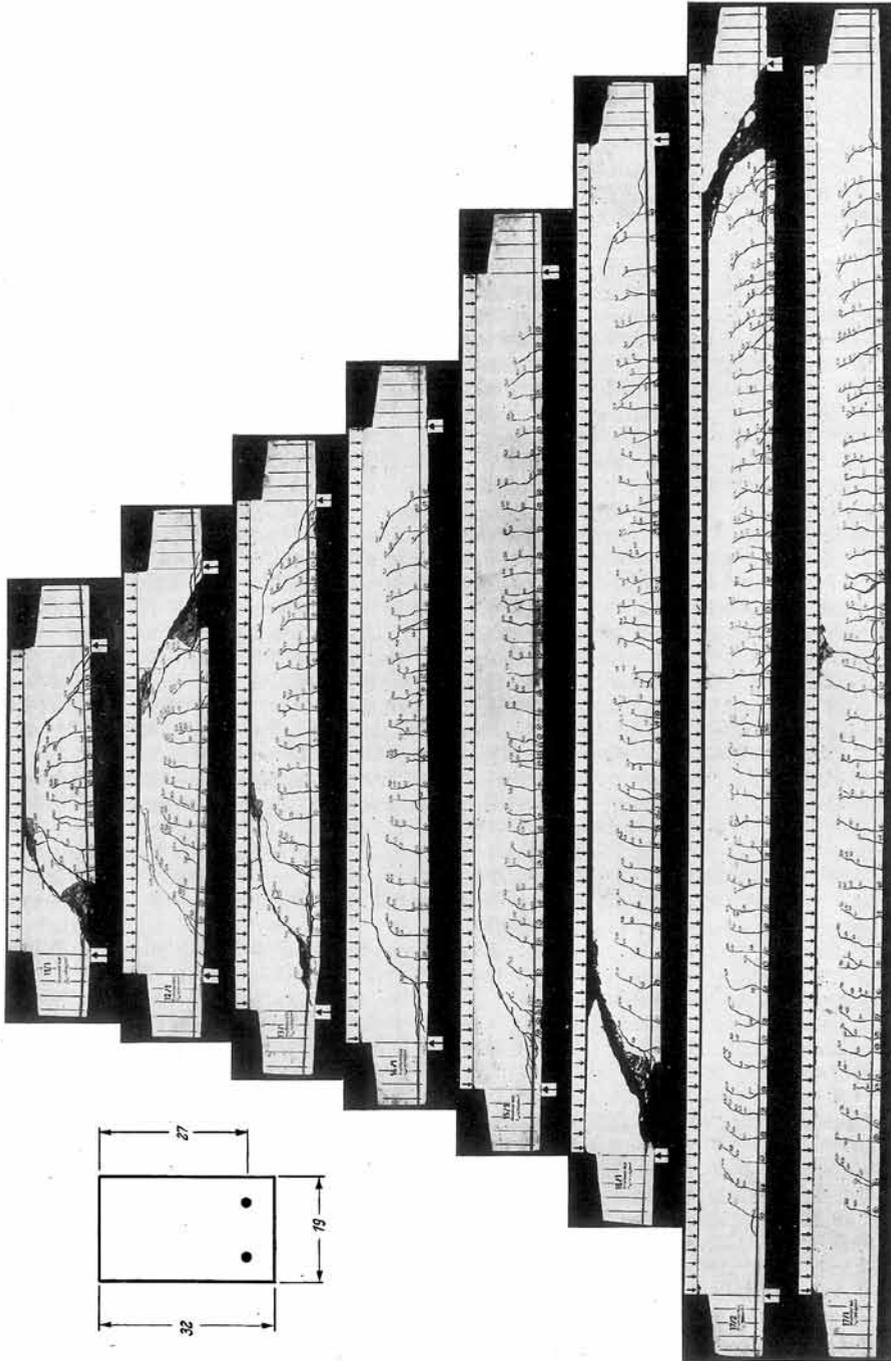
Fig. 5.23. Crack pattern of simply supported beams loaded by uniformly distributed load ((Leonhardt & Walther 1962).
