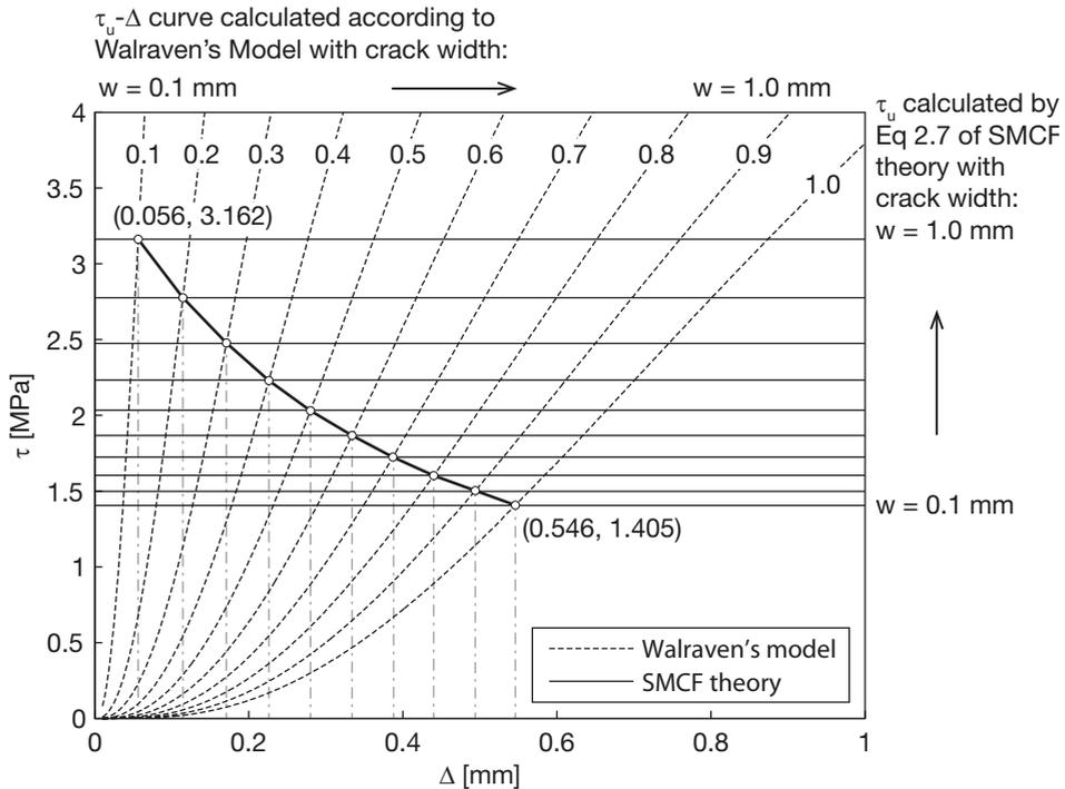
**Fig. 2.7.** Comparison between Simplified Modified Compression Field (SMCF) theory and Walraven's model for the same crack widths and shear stresses.
