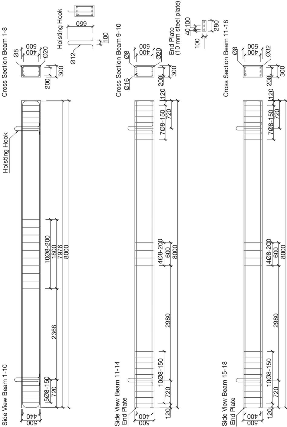
Fig. 5.3. Dimensions and reinforcement configurations of the specimens.
