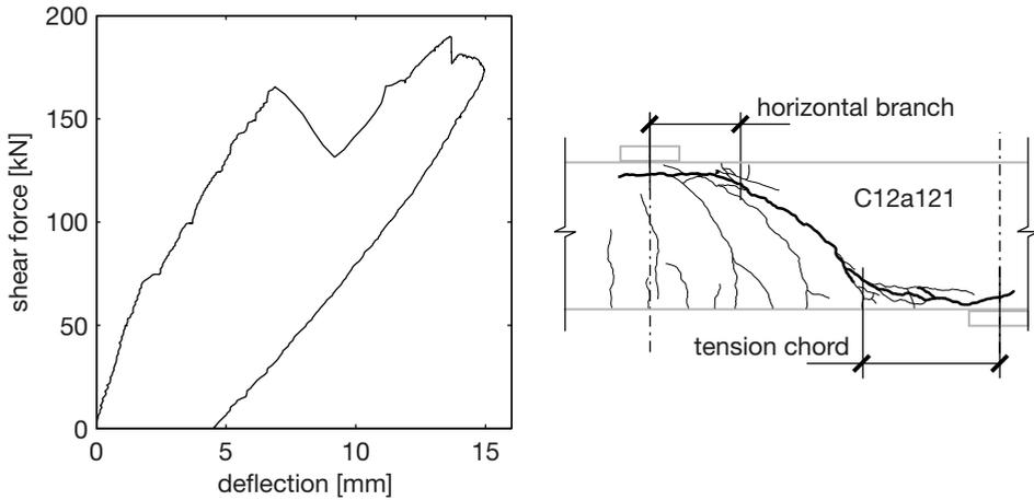
**Fig. 3.43.** Load deflection and crack pattern of specimen C12a121 with  $a/d = 2.64$ . Check Fig. 3.40 for specimen with the same boundary conditions but different failure mode.
