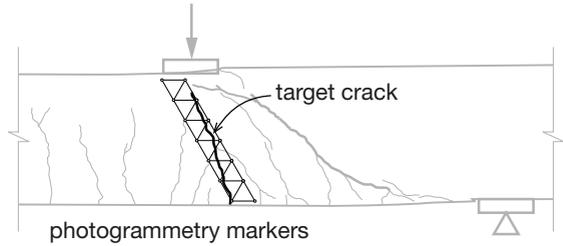
**Fig. 4.6.** Measurement of the crack opening of a major crack (C3b121).
