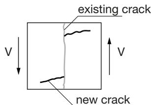
Fig. 6.8. Crack arresting mechanism, adopted from (Pimanmas & Tisavipat 2005).
