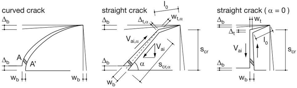
**Fig. 5.21. Kinetic condition of an inclined crack.**
