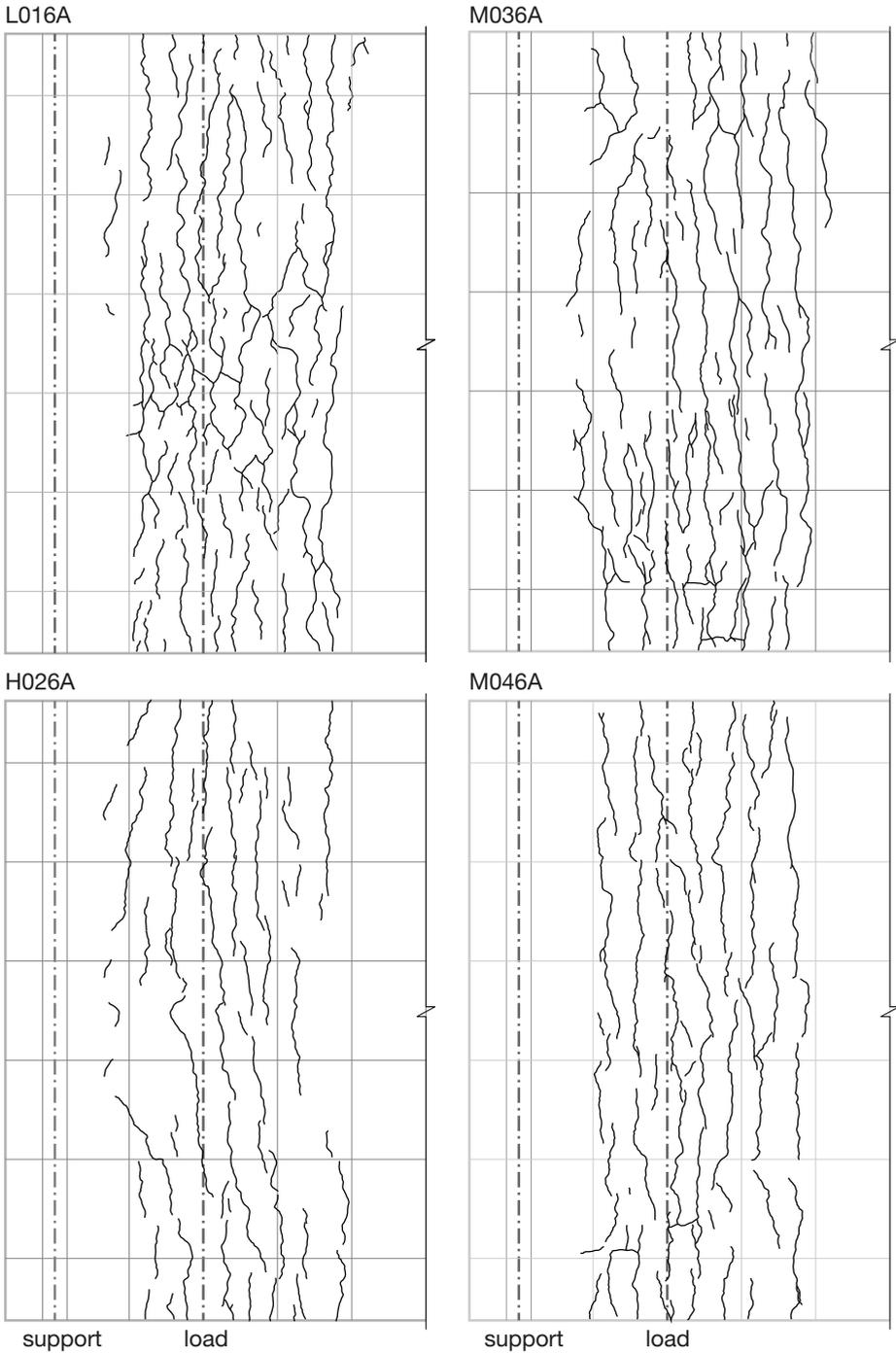
**Fig. 6.24.** Bottom crack patterns of series 1 at  $P = 800$  kN.
