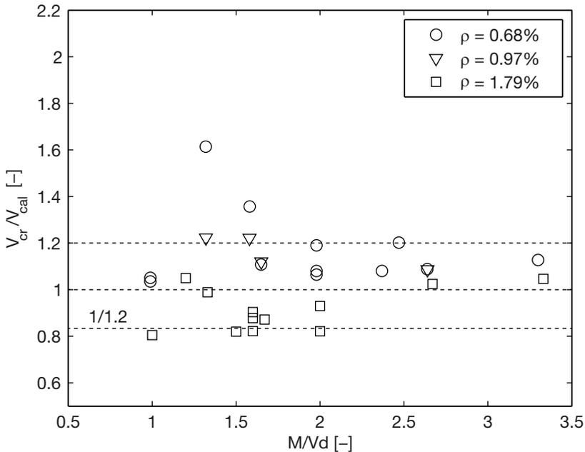
**Fig. 5.16.** Relationship between  $V_{cr}/V_{cal}$  and  $M/Vd$ ,  $V_{cal}$  as calculated with the adjusted critical vertical displacement.
