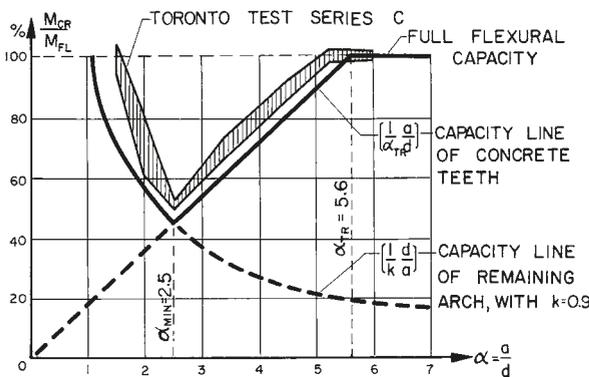
Fig. 2.10. Influence of  $a/d$  on the beam capacity known as Kani's Valley (Kani 1964).
