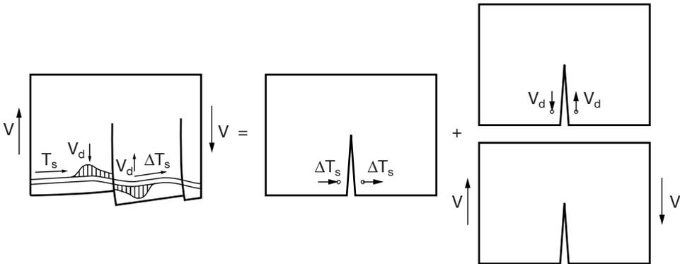
**Fig. 3.11. Forces applied at the concrete part of a RC beam**
