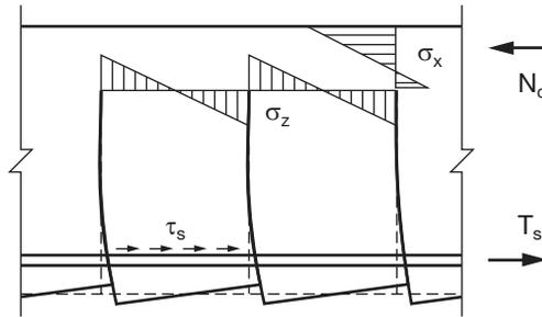
**Fig. 3.8.** Indication of stress distribution in Kani's Teeth model.
