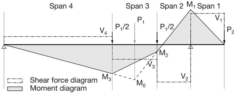
**Fig. 5.10. Moment and shear force diagram of two point loads test.**
