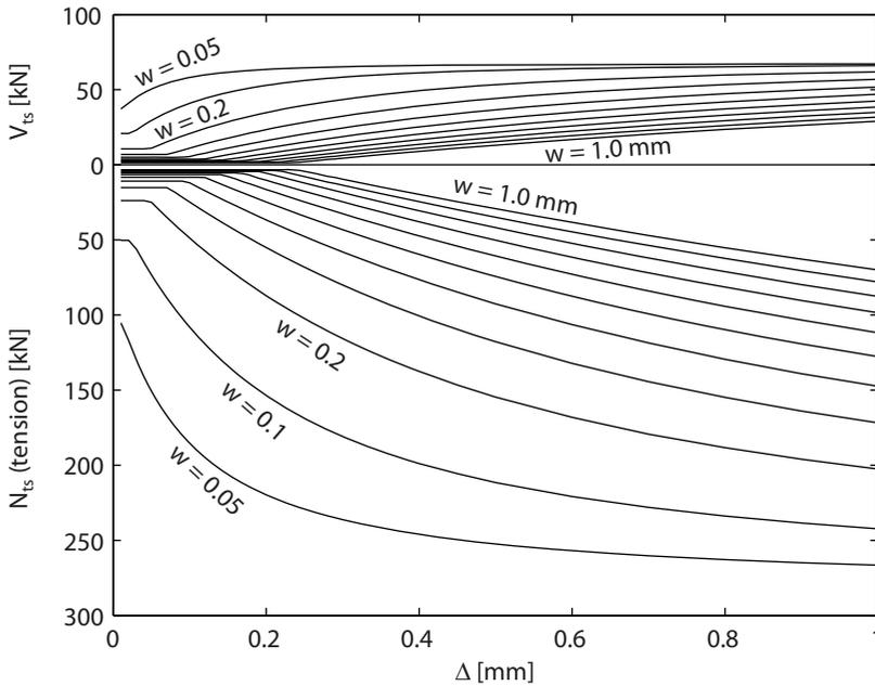
**Fig. 3.30.** Relationship between resultant forces from tension softening effect in  $x, y$  direction and crack bottom displacement ( $w, \Delta$ ).
