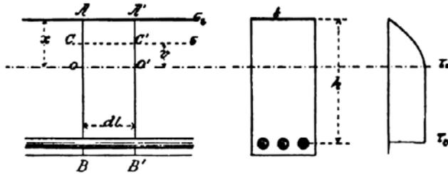
**Fig. 2.4.** Parabolic shear stress distribution assumed by Morsch (Morsch 1909).
