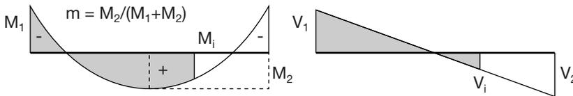
**Fig. 5.29.** Moment and shear force distribution of a beam loaded by uniformly distributed load with generalized boundary conditions.
