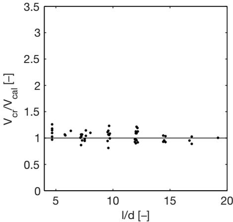
**Fig. 5.27.** Relationship between  $V_{cr}/V_{cal}$  and  $l/d$  with the improved simplified method.
