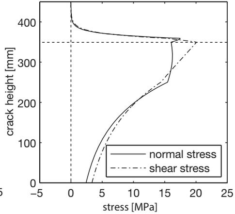
**Fig. 4.4.** Distribution of normal stress and shear stress due to aggregate interlock effect along the crack height (parabolic simplification).
