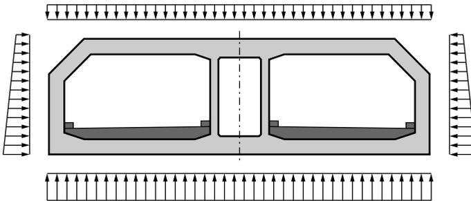
**Fig. 5.1. Loading conditions of typical concrete structures vulnerable to shear failure.**
