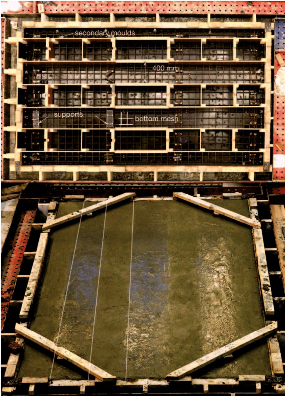
Fig. 6.19. Overview of concrete mould (top), prepared specimen after casting (bottom).
