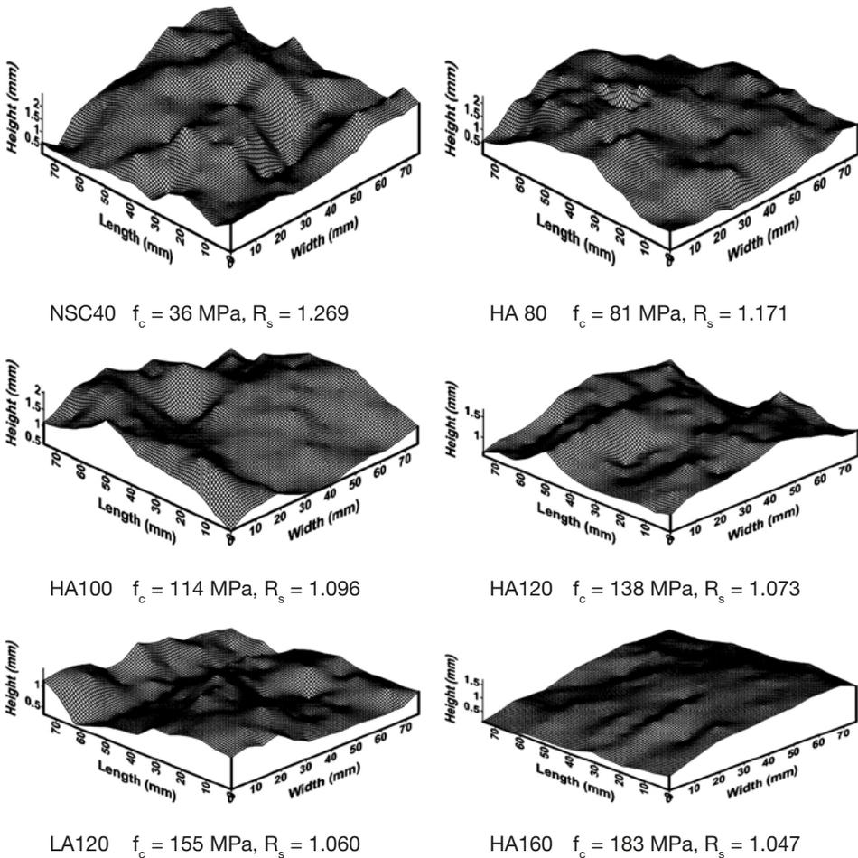
Fig. 4.14. Fractured surfaces of splitting tensile tested specimen; the names of the specimens are according to the original paper (Perera & Mutsuyoshi 2013).
