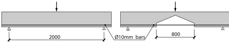
Fig. 3.44. Configurations of Beeby's beams adopted from (Walraven 2007).
