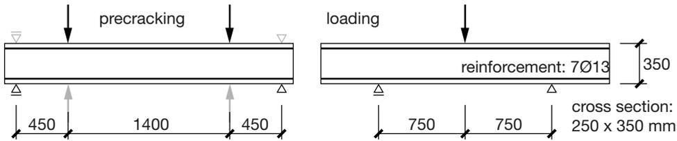
**Fig. 6.3.** Loading arrangement for Pimanmas and Tisavipat's beam tests. Adapted from (Pimanmas & Tisavipat 2005).
