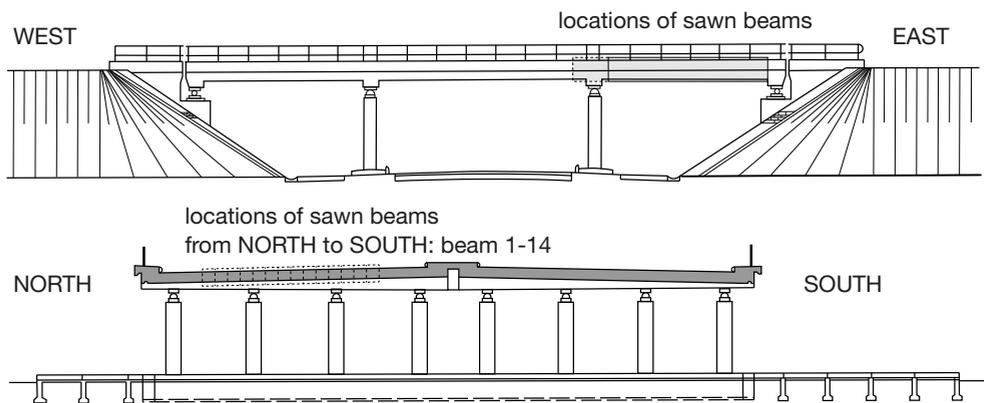
**Fig. 6.9.** Geometries of the deck of Gestelsstraat Bridge and the location of the test specimens in the bridge deck.
