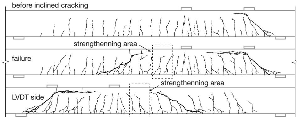
**Fig. 5.13.** Crack pattern of D18a121 after failure.
