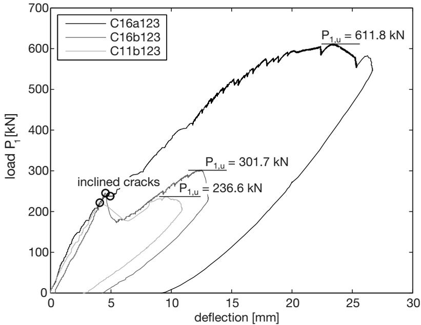
**Fig. 6.7.** Load-deflection relationship of pre-cracking tests series.
