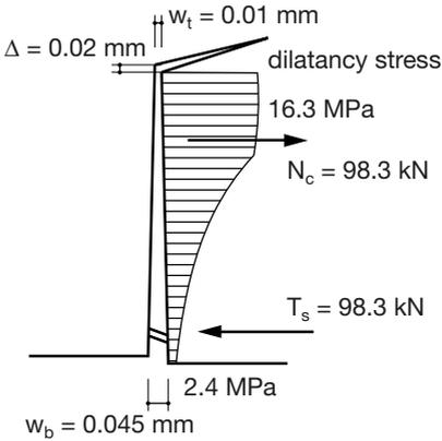
**Fig. 4.5.** Normal stress/force distribution along crack height.
