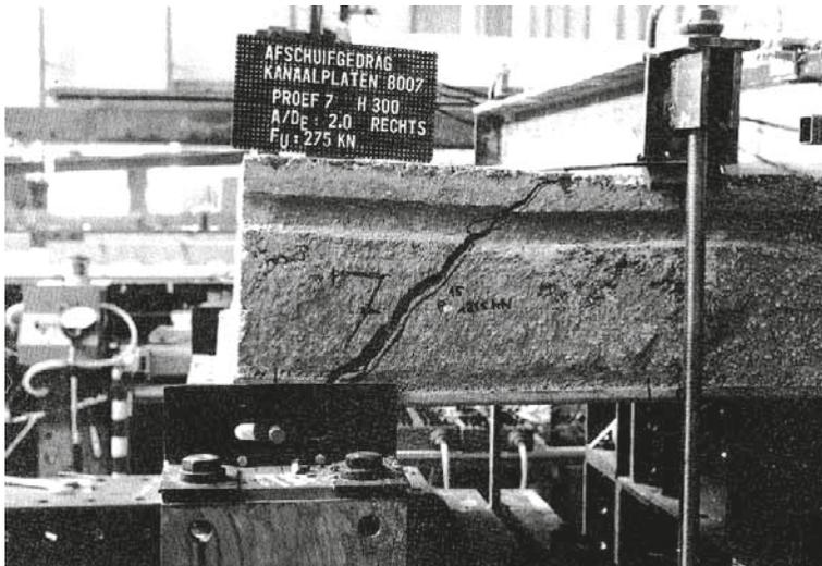
Fig. 2.1. Diagonal tension failure of a hollow core slab (Walraven & Merx 1983).
