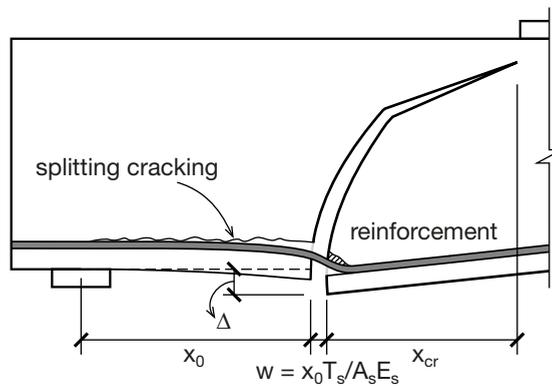
**Fig. 3.35.** Dowel cracking initiated from the root of a major crack under shear.
