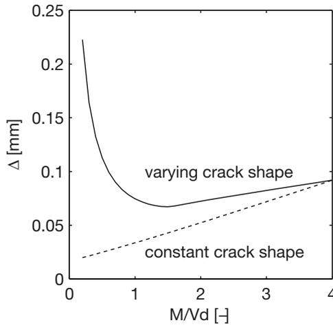
**Fig. 5.20.** Influence of crack shape to the vertical displacement under  $V = 100$  kN.
