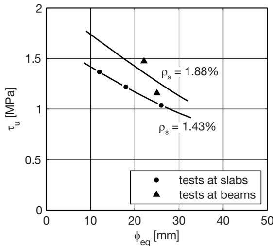
**Fig. 4.19.** Influence of diameter and spacing of bars on shear strength of beams with the same reinforcement ratio, adapted from (Leonhardt 1978).
