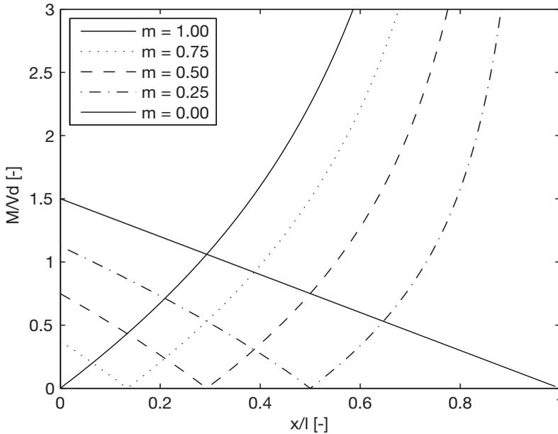
**Fig. 5.30.** Distribution of  $M/Vd$  along the longitudinal axis of the specimens in the TNO tests, see the following section.
