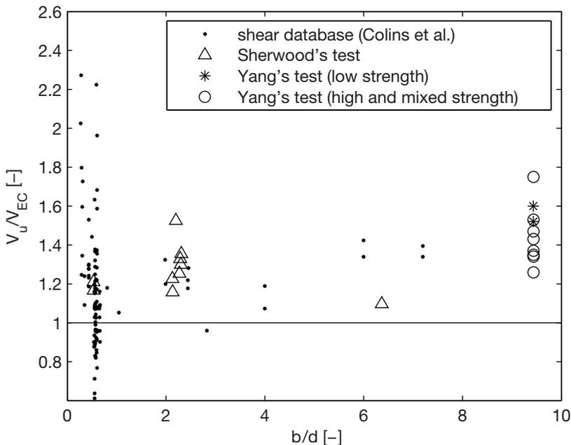
Fig. 6.23. Width depth ratio versus shear capacity prediction with Eurocode.
