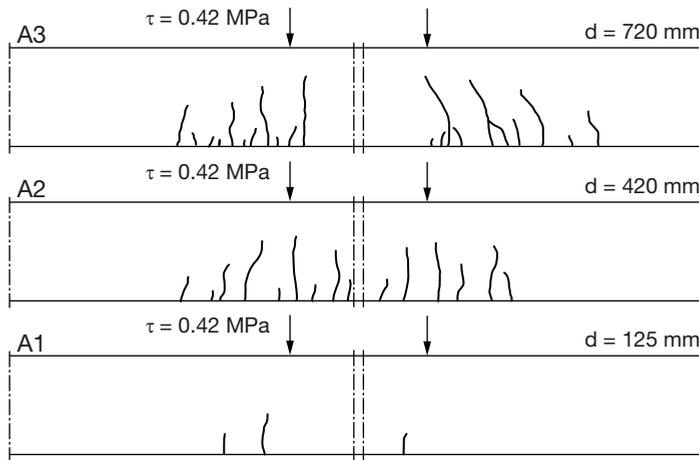
**Fig. 4.25.** Comparison of the scaled crack patterns for beam A1, A2 and A3 at  $\tau = 0.42$  MPa (Walraven 1978)
