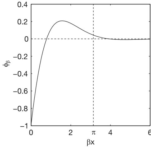
**Fig. 6.27.** Relationship between  $\phi_\beta = e^{-\beta x}(\sin\beta x - \cos\beta x)$  and  $\beta x$ .
