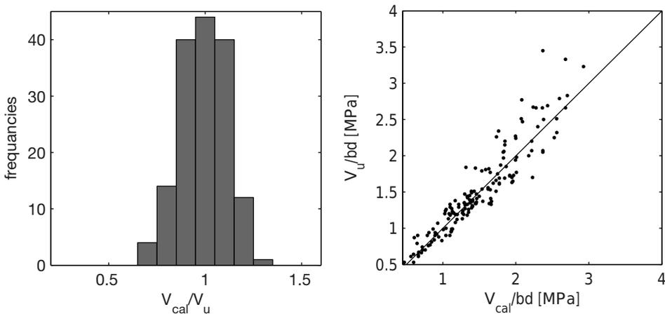
**Fig. 4.24.** Comparison of predicted shear force and test results based on König and Fischer’s database taking into account the rebar configuration.
