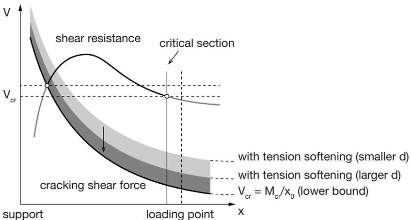
**Fig. 4.31.** Determination of shear resistance taking into account tension softening.
