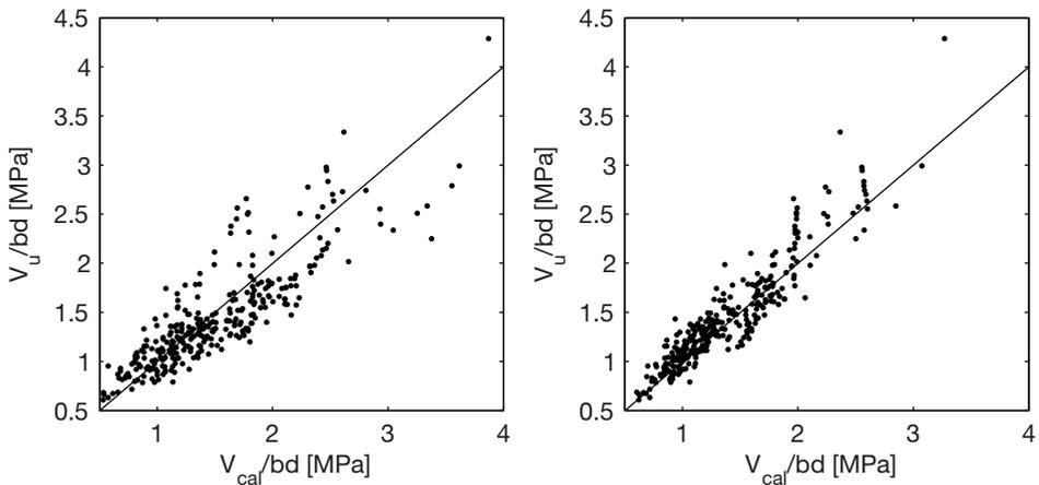
**Fig. 4.23.** Comparison of predicted and tested shear strength with Eq. (4.9) (left) and Eq. (4.15) (right).
