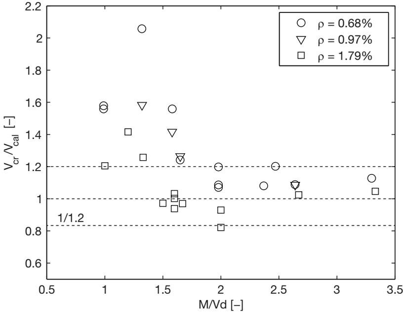
Fig. 5.14. Relationship between  $V_{cr}/V_{cal}$  and  $M/Vd$ ,  $V_{cal}$  calculated by the adjusted critical shear displacement shown in Section 4.6.
