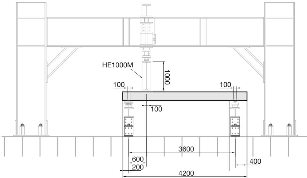
**Fig. 6.20.** Test setup of specimens with concrete strength variability in width direction.
