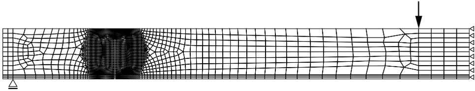
Fig. 3.16. Mesh configuration and boundary conditions of model with  $x_0 = 700$  mm.
