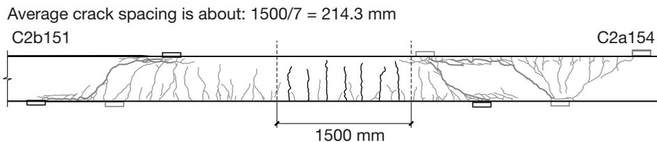
**Fig. 3.5.** Crack pattern after failure of test C2a154 and C2b151 in (Yang & den Uijl 2011).
