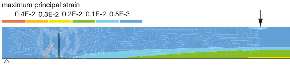
**Fig. 3.19.** Distribution of maximum principal strain of model with  $x_0 = 600$  mm.
