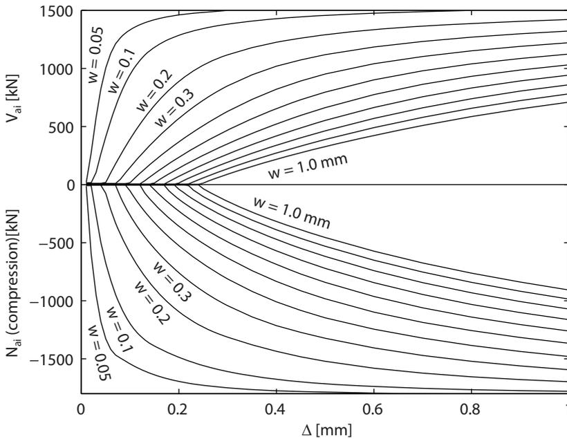
**Fig. 3.29.** Relationship between resultant forces in  $x, y$  direction and crack bottom displacements  $(w, \Delta)$  of a concrete beam.
