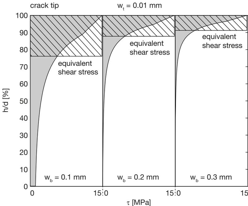
**Fig. 4.29.** Shear stress distribution calculated from different crack width at the tensile side ( $w_b = 0.1$  mm, 0.2 mm and 0.3 mm respectively,  $\Delta = 0.02$  mm,  $f_{cm} = 40$  MPa).
