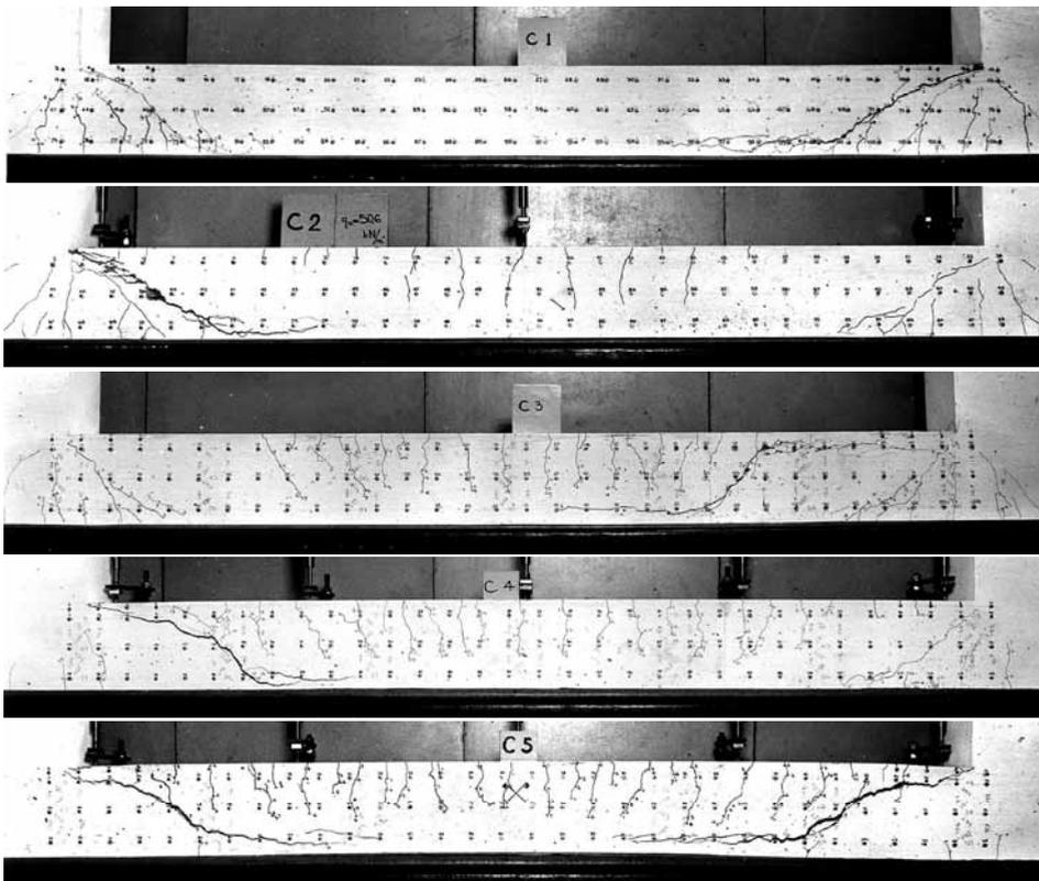
**Fig. 5.36.** Crack pattern of test series C after failure.  $l = 1350$  mm, from C1 to C5,  $m = 0.00, 0.25, 0.50, 0.75$  and  $1.00$  respectively (IBBC-TNO 1985).
