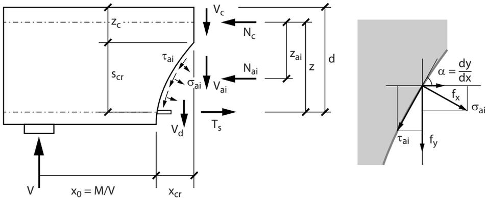
Fig. 3.25. Part of a reinforced concrete member (free body) cut along a crack ( $x_0 = d$ )
