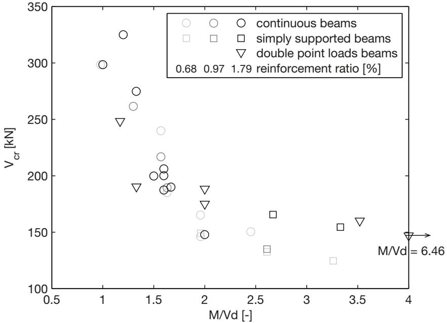
Fig. 5.12. Relationship between inclined cracking load  $V_{cr}$  and  $M/Vd$ .
