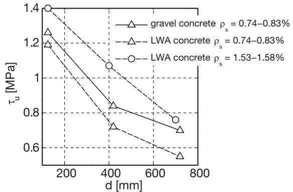
**Fig. 4.27.** Results of Walraven's size effect test on gravel and light-weight aggregate concrete, adopted from (Walraven 1978).
