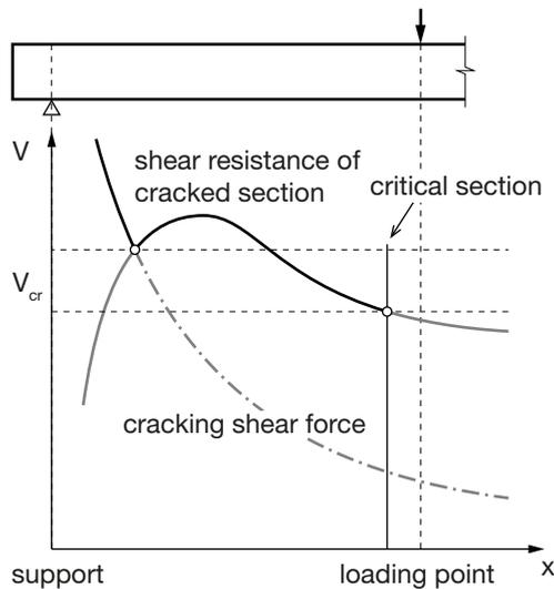
**Fig. 3.38.** Illustration of shear resistance versus cracking shear force line at shear failure.
