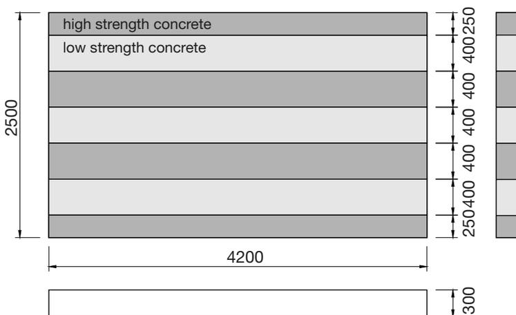
Fig. 6.18. Dimensions and layout of test specimens with mixed strengths.
