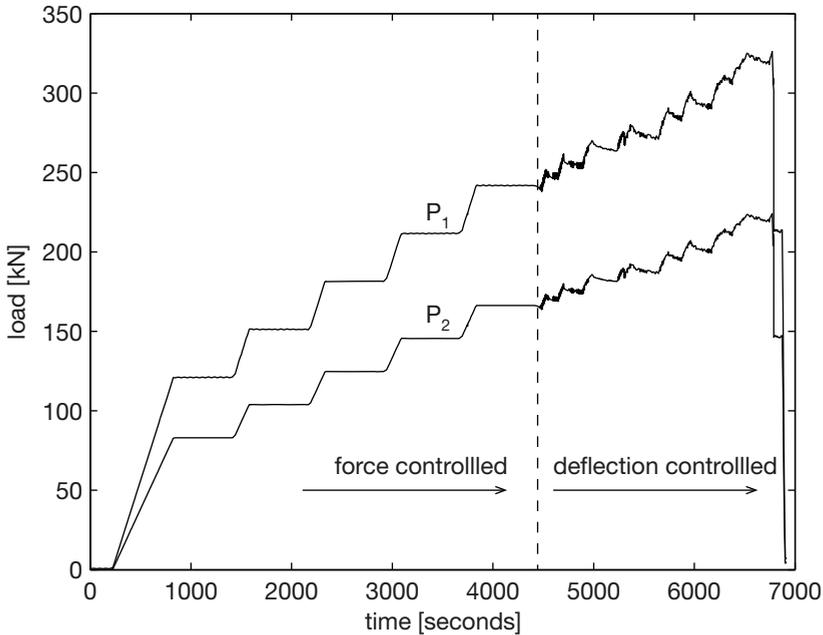
**Fig. 5.6.** Loading procedure of specimen C2a152.
