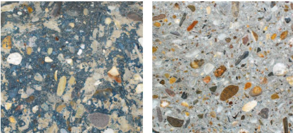
**Fig. 6.17.** Surface of inclined crack in Beam 4E (left) and Beam 1N (right).
