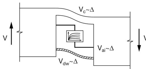
**Fig. 3.45.** Shear resisting components in an inclined cracked region of a reinforced concrete beam.
