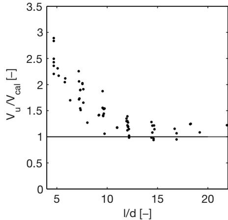
**Fig. 5.28.** Relationship between  $V_u/V_{cal}$  and  $l/d$  with the improved simplified method.
