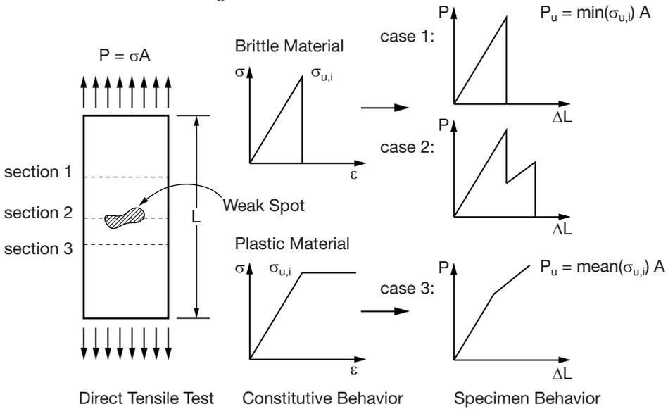
**Fig. 6.1.** Relation of material constitutive behaviour to the behaviour of tensile element with weak spot.
