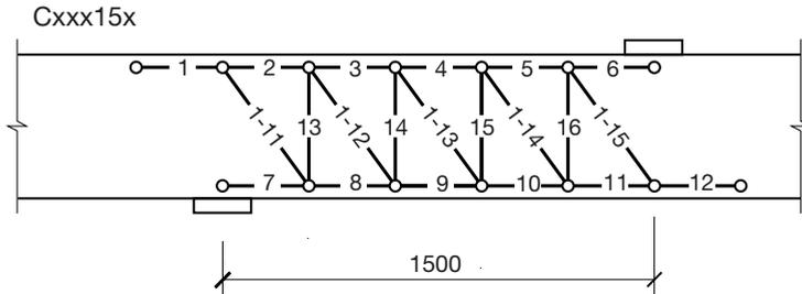
**Fig. 5.7.** Configurations of LVDT array for beams with shear span  $a = 1500$  mm.
