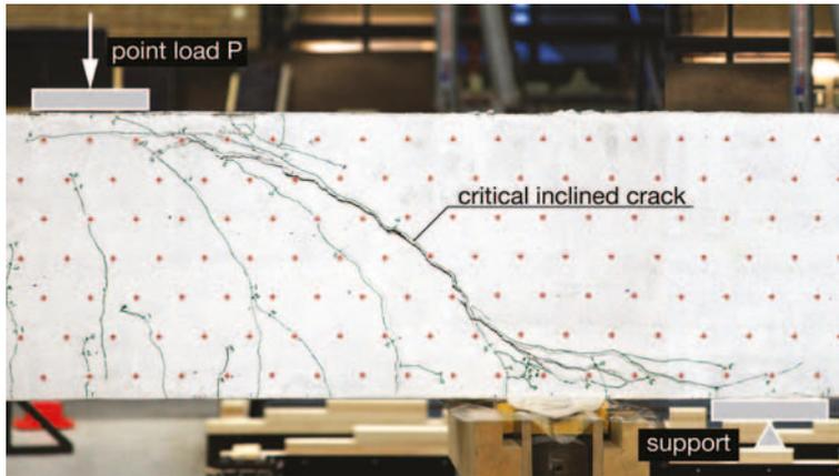
**Fig. 2.2.** Crack pattern of beam with flexural shear failure (diagonal tension failure according to some literature).
