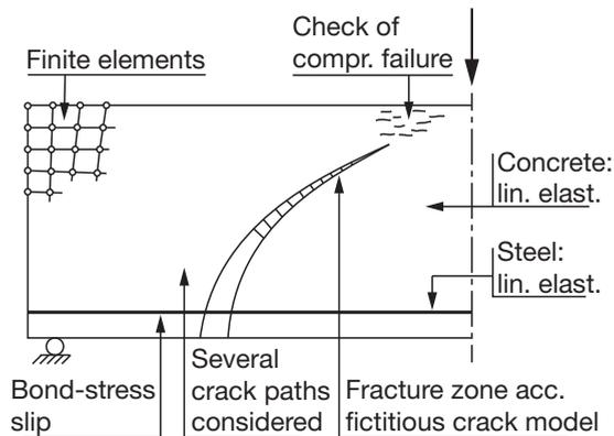
Fig. 2.9. Fictitious crack model for shear cracking simulation (Gustafsson & Hillerborg 1988).
