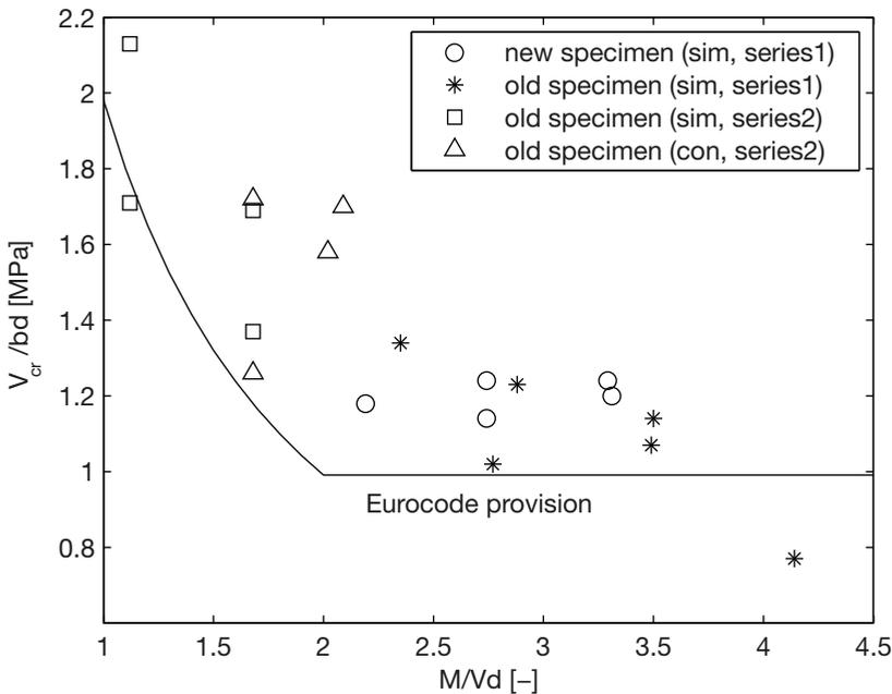
**Fig. 6.15.** Comparison of  $V_{cr}/bd$  derived from specimens made of old concrete and new concrete. In the legend, sim stands for simply supported specimens, con stands for continuous supported specimens
