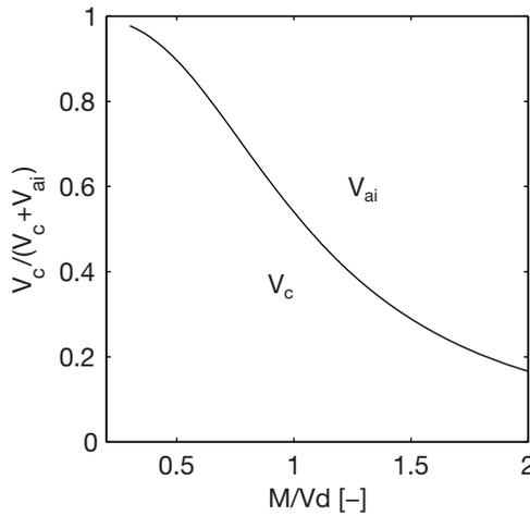
**Fig. 5.15.** Variation of proportion between  $V_c$  and  $V_{ai}$  with respect to  $M/Vd$ .
