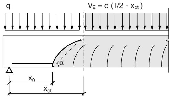
**Fig. 5.18.** Evaluating shear force  $V_E$  for a critical shear crack.
