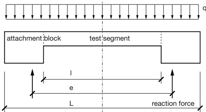
**Fig. 5.32.** Configuration of TNO test specimens. Adapted from (IBBC-TNO 1985).
