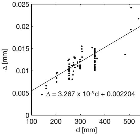
**Fig. 4.20.** Relationship between beam height  $d$  and critical shear displacement  $\Delta_{cr}$  for beams reinforced by  $\text{Ø}25$  bars.
