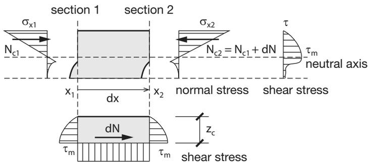
Fig. 3.27. Stress distribution in concrete compressive zone. Adopted from (Reineck 1991).
