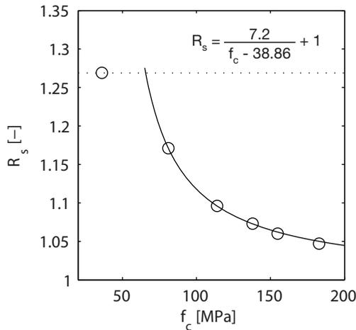
**Fig. 4.13.** Influence of concrete strength to fractured surface roughness, adapted from (Perera & Mutsuyoshi 2013).
