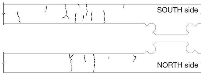
**Fig. 6.11.** Existing cracks in Beam 6.
