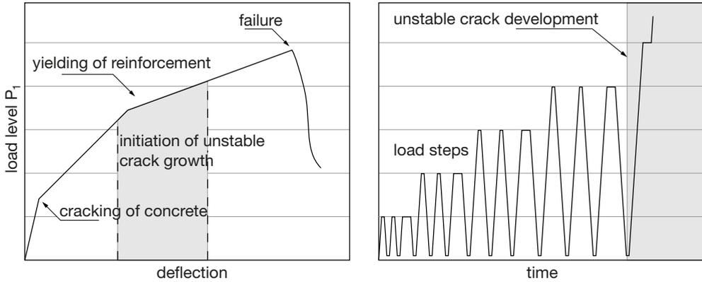
**Fig. 6.14.** Illustration of loading scheme of  $P_1$ .
