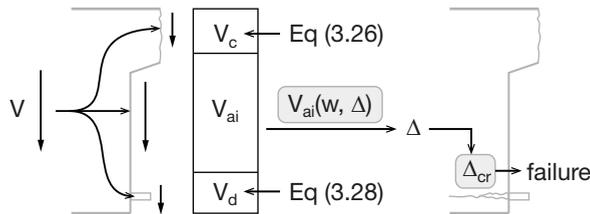
**Fig. 4.1.** Scheme of inclined crack evaluation, where the items in the boxes have to be evaluated.
