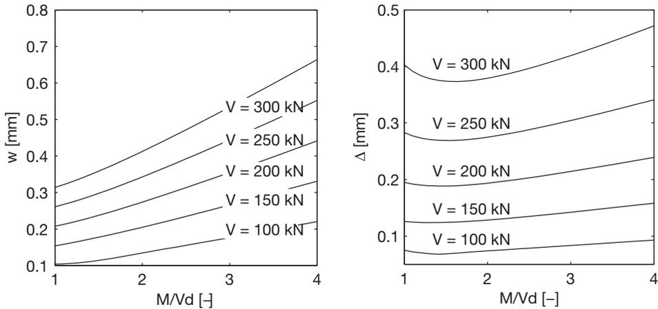
**Fig. 3.33.** Crack opening combination of cracks generated at  $M/Vd$  from 1.0 to 4.0 under different shear forces (left: crack opening  $w$  in longitudinal direction; right: crack opening  $\Delta$  in vertical direction).
