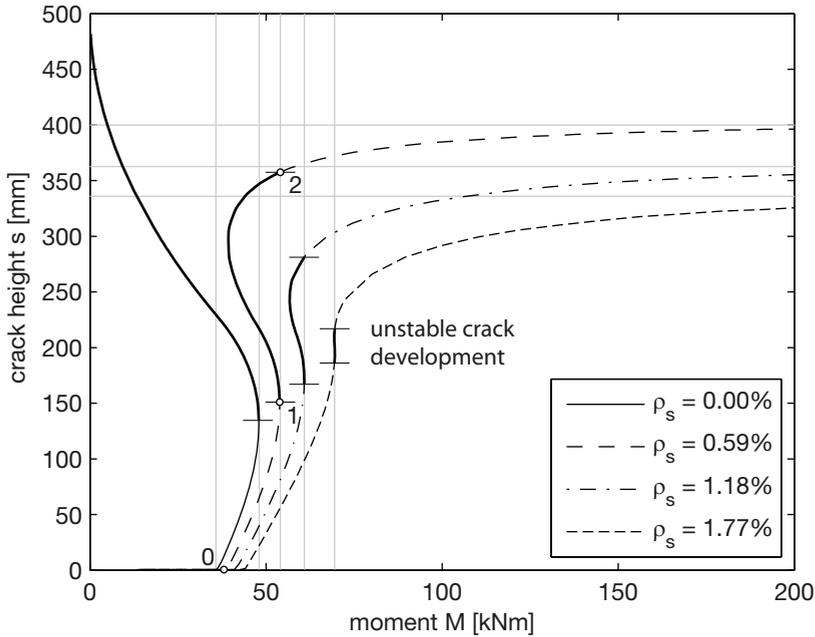
**Fig. 3.2.** Crack height  $s$  versus cross-sectional moment  $M$  relationship for beams with different reinforcement ratios.
