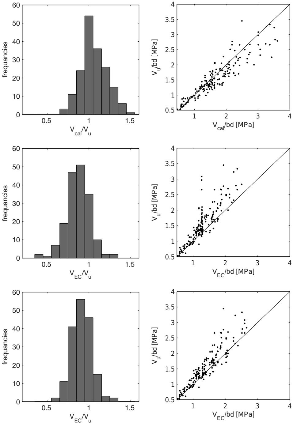
**Fig. 4.12.** Comparison of predicted shear capacities and test results based on König and Fischer's shear database. From top to bottom: results of own  $\Delta_{cr}$  model, Eurocode and Eurocode without limitation on  $k \leq 2.0$ .
