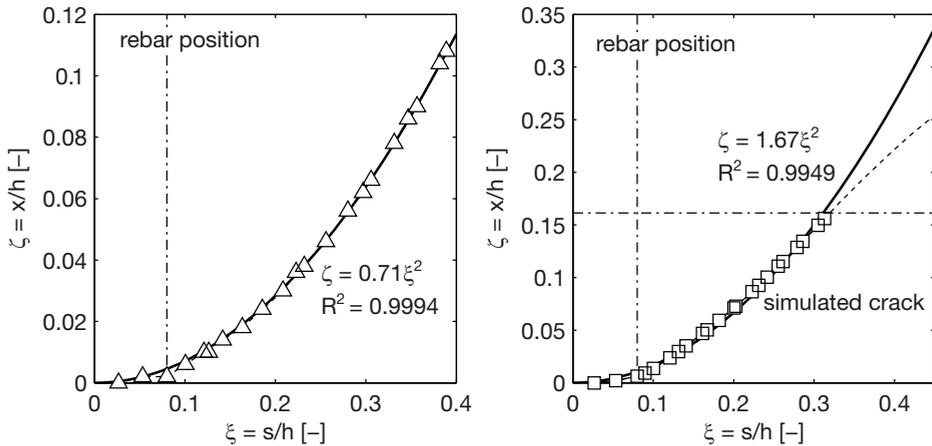
**Fig. 3.22.** Regression analysis of two crack paths. Left:  $x_0 = 1400$  mm. Right:  $x_0 = 200$  mm.
