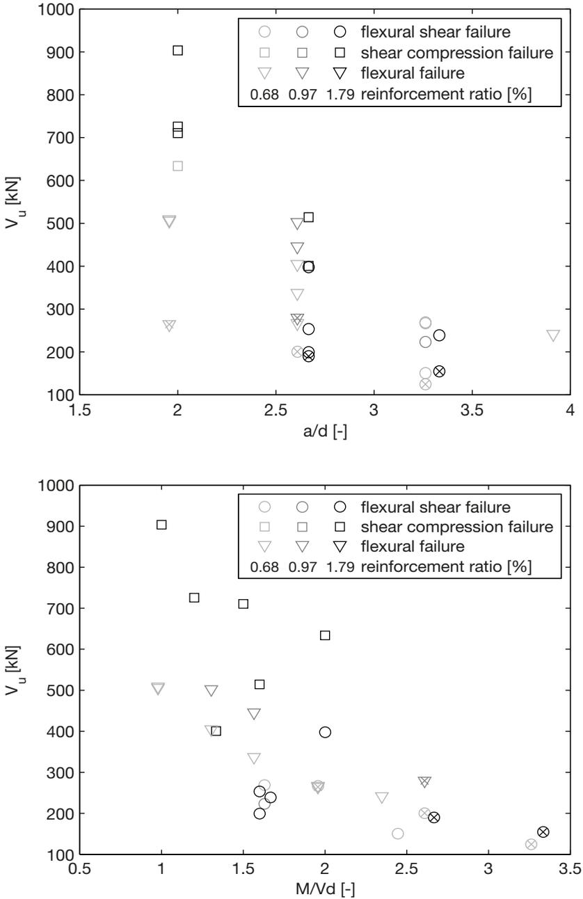
**Fig. 5.11.** Relationship of maximum shear capacity  $V_u$  plotted against  $a/d$  (upper) and  $M/Vd$  (lower): the additional cross on the markers stands for simply supported beams. The extra sign  $\times$  on the data point indicates that it is a simply supported test.
