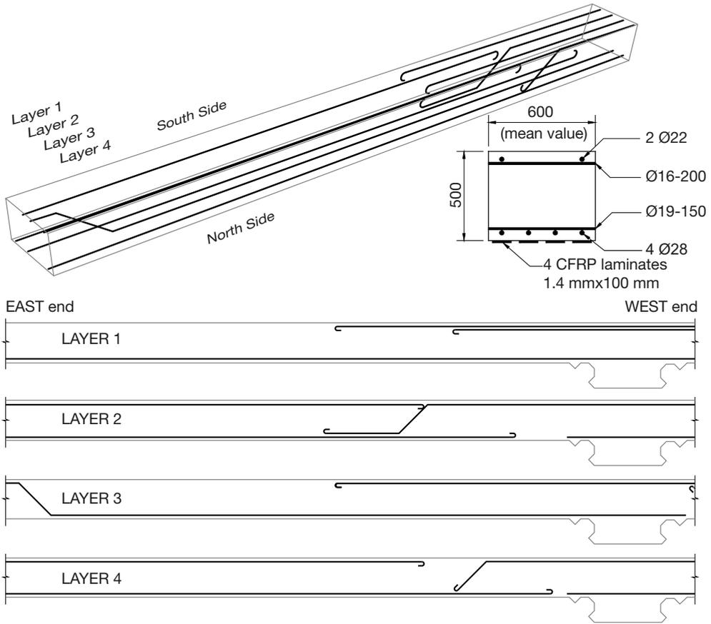
**Fig. 6.10.** Reinforcement layout of the old beams sawn from the Gestelsstraat bridge.
