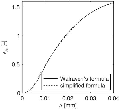
Fig. 4.9. Relationship between  $v_{ai}$  and  $\Delta$  derived from Walraven's formula and the simplified relationship.
