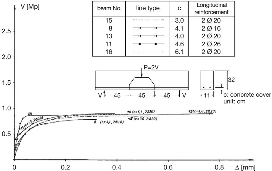
Fig. 3.28. Shear displacement – dowel force relationship of tests carried out by Baumann and Rüsç, adapted from (Baumann & Rüsç 1970).
