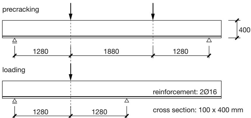
Fig. 6.2. Loading arrangement for Hamadi and Regan's beam tests with existing flexural cracks (Hamadi & Regan 1980).
