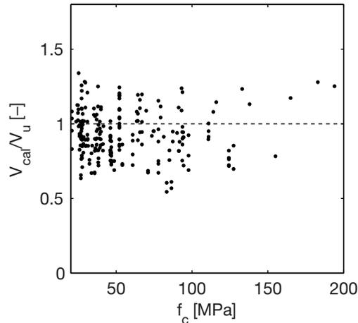
**Fig. 4.17.** Influence of concrete strength to the shear capacity prediction after limiting the concrete strength when  $f_c > 45$  MPa.
