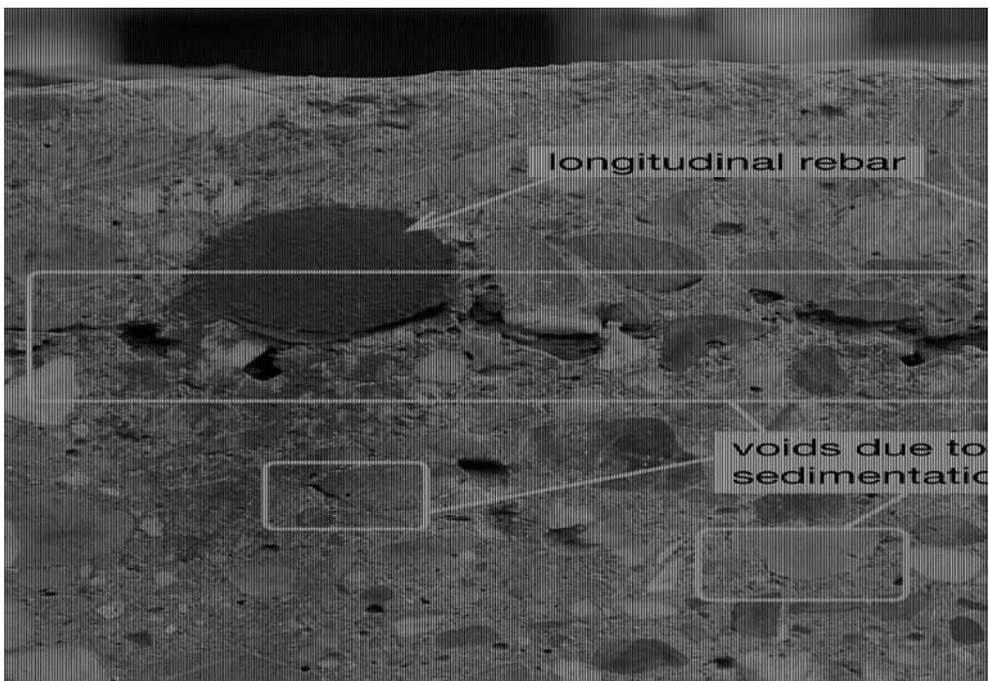
**Fig. 6.12.** Voids observed in a section of concrete beam specimen.
