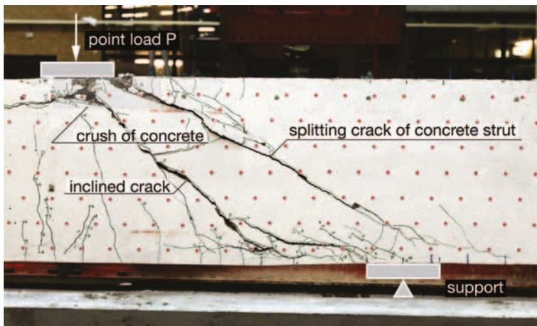
**Fig. 2.3.** Crack pattern of beam with shear compression failure.
