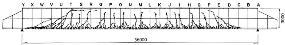
**Fig. 3.6.** Crack patterns of tests specimens with various effective depths (Shioya 1989), the effective heights of the specimens from the top are 100 mm, 1000 mm and 3000 mm respectively.
