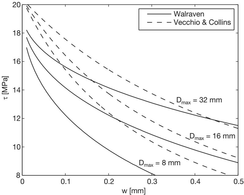
**Fig. 2.6. Comparison between Walraven's model (upper bound) and Vecchio and Collins' model.**
