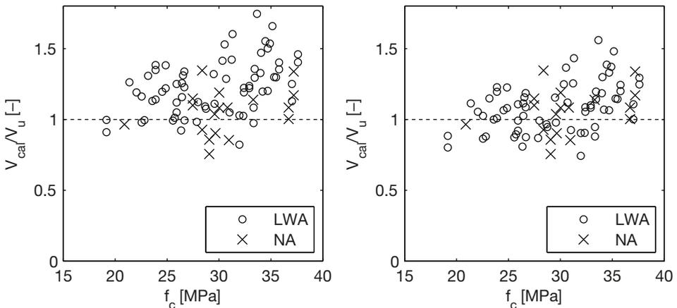
**Fig. 4.18.** Comparison of shear capacity prediction and experimental results. (left: before contact area correction, right: contact area corrected by a factor 0.75, LWA: lightweight aggregate concrete specimens, NA: normal aggregate specimens).
