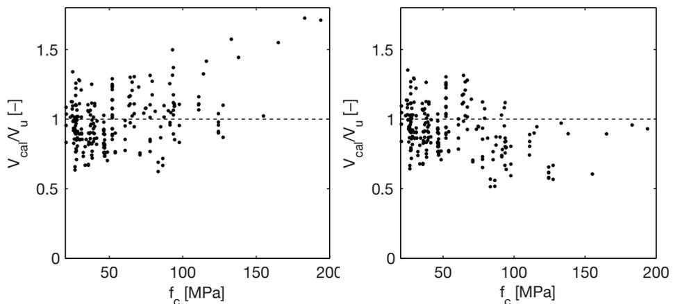
**Fig. 4.16.** Influence of concrete strength to the shear capacity prediction. (left: without aggregate fracture correction, right: with aggregate fracture correction).
