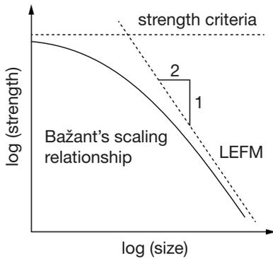
**Fig. 4.26.** Illustration of Bažant's transitional scaling effect relationship (Bažant 2005).
