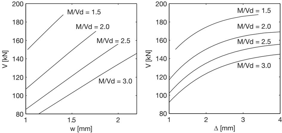
**Fig. 3.36.** Shear force crack bottom displacement relationship according to Eq. (3.34) (left: crack opening  $w$  in longitudinal direction; right: crack opening  $\Delta$  in vertical direction).
