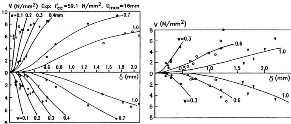
Fig. 4.15. Relationship between shear stress, normal stress, shear displacement and normal displacement of a crack in a plain concrete specimen (left:  $f_c = 59.1$  MPa, right:  $f_c = 110$  MPa), adopted from (Walraven & Stroband 1999).
