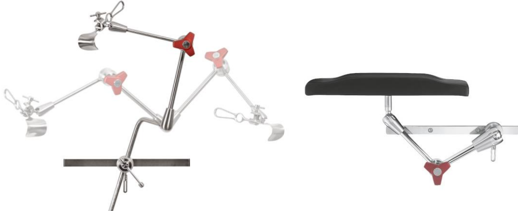
Figure 3.4.3: Fisso articulated arms. 29 A: shown in three different positions. The red one knob handle simultaneously clamps or releases all three joints. All segments can rotate in multiple directions. B: example of arm support application.
