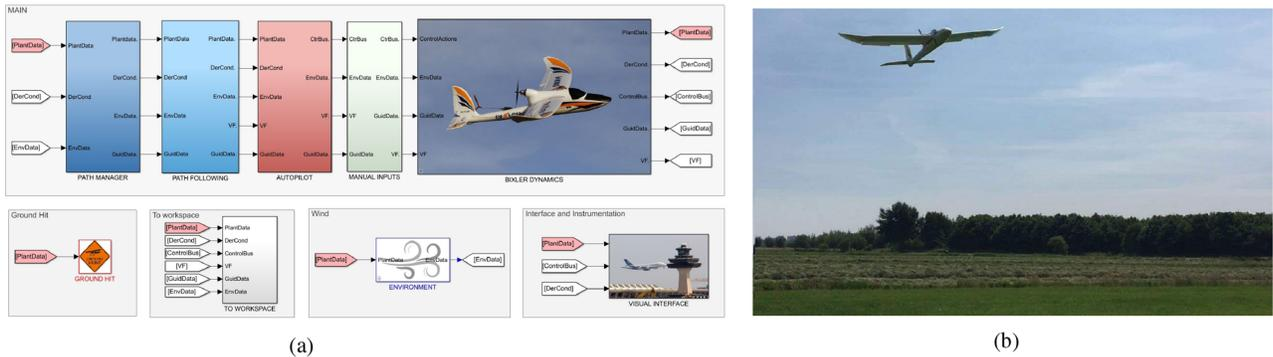
Fig. 5. UAV simulator and actual Bixler during field experiments. (a) UAV simulator (in Matlab-Simulink environment). (b) Actual Bixler during tests.
