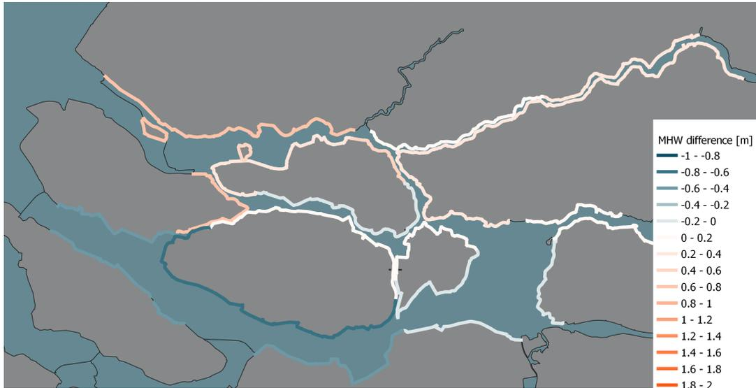
(b) Delta21, failure probability of Europoort barrier of 1/100 per closure and 1 m sea level rise.
