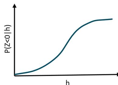
Figure 3.9: Illustration of a fragility curve. The conditional failure probability is depicted on the vertical axis, and the water level on the horizontal axis
