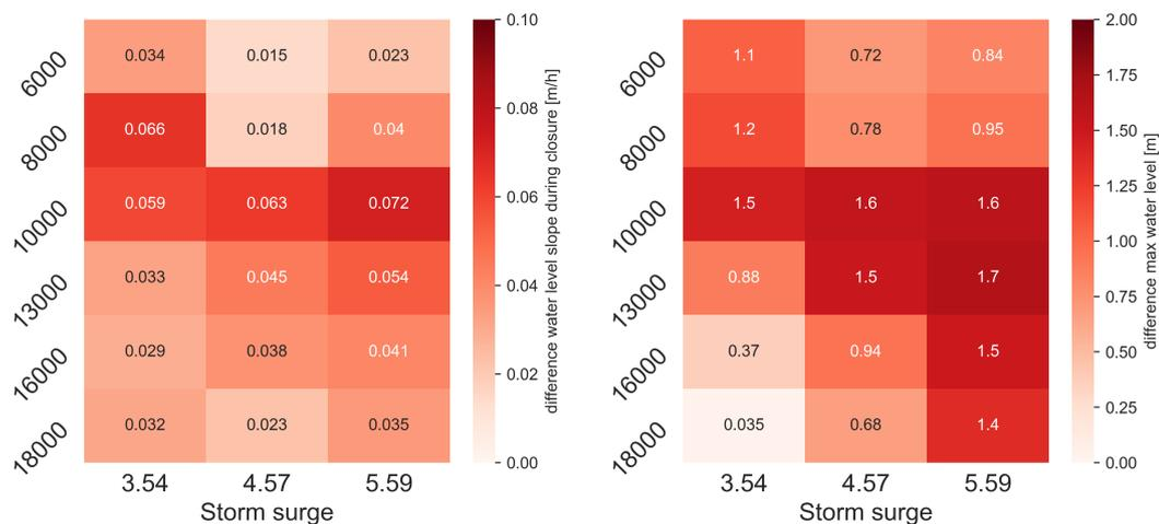
(e) Difference in water level gradient between current system and Delta21.
