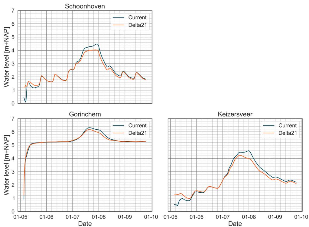
Figure 4.12: Water levels for both configurations during a storm with a Rhine discharge ( $Q_{\text{Lobith}}$ ) of  $10\,000\text{ m}^3/\text{s}$  and storm surge ( $L$ ) of  $3.54\text{ m}$ . Locations are in the discharge dominant area.
