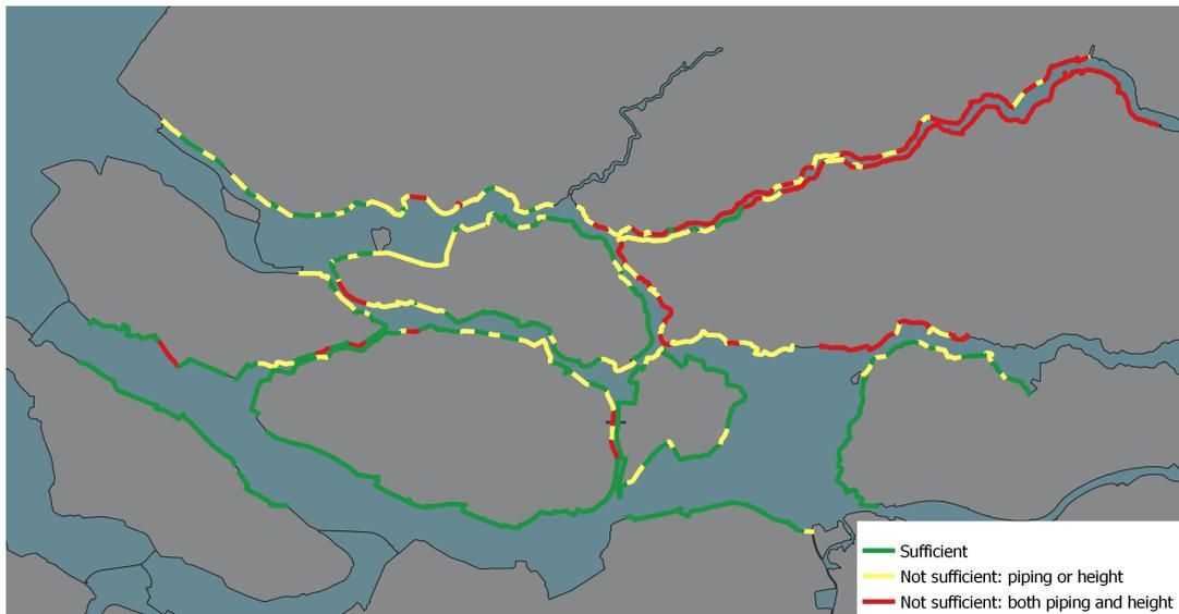
(a) Delta21, failure probability of Europoort barrier of 1/100 per closure and 0 meter sea level rise.
