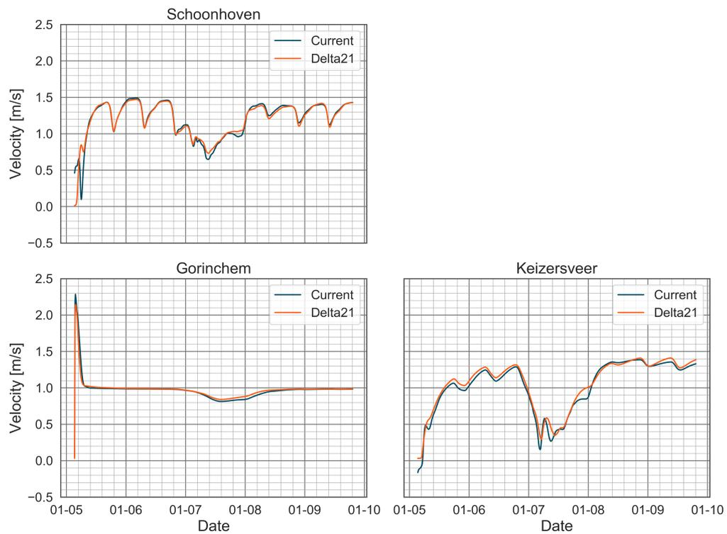
Figure 4.14: Velocities for both configurations during a storm with a Rhine discharge ( $Q_{\text{Lobith}}$ ) of  $10\,000\text{ m}^3/\text{s}$  and storm surge ( $L$ ) of  $3.54\text{ m}$ . Locations are in the discharge dominant area.
