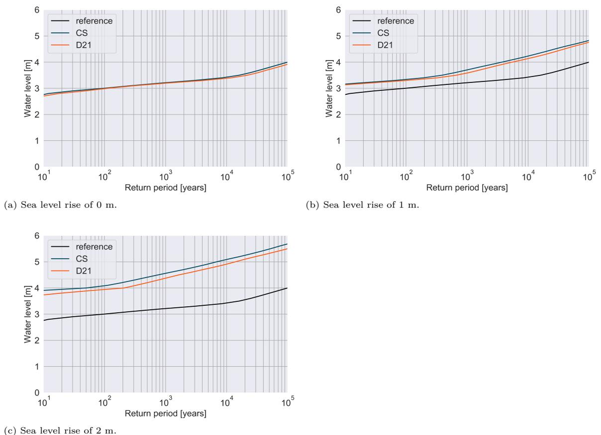
Figure 5.4: Water level frequency lines at Rotterdam for different sea level rise. The current system is indicated with the blue line, Delta21 with the orange line.
