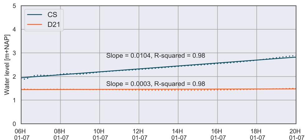
(b) Water level at Rotterdam during the closure of the Europoort barrier. The red square of the upper plot corresponds with the boundaries of this plot. A linear regression line is fitted through the observation points of the simulation, including the slope [m/h] and R-squared.
