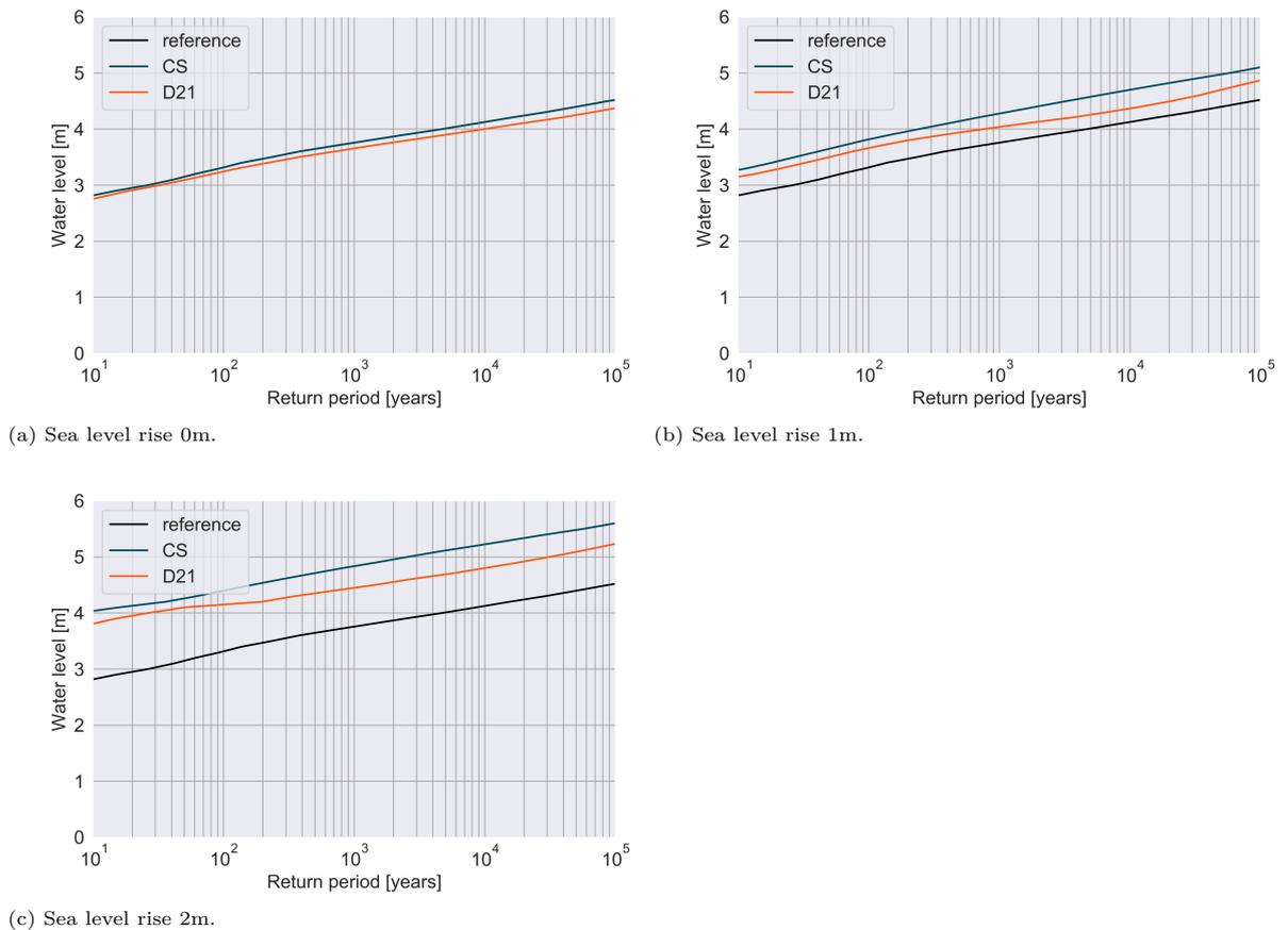
Figure 5.8: Water level frequency lines at Schoonhoven for different sea level rise. The current system is indicated with the blue line, Delta21 with the orange line.
