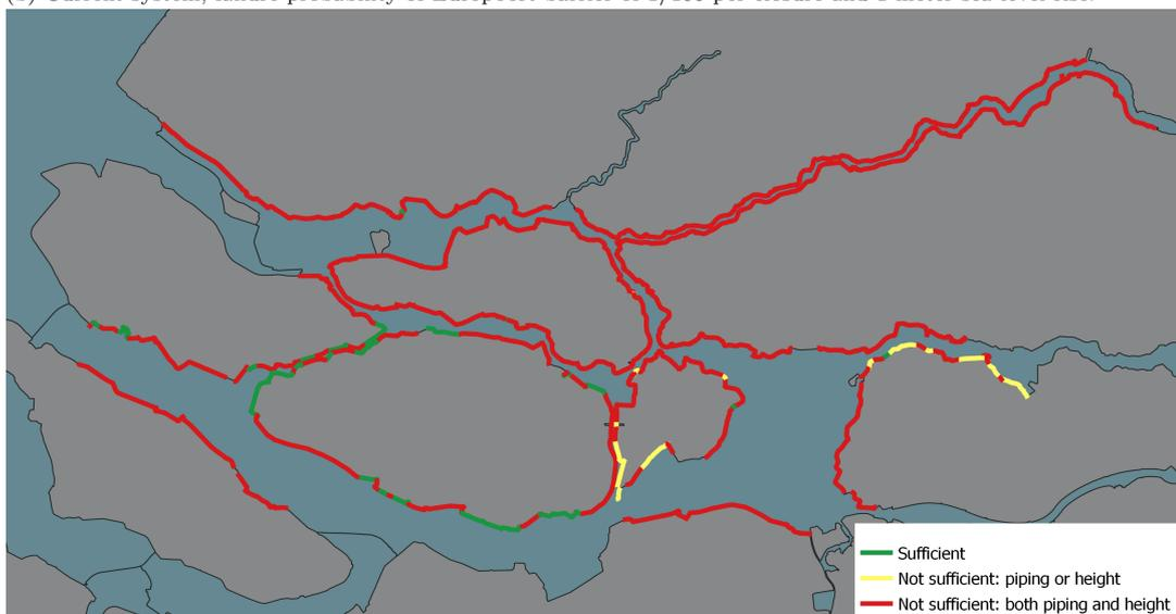
(c) Current system, failure probability of Europoort barrier of 1/100 per closure and 2 meter sea level rise.
