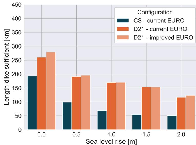
Figure 6.11: Kilometers dike that meet the norm for three different configurations. For different steps of sea level rise, the length of dikes that meet the norms for piping or height are depicted. The current system is depicted in blue and Delta21 is rendered in orange. For Delta21, a distinction is made between the current failure probability (1/100 per closure) and an improved failure probability (1/1000 per closure) of the Europoort barrier. The total length of dikes in the domain is 484 km.
