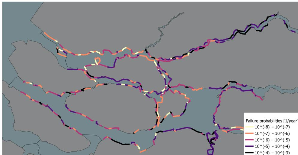
Figure 6.2: Failure probabilities for dike sections in the Rhine-Meuse estuary. Light coloured lines indicate a low failure probability, dark lines correspond to a higher failure probability. This map only provides information about the failure probability, not whether this probability meets the norm. Note that the interval of the classes is logarithmic (Based on data of Vergouwe (2015)).
