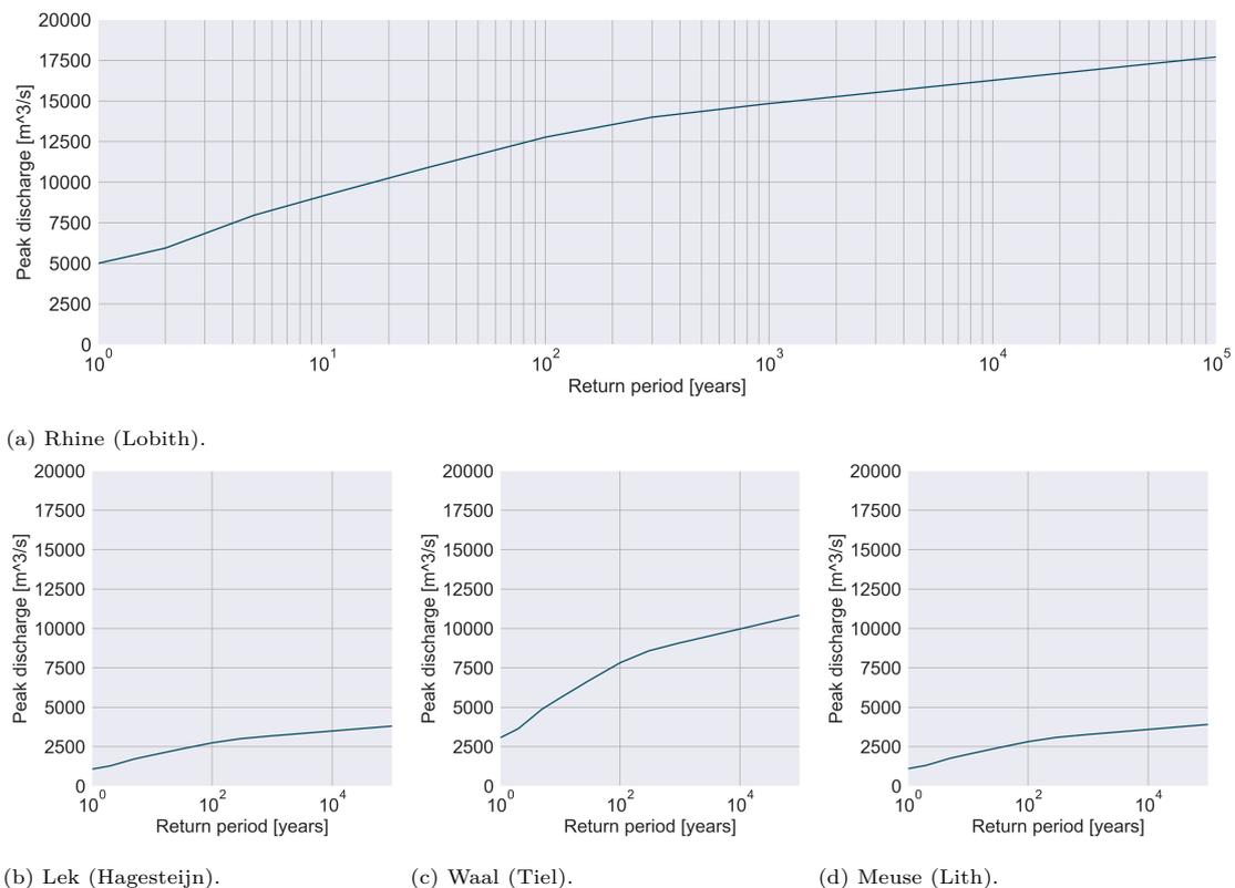
Figure 3.2: Frequency discharge curves for the Rhine branches and the Meuse. In the top graph the frequency discharge curve of the Rhine at Lobith is presented. In this research, the discharge at the Lek, Waal en Meuse river were coupled directly and is confirm WBI-2017 (Hegnauer et al., 2015; Agtersloot and Paarlberg, 2016).
