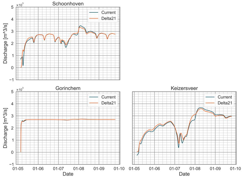
Figure 4.13: Discharges for both configurations during a storm with a Rhine discharge ( $Q_{\text{Lobith}}$ ) of  $10\,000\text{ m}^3/\text{s}$  and storm surge ( $L$ ) of  $3.54\text{ m}$ . Locations are in the discharge dominant area.
