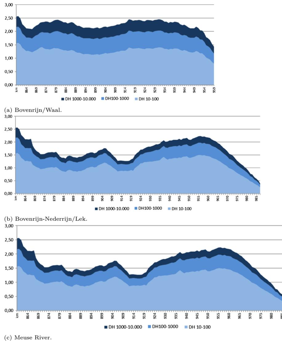
Figure 2.3: Cumulative decimation heights for the Bovenrijn-Nederrijn/Lek, Bovenrijn-Waal and Meuse River. The figure depicts the differences in flood water levels with probabilities of occurrence ranging from 1:10 to 1:10,000 per year. On the x-axis, the chainage of the corresponding branch is denoted (Hegnauer et al., 2014; Klijn et al., 2018).
