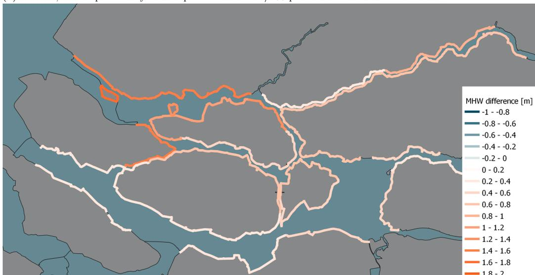
(c) Delta21, failure probability of Europoort barrier of 1/100 per closure and 2 m sea level rise.
