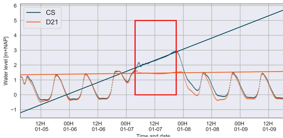
(a) Water level at Rotterdam over simulation period. The dots indicate the output of the hydrodynamic model. The two straight lines are fitted to the dots present in the red rectangle.
