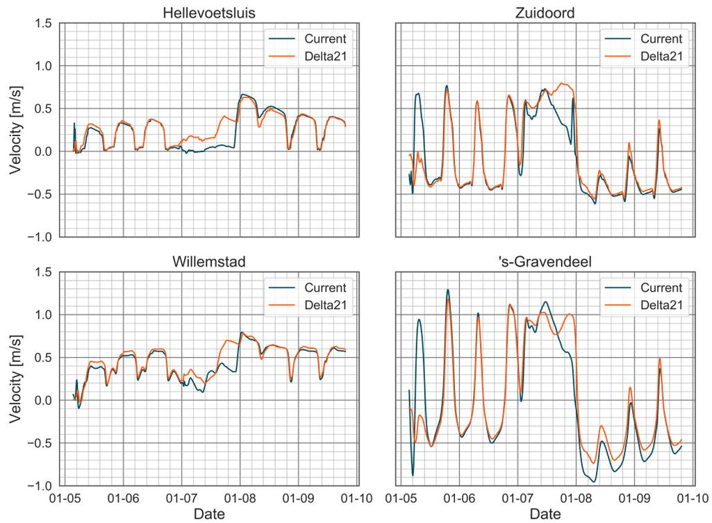
Figure 4.10: Velocities for both configurations during a storm with a Rhine discharge ( $Q_{\text{Lobith}}$ ) of  $10\,000\text{ m}^3/\text{s}$  and storm surge ( $L$ ) of  $3.54\text{ m}$ . Locations are in the flood storage dominant area.
