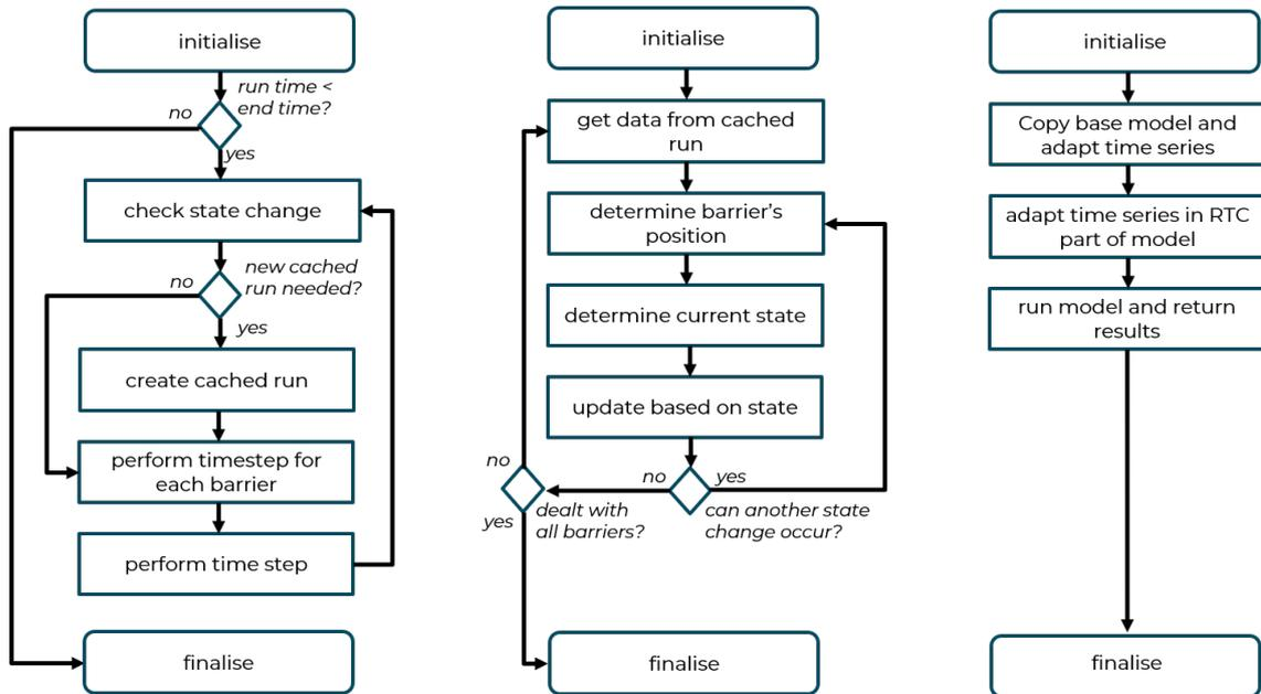
Figure B.3: Various loops of Singlerunner. The left loop investigates whether a new cached run is needed, the loop in the middle updates the state and corresponding position of the barrier and the right loop writes the results of the RTC to SOBEK (Adjusted from Deltares (2018)).
