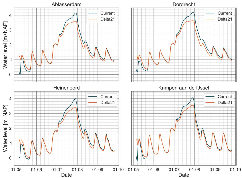
Figure 4.16: Water levels for both configurations during a storm with a Rhine discharge ( $Q_{\text{Lobith}}$ ) of  $10\,000\text{ m}^3/\text{s}$  and storm surge ( $L$ ) of  $3.54\text{ m}$ . Locations are in the transition area.
