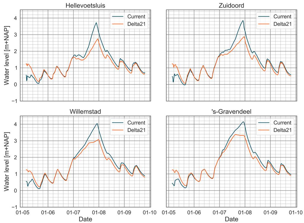
Figure 4.8: Water levels for both configurations during a storm with a Rhine discharge ( $Q_{\text{Lobith}}$ ) of  $10\,000\text{ m}^3/\text{s}$  and storm surge ( $L$ ) of  $3.54\text{ m}$ . Locations are in the flood storage dominant area.
