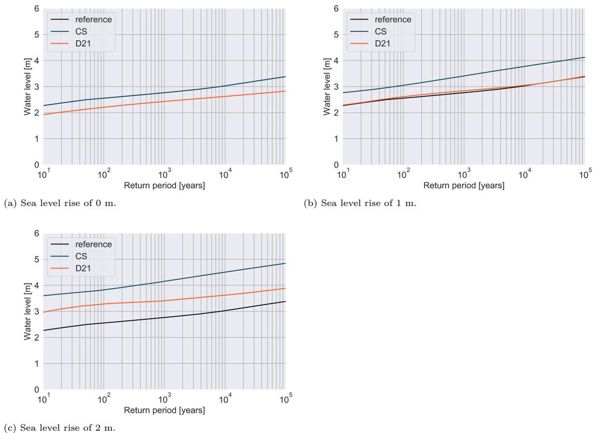
Figure 5.10: Water level frequency lines at Dordrecht for different sea level rise. The current system is indicated with the blue line, Delta21 with the orange line.
