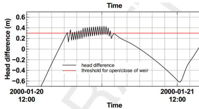
Figure B.1: Illustration of on-off control of the Haringvliet sluices triggered by the head difference (Deltares, 2019).
