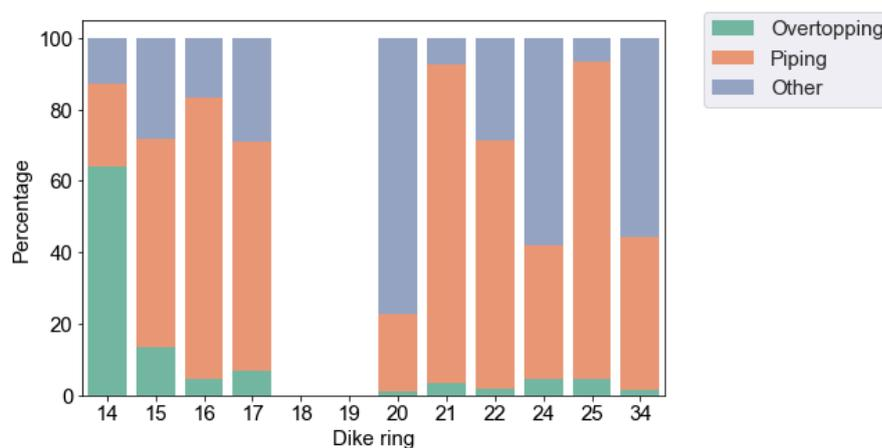
Figure 6.3: Contribution of failure mechanisms piping and height in total failure probability. Per dike ring, the share of the failure probability for piping and height is computed. The distribution belongs to the current situation without sea level rise (Based on data of Vergouwe (2015)).
