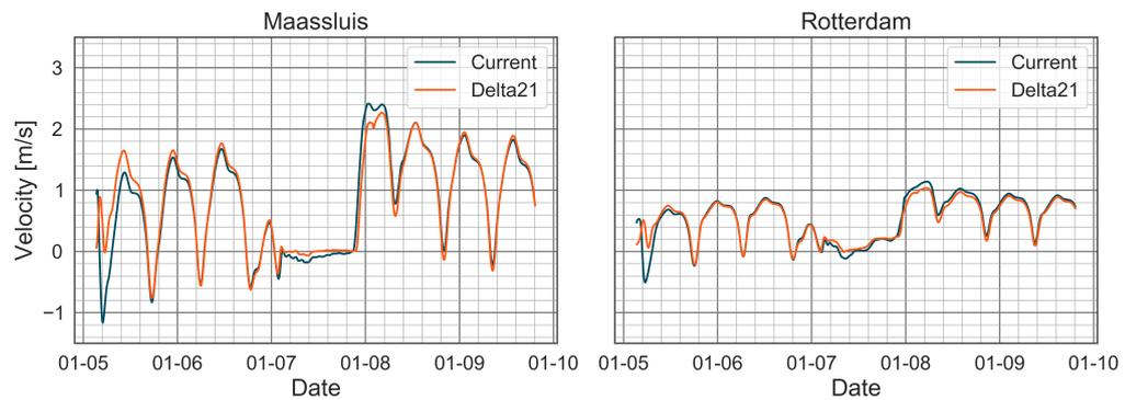
Figure 4.6: Velocities for both configurations during a storm with a Rhine discharge ( $Q_{\text{Lobith}}$ ) of  $10\,000\text{ m}^3/\text{s}$  and storm surge ( $L$ ) of  $3.54\text{ m}$ . Locations are in the storm surge dominant area.
