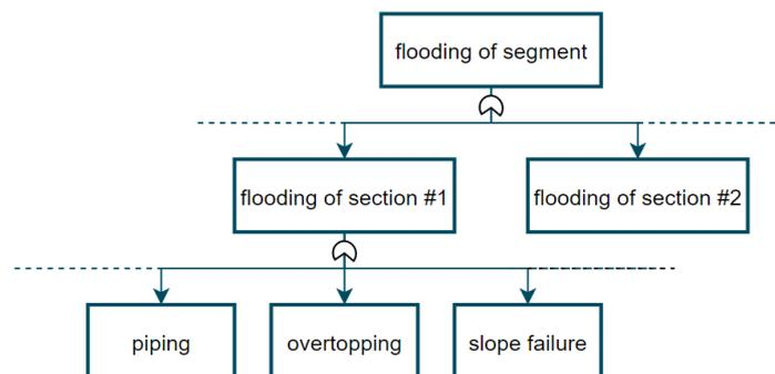
Figure 3.8: Fault tree of a dike segment. Different failure mechanisms are involved in the failure of the dike. On a dike section level, the probabilities are determined and translated to a dike segment level (adjusted from Jonkman et al. (2018)).
