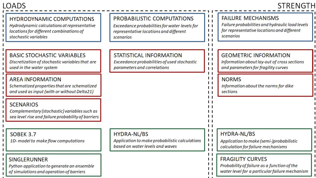
Figure 3.1: Structure of modelling approach. The blue boxes indicate the different steps undertaken in this research. The results of the hydrodynamic computations, probabilistic computations and failure mechanisms are discussed in Chapter 4, 5 and 6 respectively. The boxes with a red outline indicate which information serves as input, where the green boxes represent the used application or method.
