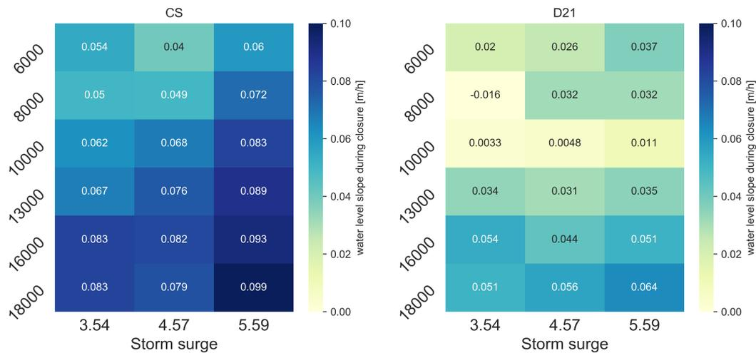
(a) Water level gradient for current system.
