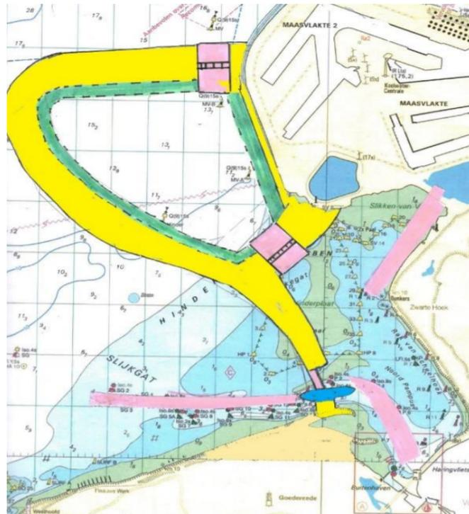
Figure 2.5: Illustration of the Delta21 plan (Delta21, 2019). The energy storage lake is constructed within the yellow dike sections. Between the Haringvliet sluices (bottom right) and the energy storage lake, a tidal lake is created. This tidal lake is connected to the North Sea with a storm surge barrier in between.
