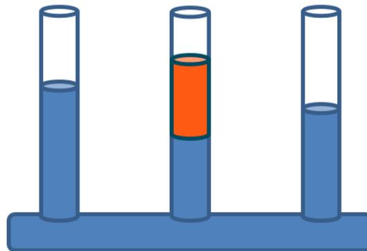
Figure 16.3: Illustration of communicating vessels.
