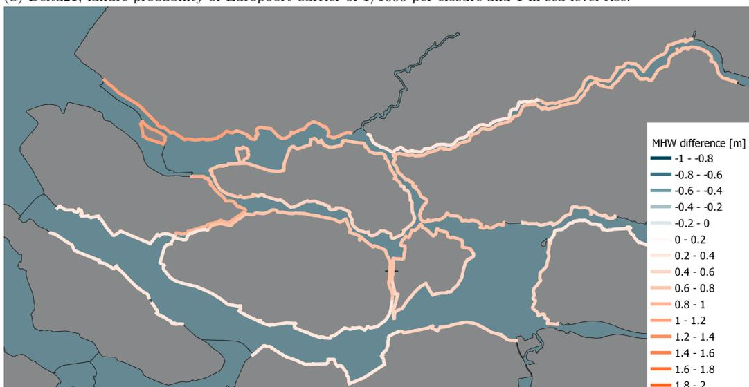
(c) Delta21, failure probability of Europoort barrier of 1/1000 per closure and 2 m sea level rise.
