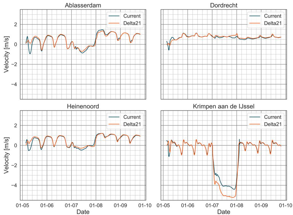
Figure 4.18: Velocities for both configurations during a storm with a Rhine discharge ( $Q_{\text{Lobith}}$ ) of  $10\,000\text{ m}^3/\text{s}$  and storm surge ( $L$ ) of  $3.54\text{ m}$ . Locations are in the transition area.
