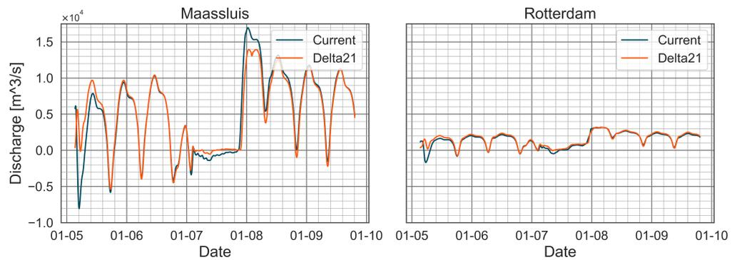
Figure 4.5: Discharges for both configurations during a storm with a Rhine discharge ( $Q_{\text{Lobith}}$ ) of  $10\,000\text{ m}^3/\text{s}$  and storm surge ( $L$ ) of  $3.54\text{ m}$ . Locations are in the storm surge dominant area.
