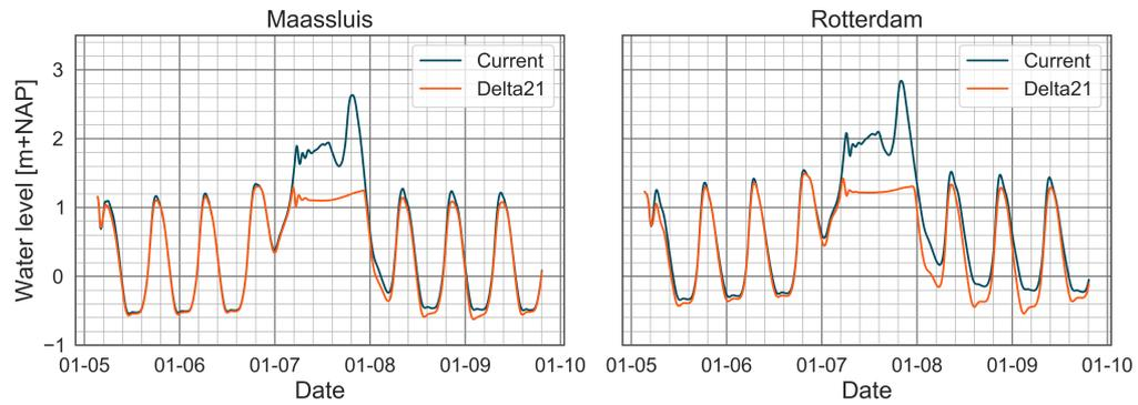
Figure 4.4: Water levels for both configurations during a storm with a Rhine discharge ( $Q_{\text{Lobith}}$ ) of  $10\,000\text{ m}^3/\text{s}$  and storm surge ( $L$ ) of  $3.54\text{ m}$ . Locations are in the storm surge dominant area.
