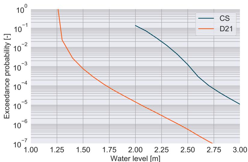
Figure 4.19: Exceedance probability of water level at Willemstad. The current system is depicted in blue and Delta21 is rendered in orange. Willemstad is located right next to the Volkerak sluices. In case of Delta21, the threshold water level of NAP+ 2.6 m is exceeded less.
