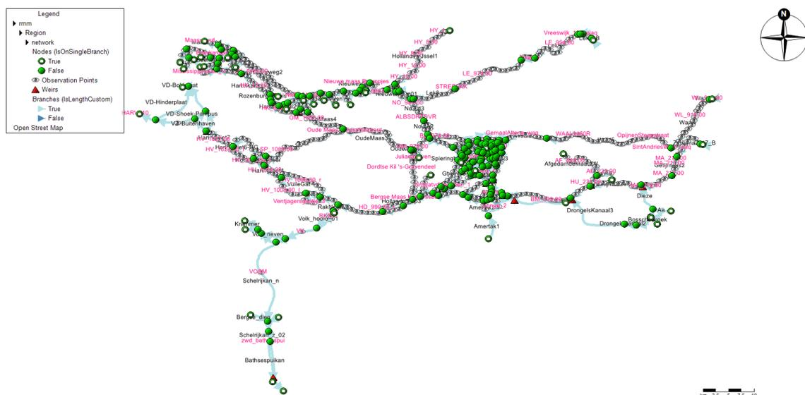
Figure 3.5: The RMM-model in SOBEK3. The arrows and green dots represent the branches and nodes respectively. Moreover, all structures are included. The boundaries on the east side of the domain are governed by the discharge of the rivers Lek, Waal and Maas. The boundary nodes on the west side are governed by the water level at the North Sea.
