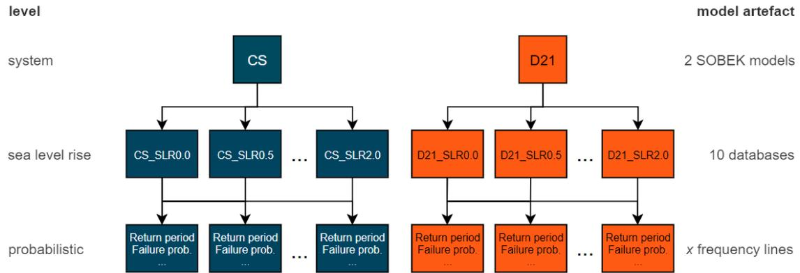
Figure 3.7: Graphical representation of the simulation approach. The blue boxes indicate simulations in which the current system is used. The orange boxes represent simulations with the properties of Delta21. For each step of sea level rise of 0.5 meters, 164 simulations are made corresponding to 9 discharges, 6 storm surges and three operation states of the Europoort barrier.
