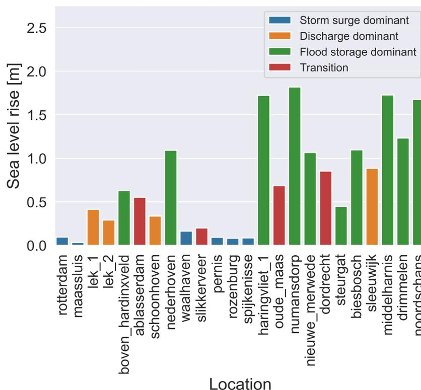
Figure 5.16: Amount of sea level rise mitigated by Delta21. For various locations throughout the current governing high water level without Delta21 and without sea level rise is compared to a situation with Delta21. The amount of sea level rise indicated up to which Delta21 succeeds in keeping the governing water level lower or equal to the current governing high water level.
