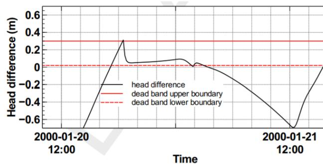
Figure B.2: Illustration of dead-band control of the Haringvliet sluices triggered by the head difference (Deltares, 2019).
