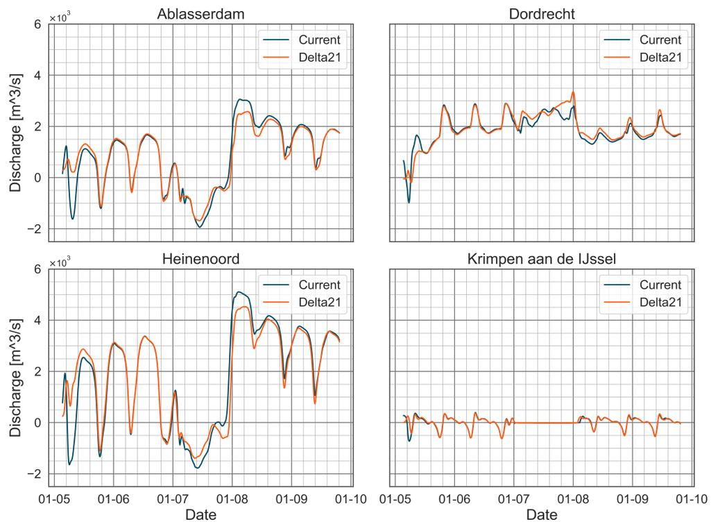
Figure 4.17: Discharges for both configurations during a storm with a Rhine discharge ( $Q_{\text{Lobith}}$ ) of  $10\,000\text{ m}^3/\text{s}$  and storm surge ( $L$ ) of  $3.54\text{ m}$ . Locations are in the transition area.
