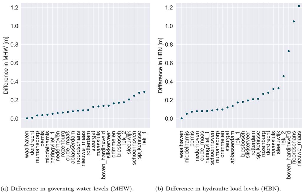
Figure 3.6: Comparison of MHWp5 database to the WBI database. The difference - in absolute values - between the databases for the water levels and hydraulic load levels for different locations throughout the Rhine-Meuse estuary. The values are sorted from lowest to highest.
