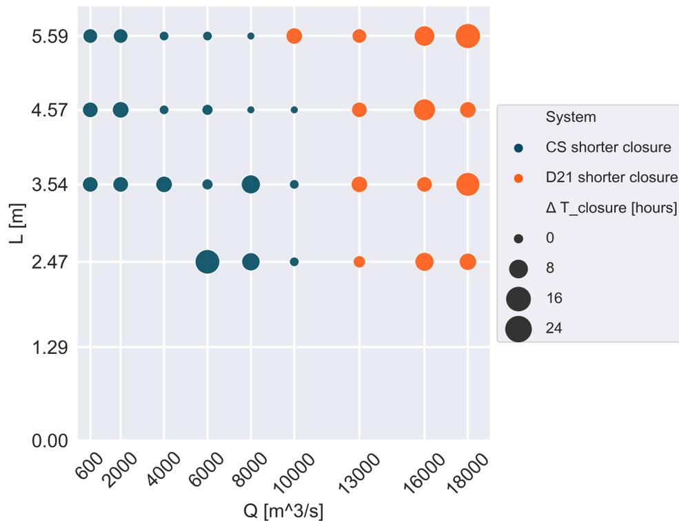
Figure 4.22: Difference in closure duration of the current configuration and a configuration with Delta21. The size of the circles indicates difference in number of hours. An blue circle corresponds to a shorter closure of the current configuration, an orange circle represents an shorter closure for Delta21.
