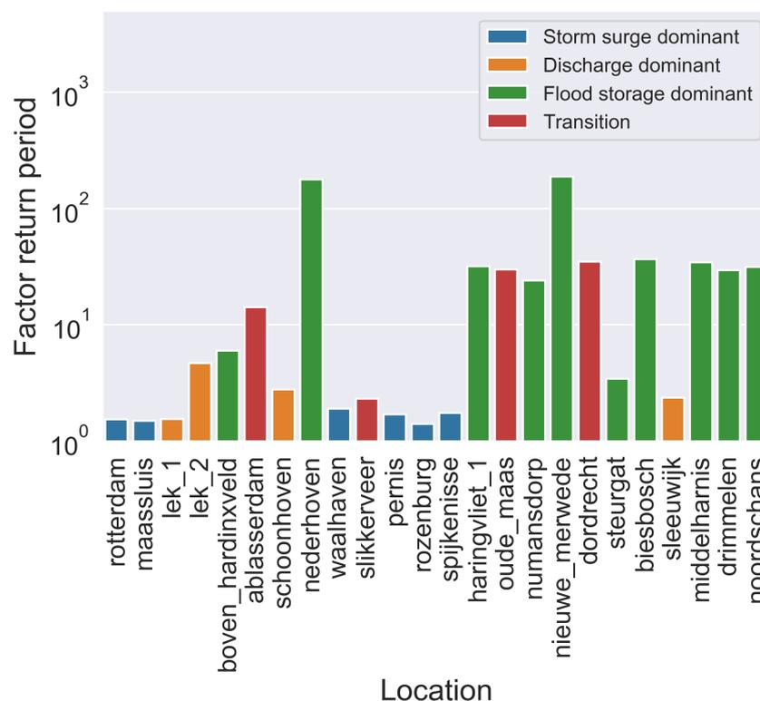
Figure 5.11: Factor return period for different locations. This factor indicates the ratio between return periods for the current system and Delta21 for a particular water level. Note that the scale on the vertical axis is logarithmic.
