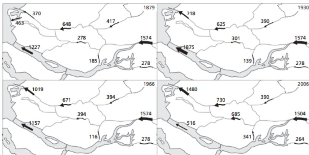
Figure 2.1: Division of mean river discharge (in  $\text{m}^3/\text{s}$ ) over channels in the RMD over the past century (Huisman and Hoitink, 2017). Major changes in discharge can be observed in the Nieuwe Waterweg and Haringvliet.
