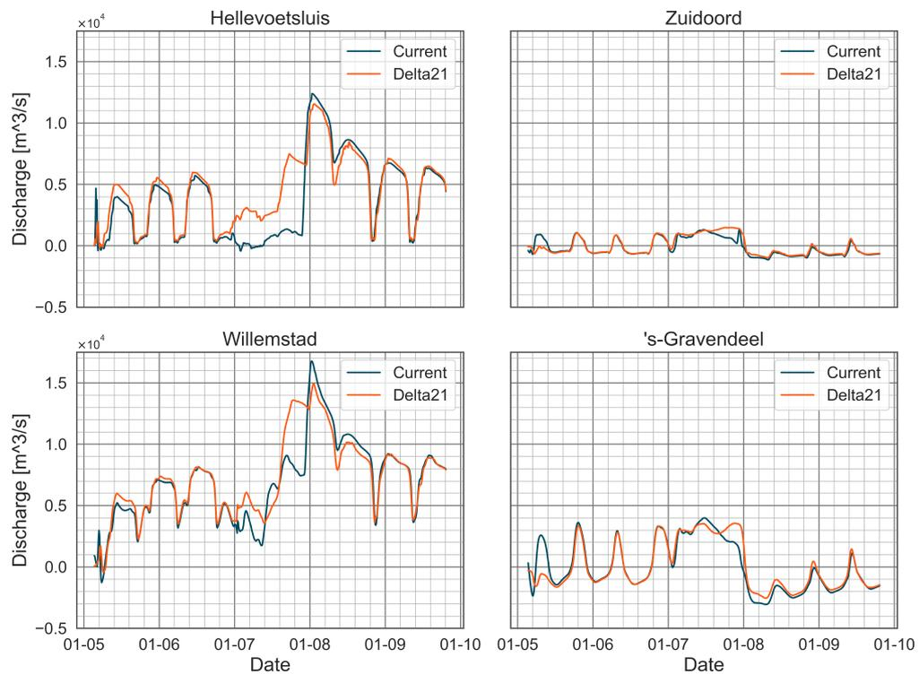
Figure 4.9: Discharges for both configurations during a storm with a Rhine discharge ( $Q_{\text{Lobith}}$ ) of  $10\,000\text{ m}^3/\text{s}$  and storm surge ( $L$ ) of  $3.54\text{ m}$ . Locations are in the flood storage dominant area.
