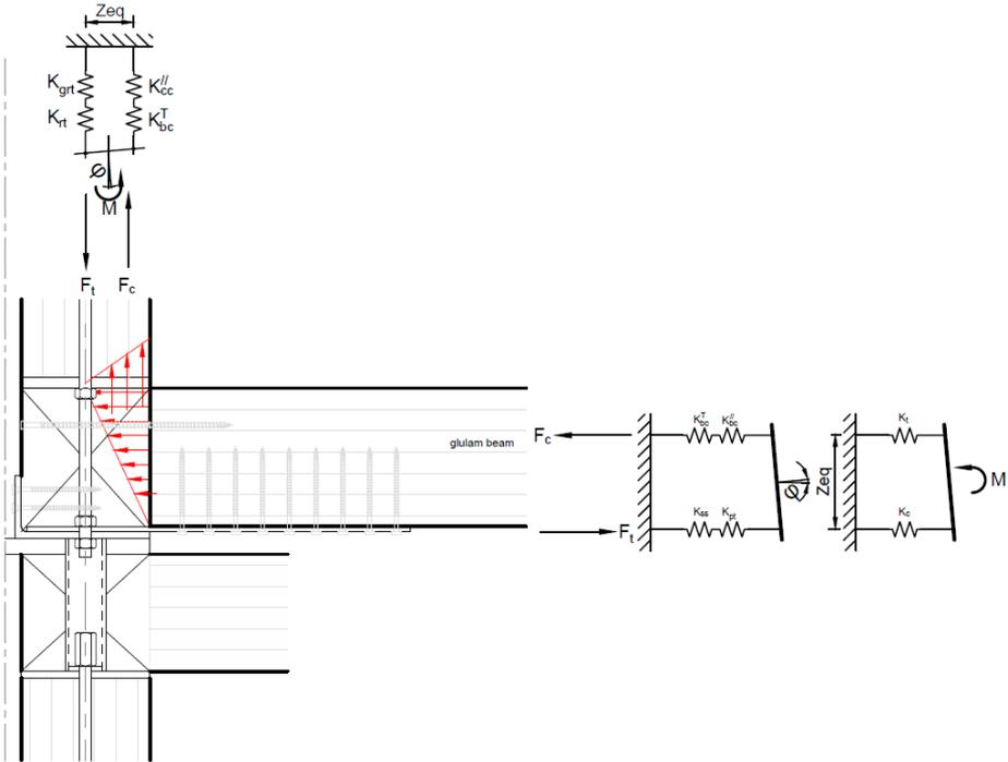
Figure 7.10: Rotational spring model for combination of the intra- and inter modular connection in case of a closing moment  $\theta^-$
