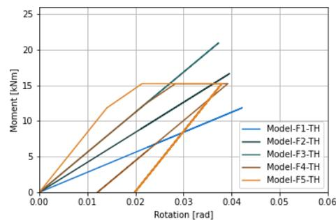
**Figure 9.3:** Time history results for moment-rotation floor beam-column connection of parameter study scenario F
