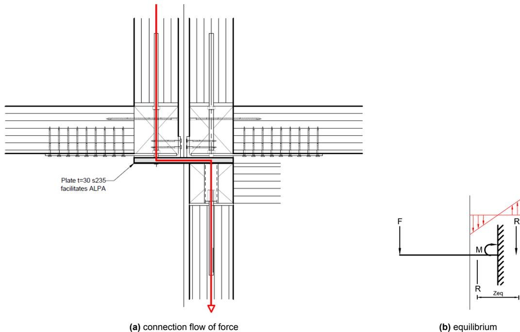
Figure B.1: Alternative load path of steel plate in the inter-modular connection
