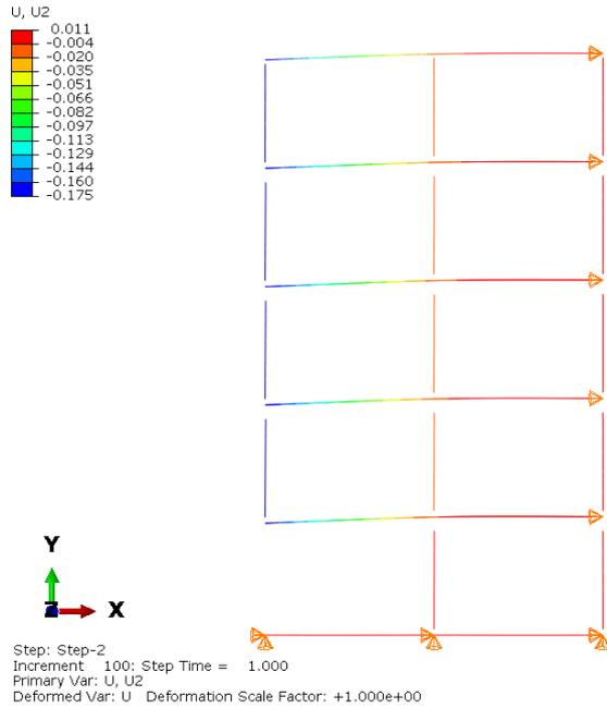
Figure 8.21: Vertical displacement [m] at failure NLS-analysis scenario E
