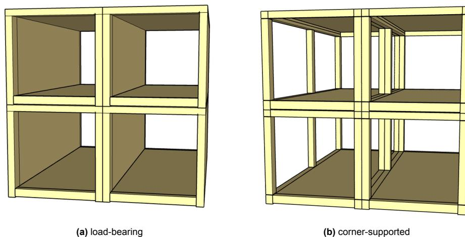
Figure 4.2: 2 different module forms
