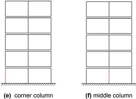
Figure 7.19: Removal scenarios side view in analysis model-2
