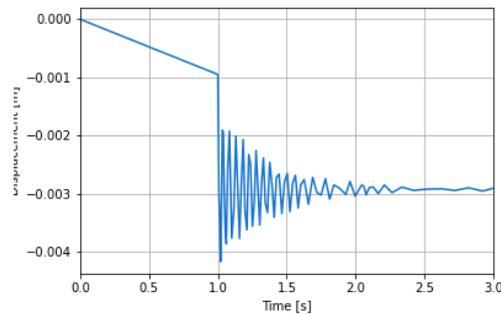
Figure 8.20: time history response at node removed column scenario D
