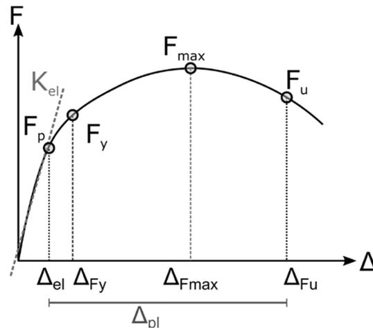
Figure 3.2: Example of ductile load-displacement curve with elastic and plastic displacements [26]
