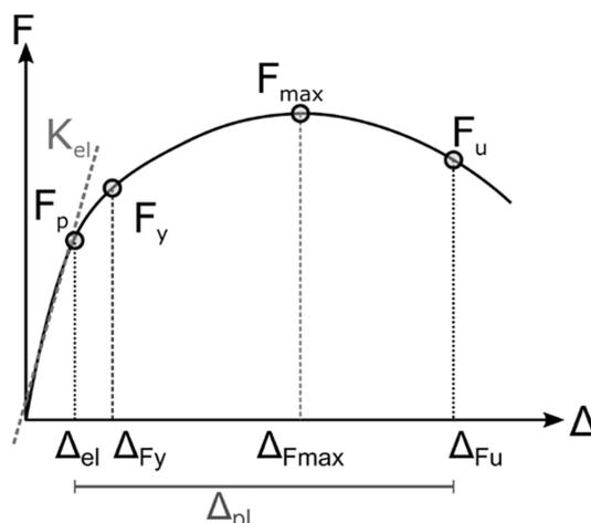
Figure 6.1: Example of ductile load-displacement curve with elastic and plastic displacements [26]
