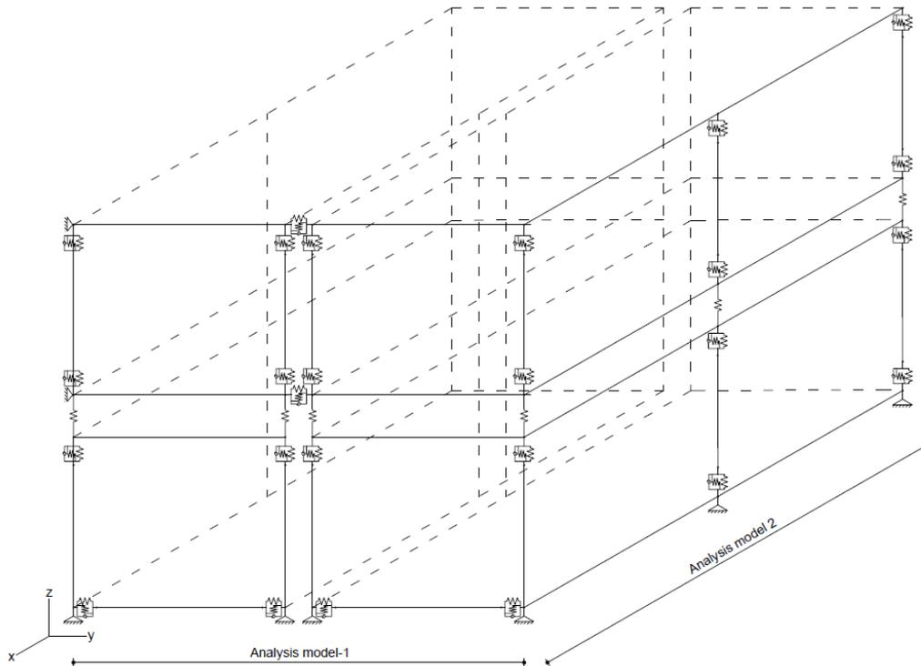
**Figure 7.13:** Illustration of 3D model with springs replacing the connections
