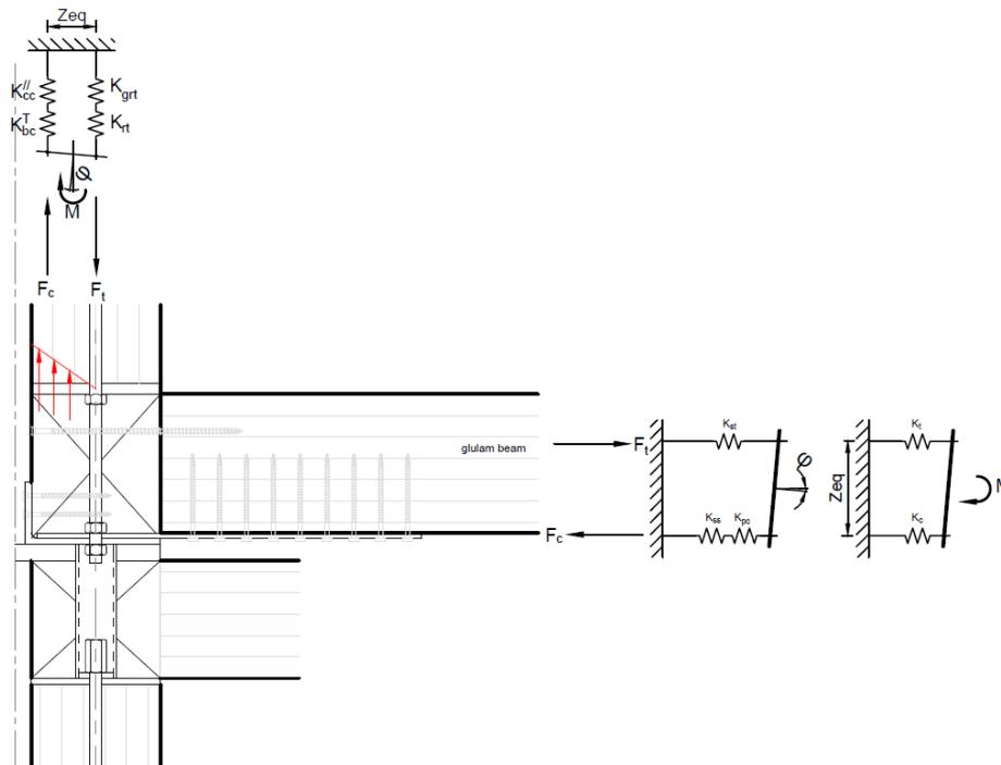
**Figure 7.9:** Rotational spring model for combination of the intra- and inter modular connection in case of a opening moment  $\theta^+$
