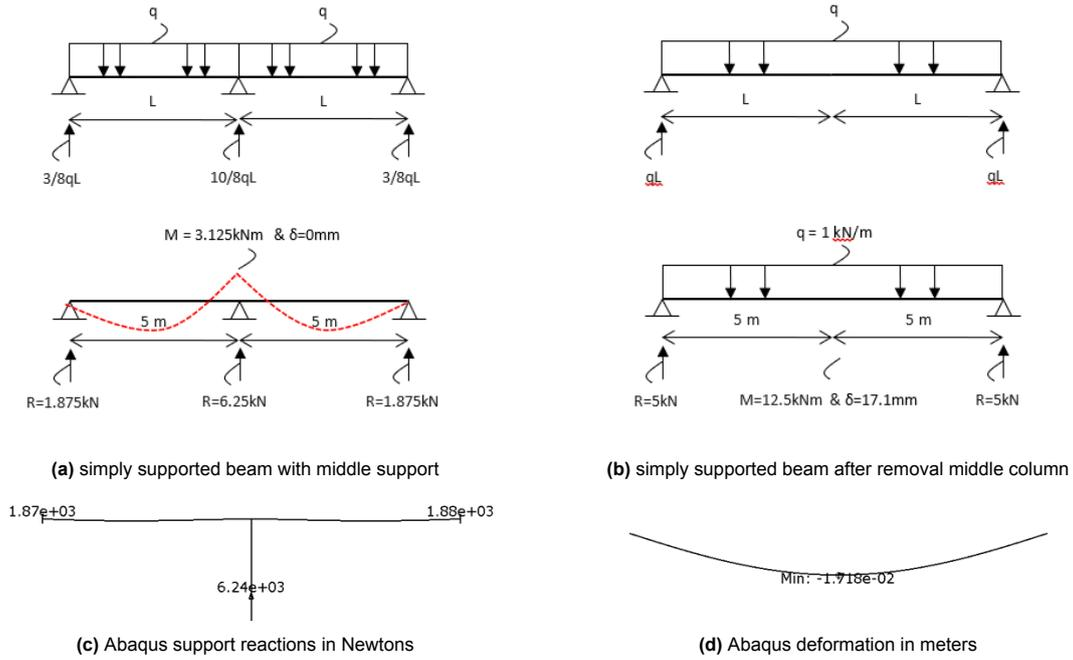
Figure 7.24: Simple model validation with analytical and fem results for static loading
