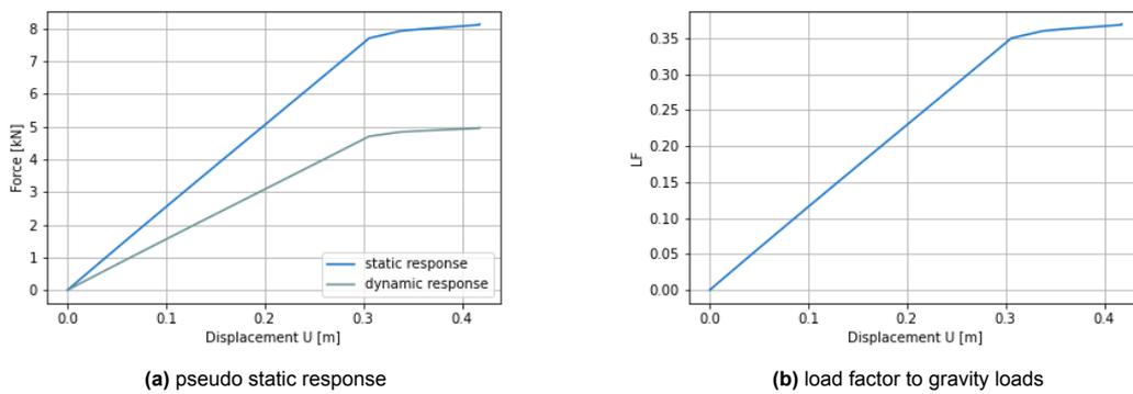
Figure 8.2: Push-down response curves scenario A
