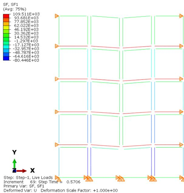
Figure 8.14: Section normal forces scenario C
