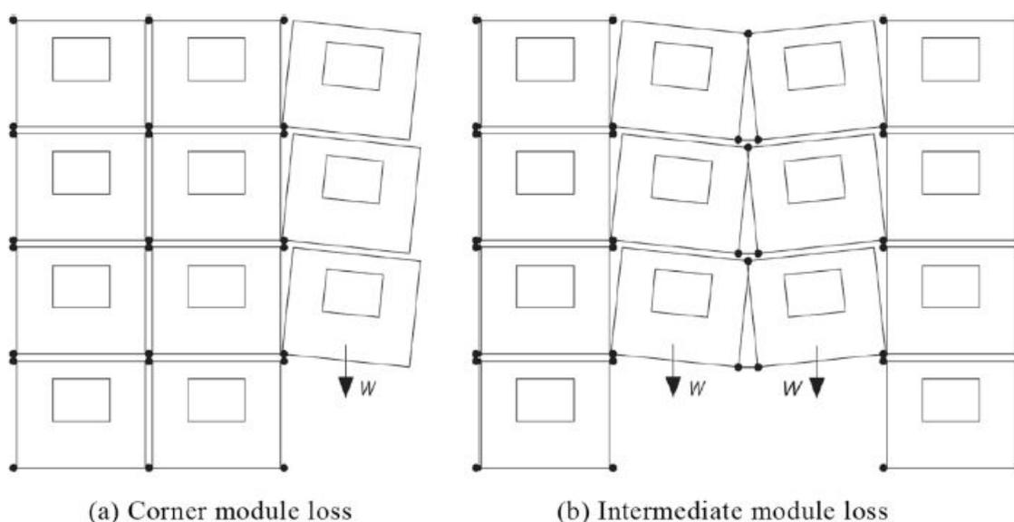
Figure 4.7: Module loss scenario [16].
