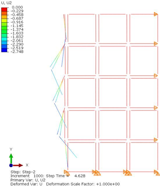
Figure 8.6: Collapsed area in time history analysis scenario A
