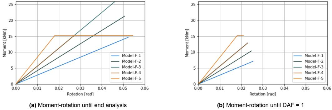
Figure 9.4: Moment-rotation output for floor beam-column connection of variants F - NLS
