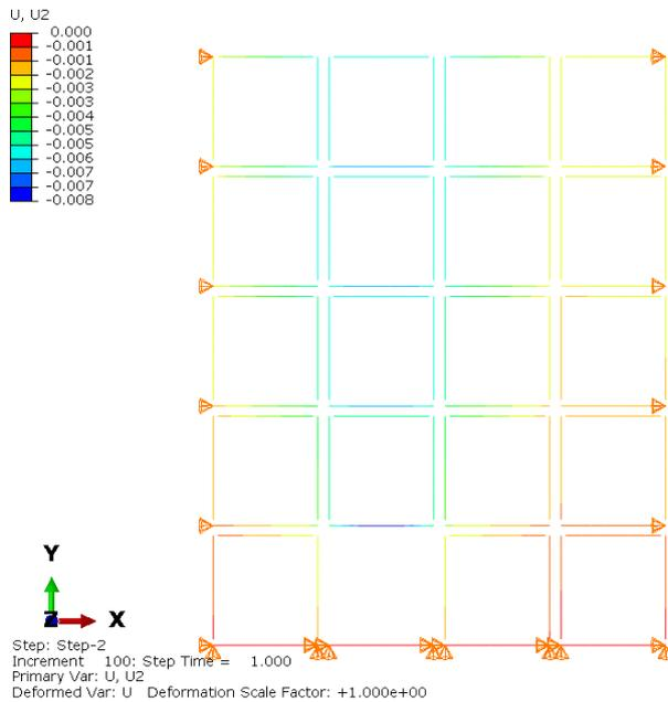
Figure 8.18: Vertical displacement [m] at failure NLS-analysis scenario D
