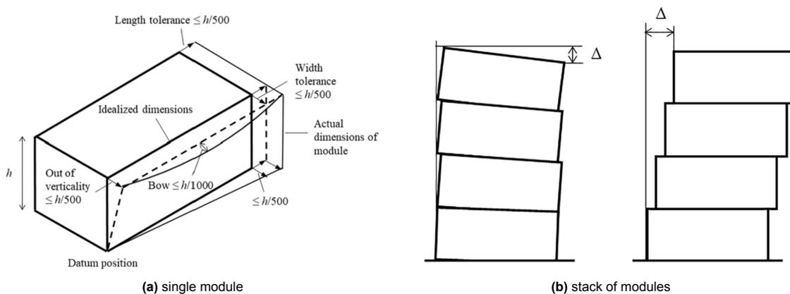
Figure 4.5: Construction tolerances of modular buildings [31].
