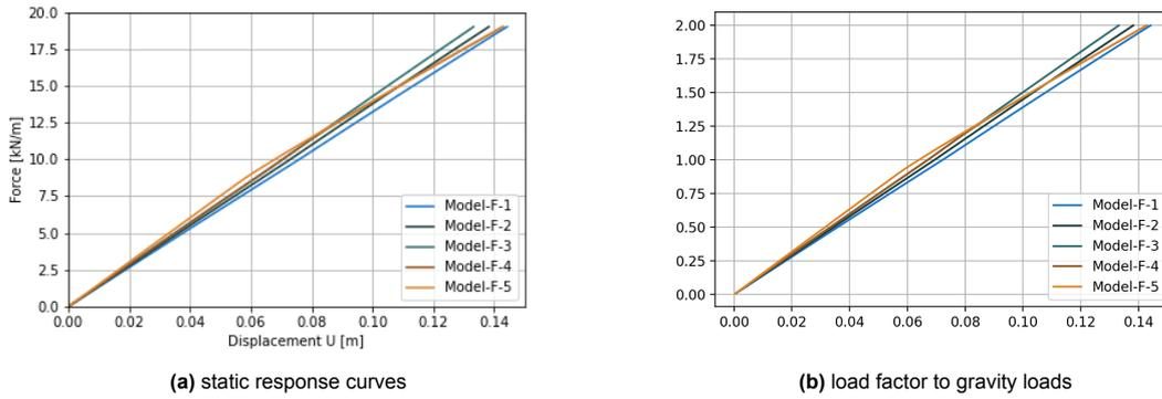
Figure 8.29: Push-down curves parameter study scenario F
