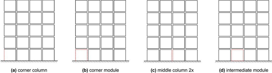
Figure 7.18: Removal scenario's front view in analysis model-1
