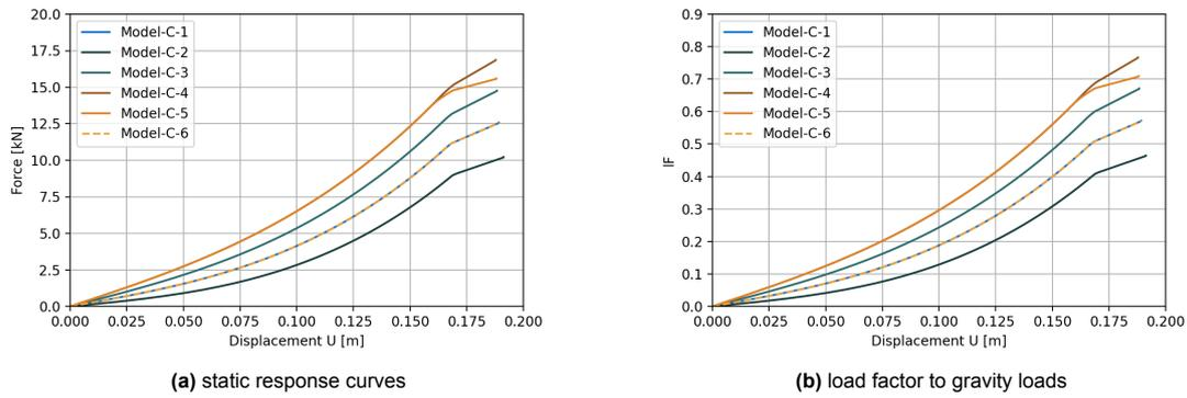
Figure 8.28: push-down curves parameter study scenario
