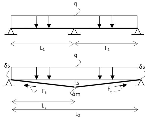
**Figure 9.6:** Schematic representation of catenary action
