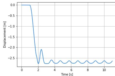
Figure 8.4: Time history response at node removed column scenario A
