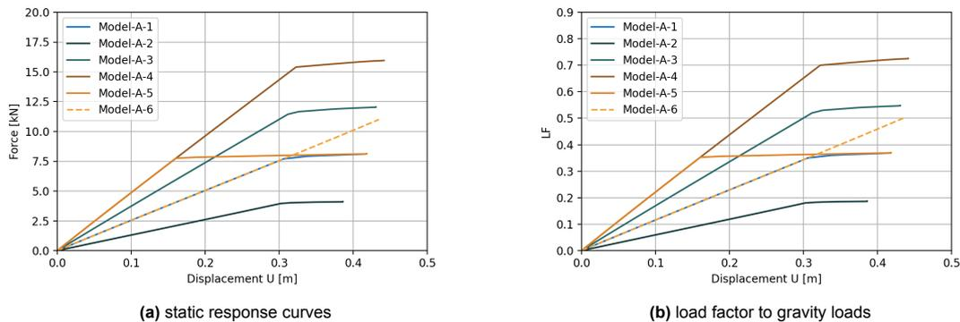
**Figure 8.27:** Push-down curves parameter study scenario A
