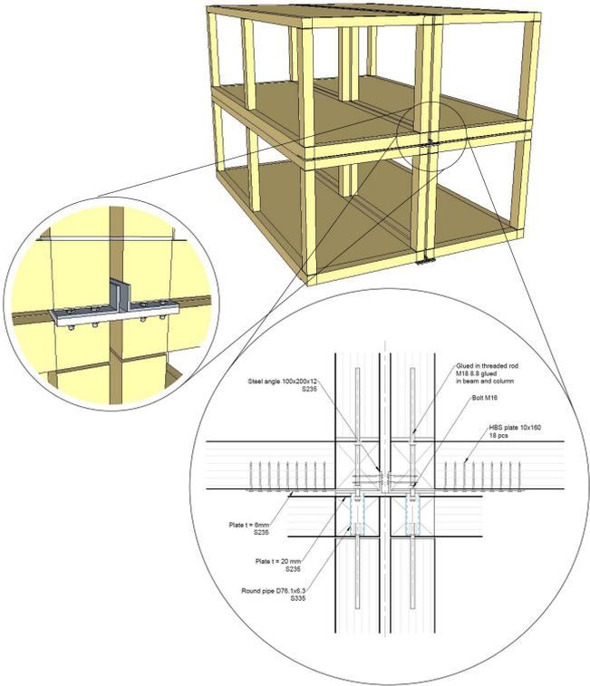
Figure 7.5: Inter-modular connection location
