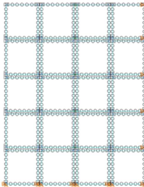
Figure 7.22: Figure with meshed elements representing analysis model 1 in the Abaqus environment
