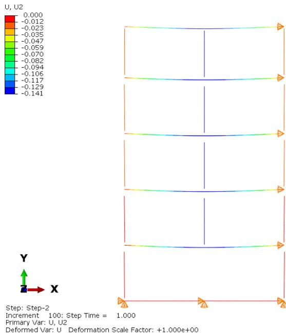
**Figure 8.24:** Vertical displacement [m] at failure NLS-analysis scenario F
