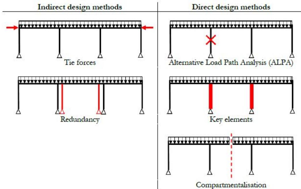
Figure 3.3: Direct and indirect design methods for robustness [35].
