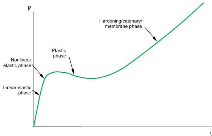
Figure 5.3: Phases of failure [21]
