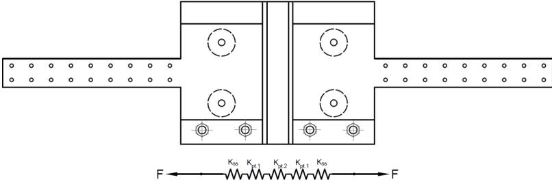
**Figure 7.12:** Translational spring inter-modular connection
