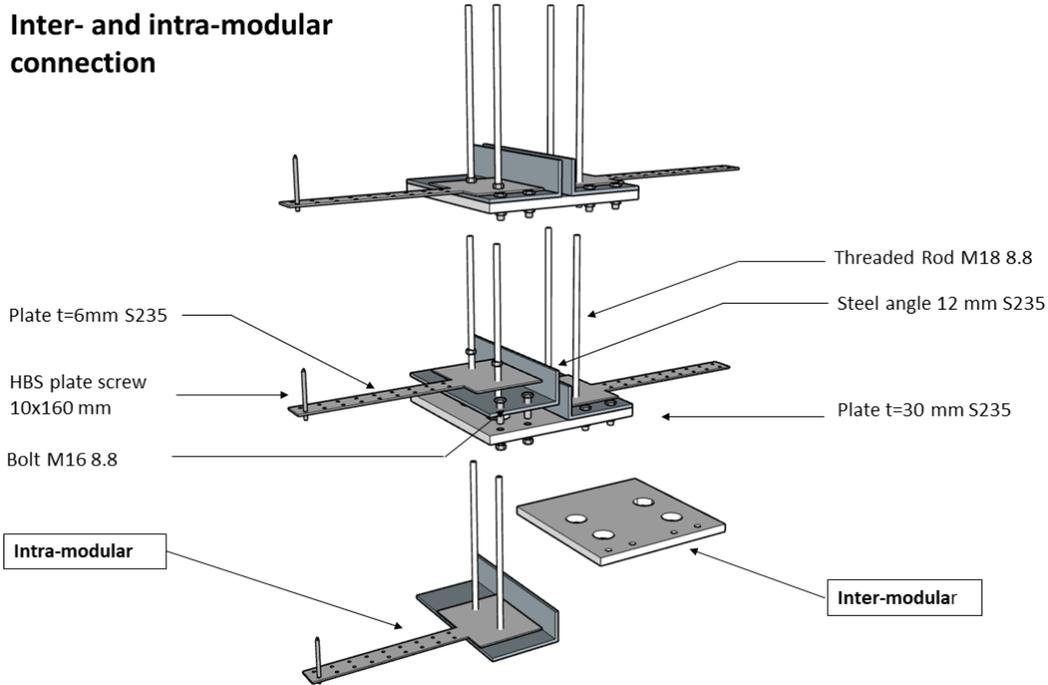
**Figure 7.7:** 3D overview of combined intra- and inter-modular connection their components
