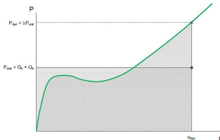
Figure 5.1: Push-down curve for dynamic response [21]
