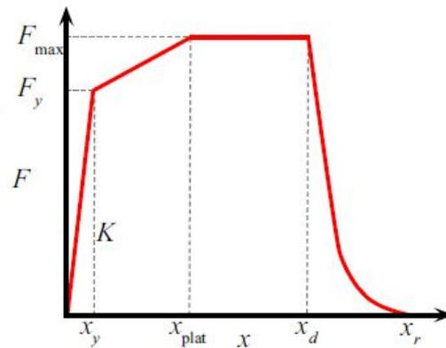
Figure A.2: Generic connector behaviour with failure motion [10].
