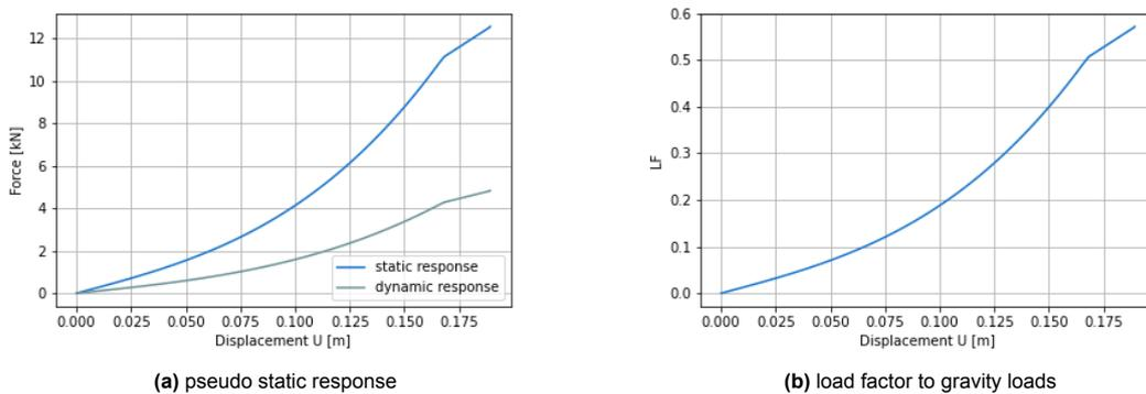
Figure 8.12: Push-down response curves scenario C
