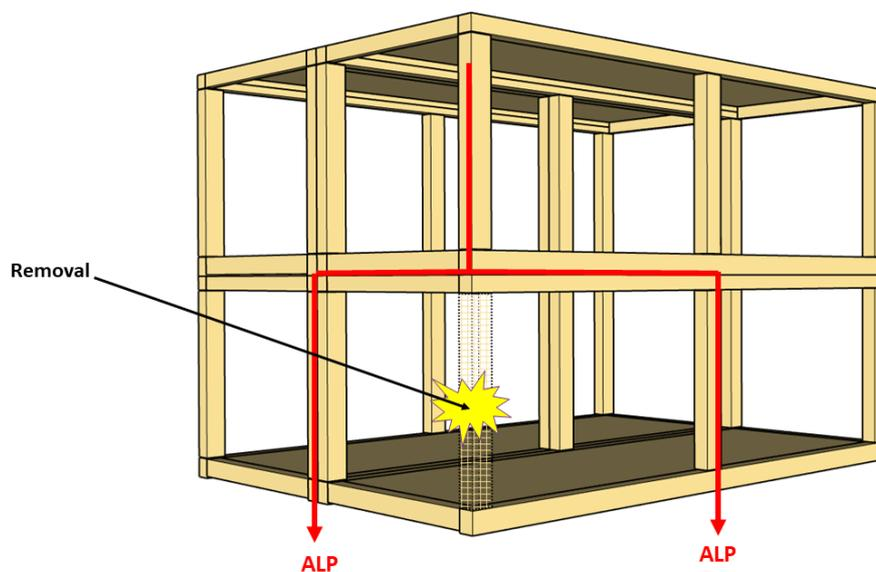
**Figure 1:** Case study example of alternative load path analysis in volumetric timber post and beam module
