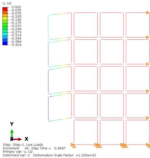
Figure 8.7: Vertical displacement [m] at failure NLS-analysis scenario B
