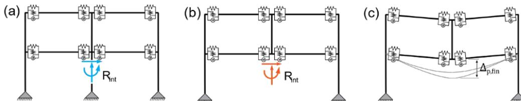
**Figure 7.21:** Adapted from Cao et al. a) Determining reactions (b) Apply reaction forces in model without column (c) Dynamic response. [4]
