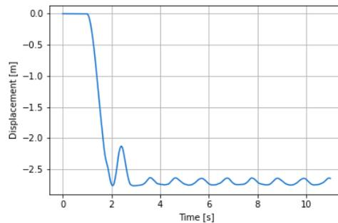
Figure 8.10: Time history response at node removed column scenario B
