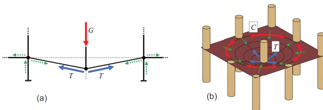
Figure 3.1: Catenary (a) and Membrane Action (b) [11].
