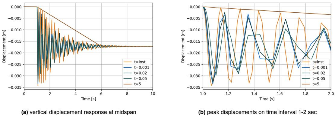
Figure 7.25: Effects of element removal speed in dynamic response
