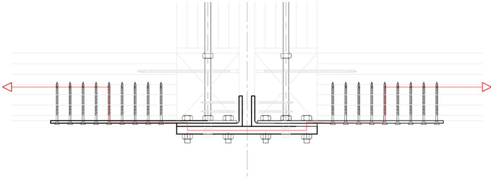
Figure 7.11: Inter-modular connection flow of force for horizontal tie
