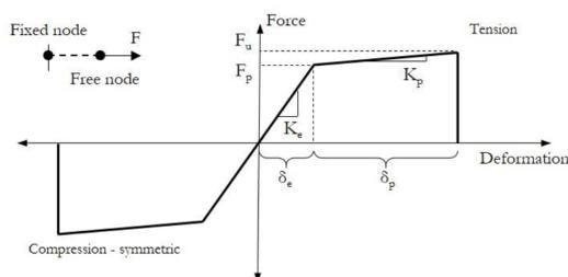
Figure A.1: Idealised connector behaviour for axial degree of freedom [35].
