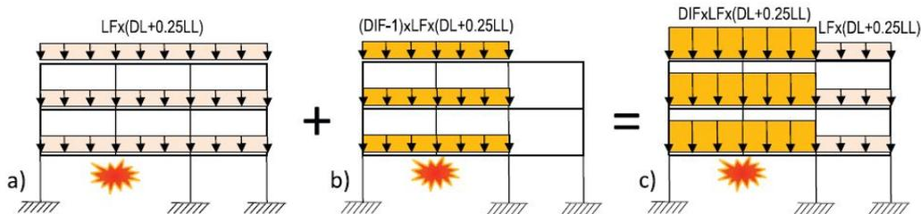
**Figure 7.20:** a) Push 1: Preliminary push-down analysis under unamplified gravity loads. (b) Push 2: Push-down analysis under additional gravity loads in the bays affected by column removal. (c) Push-down analysis under amplified gravity loads. [8]
