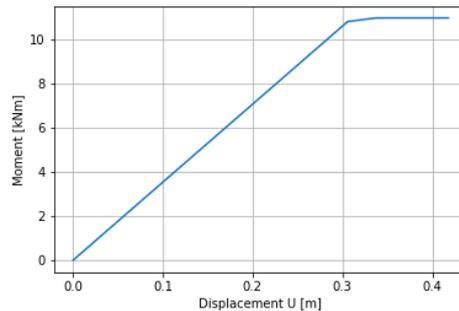
Figure 8.3: Moment response curve of the floorbeam - column connection
