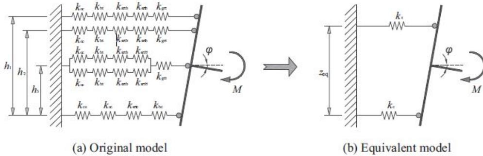
Figure 6.2: Mechanical model beam-column connection [36]
