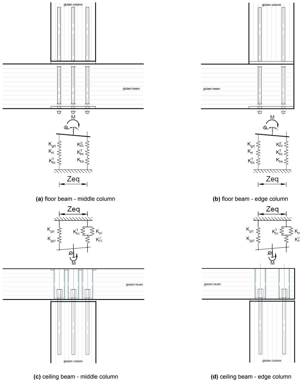
Figure 7.8: Equivalent spring models intra-modular connections
