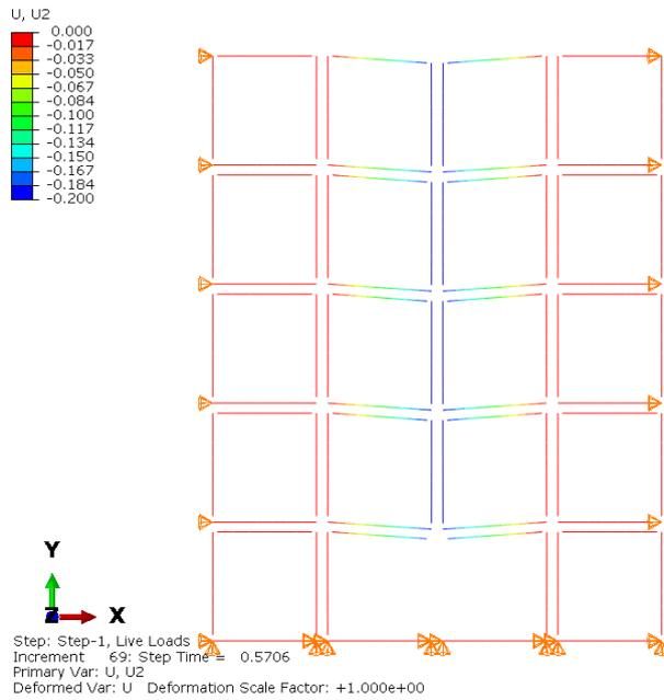
Figure 8.11: Vertical displacement [m] at failure NLS-analysis scenario C
