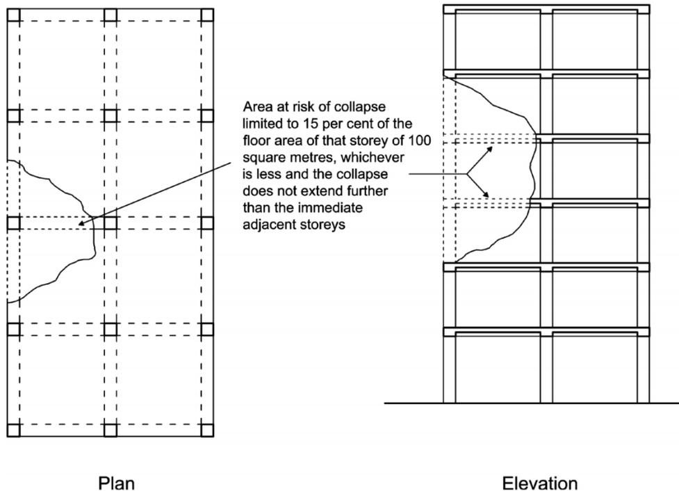
**Figure 3.5:** Recommended limit for resulting damage
