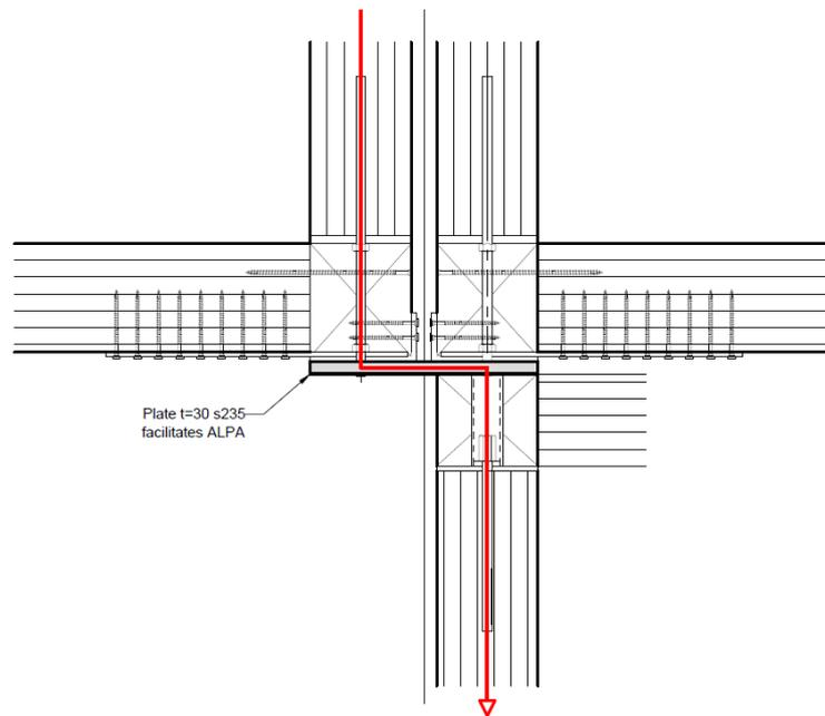
**Figure 9.2:** Alternative load path of steel plate in the inter-modular connection
