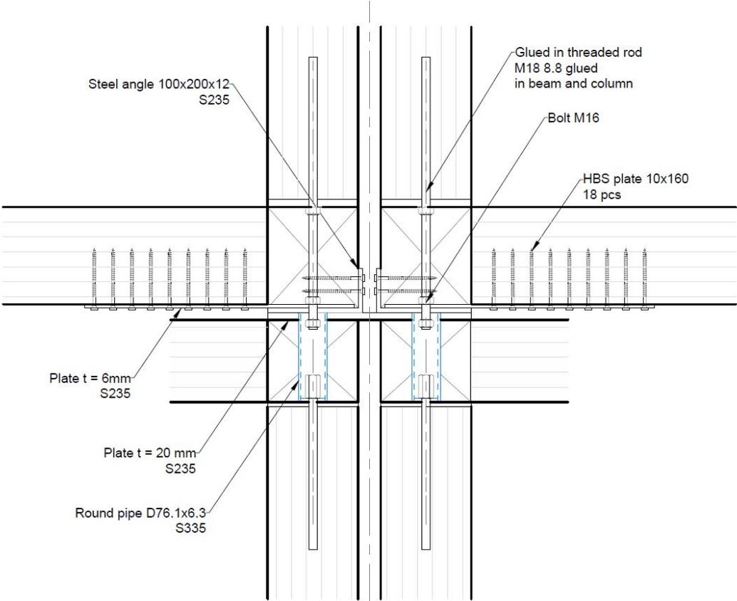
Figure 7.6: Inter-modular connection
