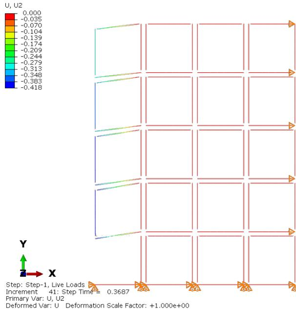
Figure 8.1: Vertical displacement [m] at failure NLS-analysis scenario A
