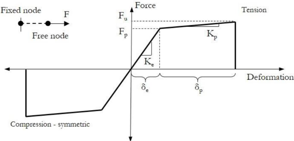
Figure 5.5: Idealised connector behaviour for axial degree of freedom [35].
