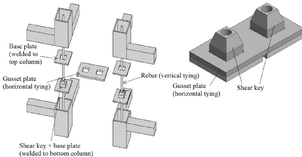
Figure 4.4: Common tie rod connection with gusset plate [31]
