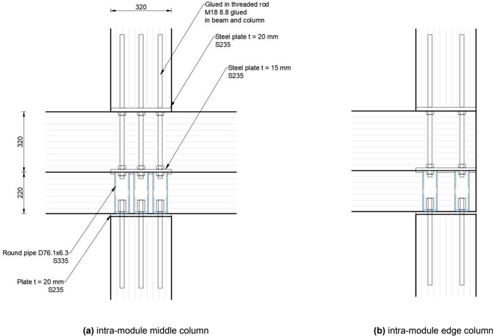
Figure 7.4: Details of intra-modular connections
