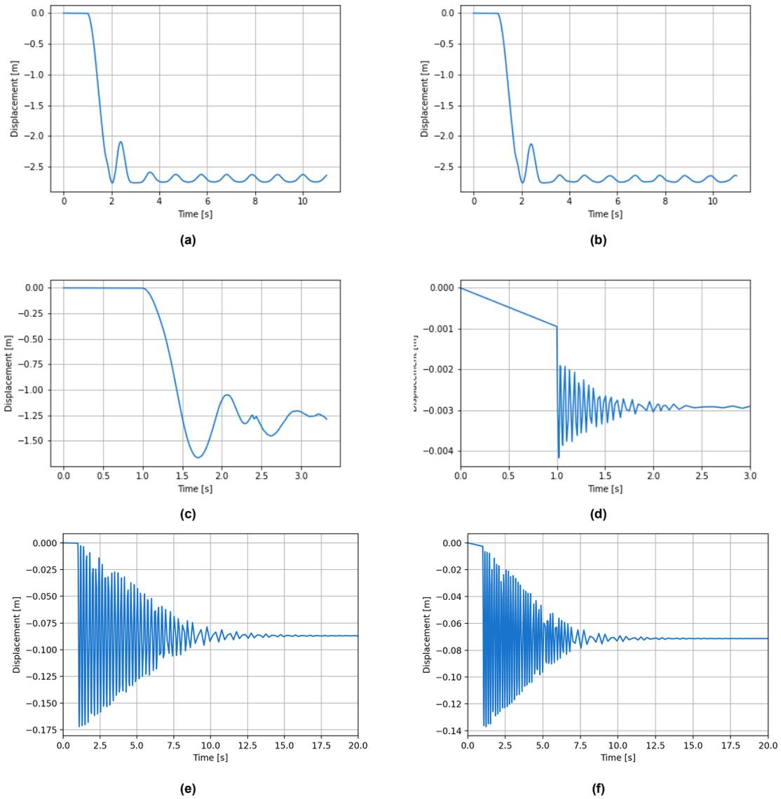
**Figure C.2:** Displacement time history response for removal scenarios a) till f)
