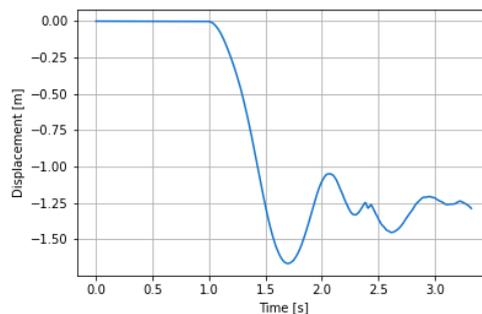
Figure 8.16: Time history response at node removed column scenario C
