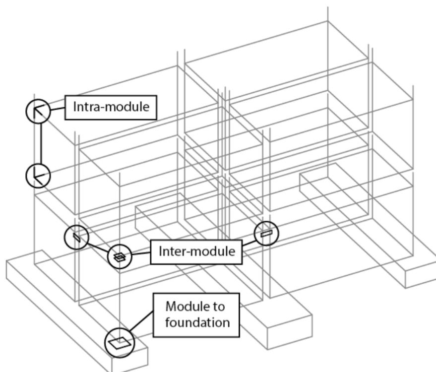
Figure 4.3: 3 connection categories in modular construction [16].
