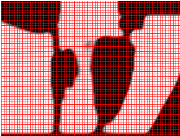
Figure G.7: Image showcasing the mesh fidelity used in the topology optimization.
