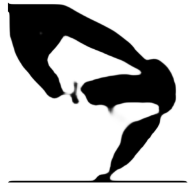
(c) Optimized topology for a spring stiffness of 200 [N/mm]
