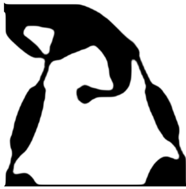
(a) Optimized topology for a spring stiffness of 25 [N/mm]
