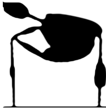
(b) Optimized topology for a spring stiffness of 100 [N/mm]
