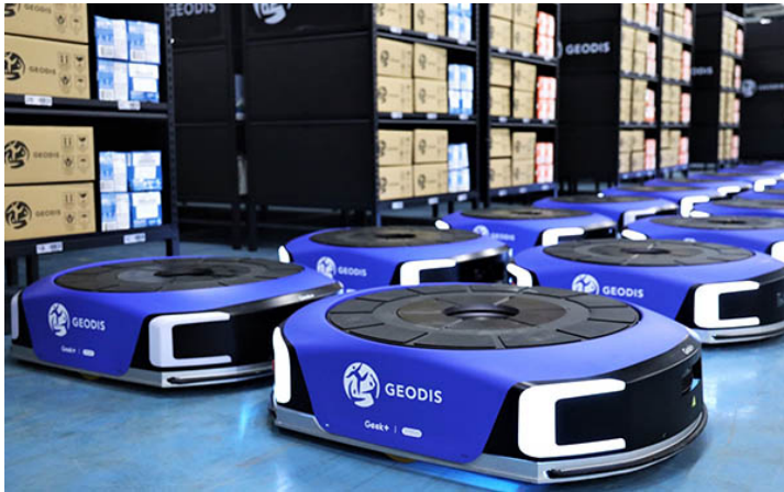
Figure 1.1: AMRs by Geek+ that can be used in RMFSs to transport pods (Robotics 24/7 Staff 2021).
