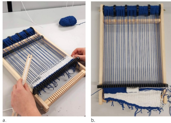
Figure 9 The frame loom in operation with five 3D-printed beams and a comb. Each beam can be tensioned separately, and the comb helps to keep the woven fabric in place as the warp is tightened. (a) The weaver uses a partial weft to weave additional areas. (b) After re-tensioning behind the comb, the textile forms a non-rectangular zone while the fell (last row woven) is kept straight to enable successive free-form weaving.
