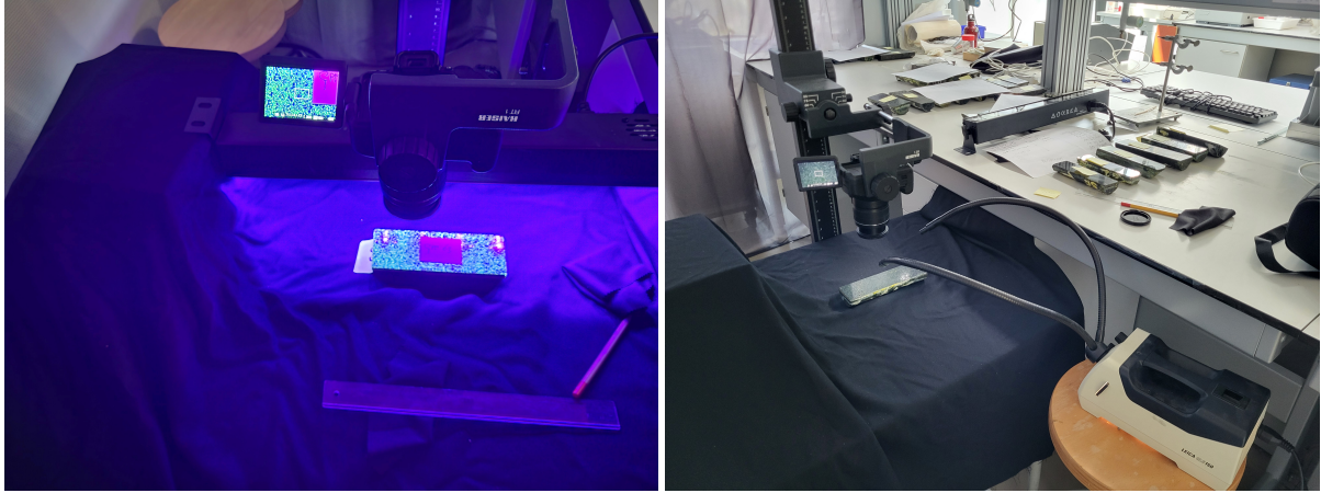
Figure 2.2: The setup with the UV light (left) and with the spotlight (right).
