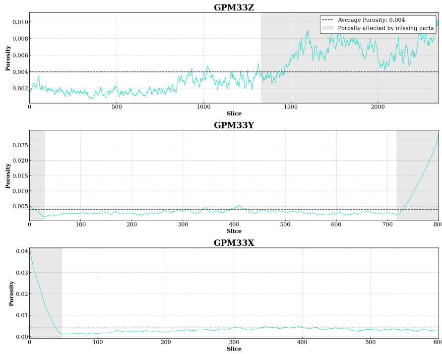
Figure 3.18: The porosity of 2D slices from CT-scanning of GPM33.
