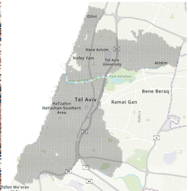
Fig 3: 4056 origin grid points spaced 126 meters apart. The points are the centroid of a hexagon for slightly more even distribution.
