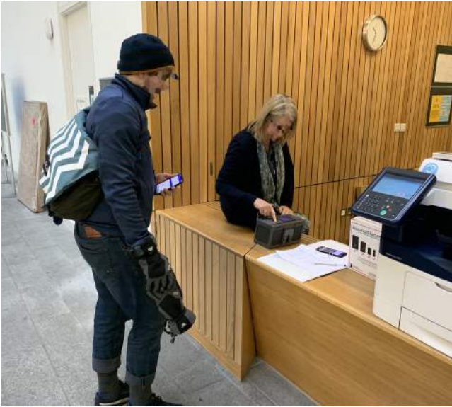
Figure 3: The receptionist pushes the button on the box to confirm she has received it, this action together with the colocation will unlock the box
