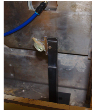
(b) Optical window located at the bottom of ST-15, (c) Adjustable mirror directing the laser sheet within the ST-15
