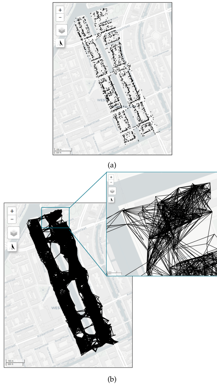
Figure 3.3.: Test area around the Bilderdijkgracht canal for experiment in Section 3.2. (a) Point scatterers inside the test area whose time series w.r.t. a common reference point (not shown) is taken for the conventional approach. (b) Arcs less than 60 meters taken for the dataset of local arcs.
