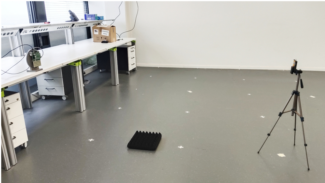
Figure A.1: Photograph of the measurement setup to investigate the effects of performing calibration in an echoic environment, taken in one of the Radar Labs of the Electrical Engineering, Mathematics and Computer Science (EEMCS) building. The DUT is placed on the edge of a table. Without the use of a specialized antenna platform, the measurement procedure relies on manual positioning of the HB100 module to implement the azimuth angles, \phi_{cal} . Moreover, a small panel of RF absorber can be seen on the floor halfway between the DUT and the beacon. This is done as an effort to suppress the scattered path due to the floor reflection.
