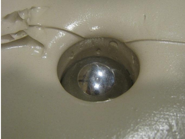
Figure 15.20: Particle penetration \Delta = 0.036 m ( D_s = 30 mm, \rho_s = 7821 kg/m 3 , v_{imp} = 2.0 m/s)
