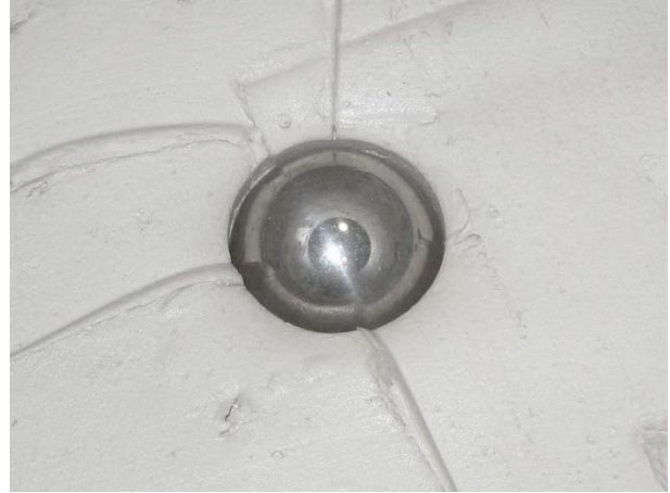
Figure 15.26: Particle penetration \Delta = 0.023 m ( D_s = 30 mm, \rho_s = 7821 kg/m 3 , v_{imp} = 3.0 m/s)
