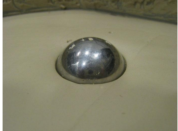
Figure 15.33: Particle penetration \Delta = 0.023 m ( D_s = 30 mm, \rho_s = 7821 kg/m 3 , v_{imp} = 5.0 m/s)
