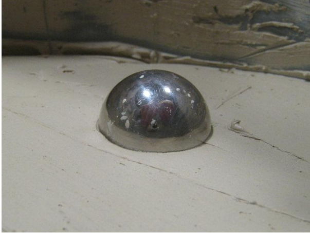
Figure 15.25: Particle penetration \Delta = 0.015 m ( D_s = 30 mm, \rho_s = 7821 kg/m 3 , v_{imp} = 2.0 m/s)
