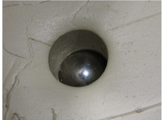
Figure 15.28: Particle penetration \Delta = 0.055 m ( D_s = 30 mm, \rho_s = 7821 kg/m 3 , v_{imp} = 5.0 m/s)
