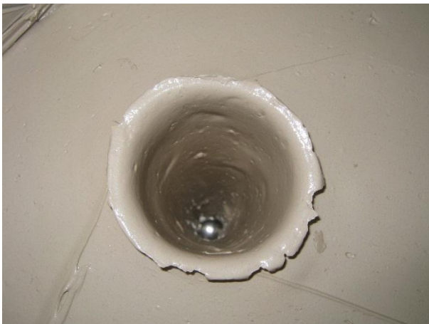
Figure 15.24: Particle penetration \Delta = 0.180 m ( D_s = 30 mm, \rho_s = 7821 kg/m 3 , v_{imp} = 6.0 m/s)
