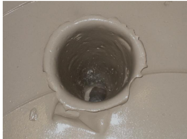
Figure 15.23: Particle penetration \Delta = 0.144 m ( D_s = 30 mm, \rho_s = 7821 kg/m 3 , v_{imp} = 5.0 m/s)
