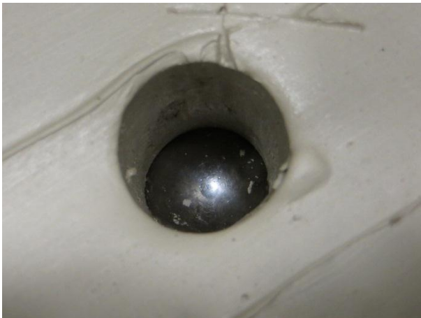
Figure 15.29: Particle penetration \Delta = 0.075 m ( D_s = 30 mm, \rho_s = 7821 kg/m 3 , v_{imp} = 6.0 m/s)
