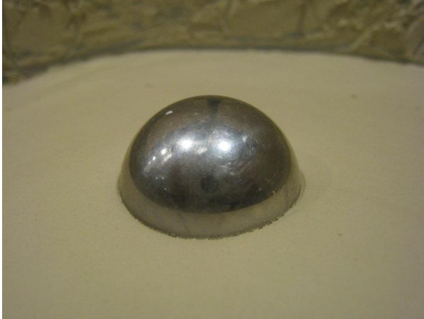
Figure 15.32: Particle penetration \Delta = 0.018 m ( D_s = 30 mm, \rho_s = 7821 kg/m 3 , v_{imp} = 4.0 m/s)
