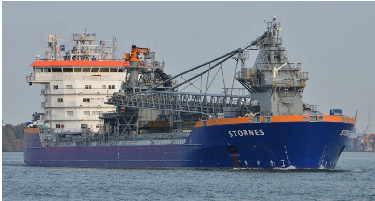
Figure 15.3: Flexible fallpipe vessel Stornes
