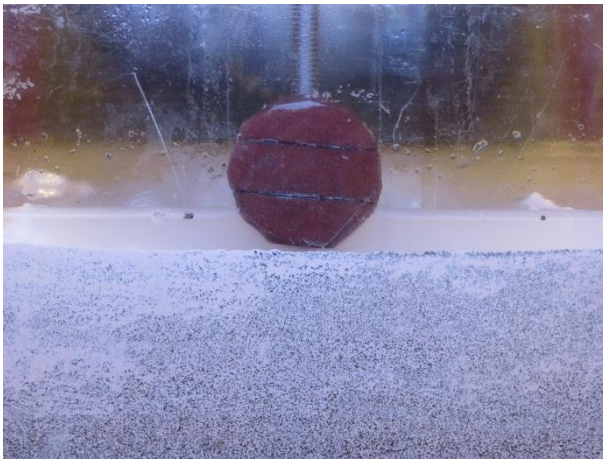
Figure 15.44: Slow penetration into normally consolidated clay with contrast material
