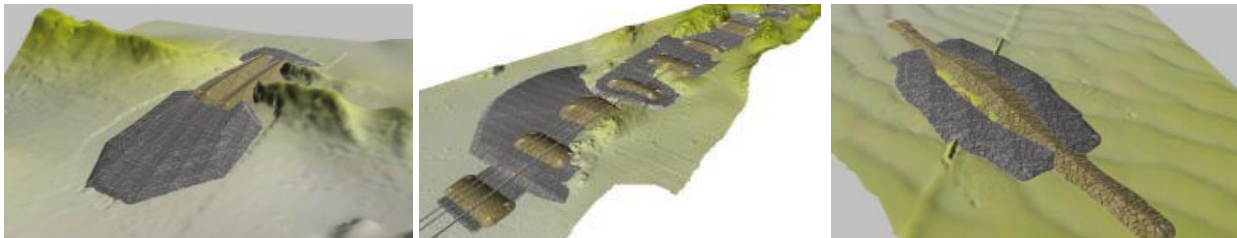
(a) The basic design of supports (brown) and counter fills (grey) (b) Free span mitigation supports (brown) including counter fills (grey) (c) Support for a pipeline crossing (brown) and counter fill (grey)
