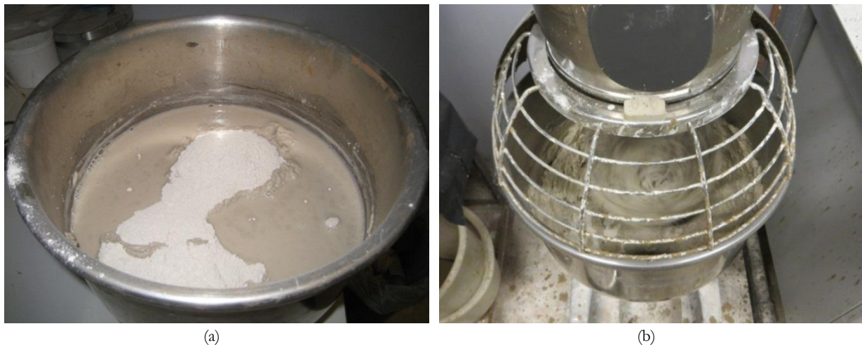
Figure 6.2: Kaolin water mixing process
