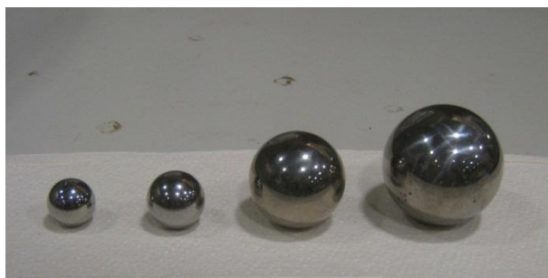
Figure 15.18: Steel bearings in different sizes ranging from 15 mm to 38 mm diameter
