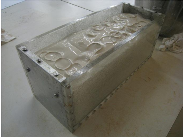
Figure 15.37: Fully saturated kaolin clay sample
