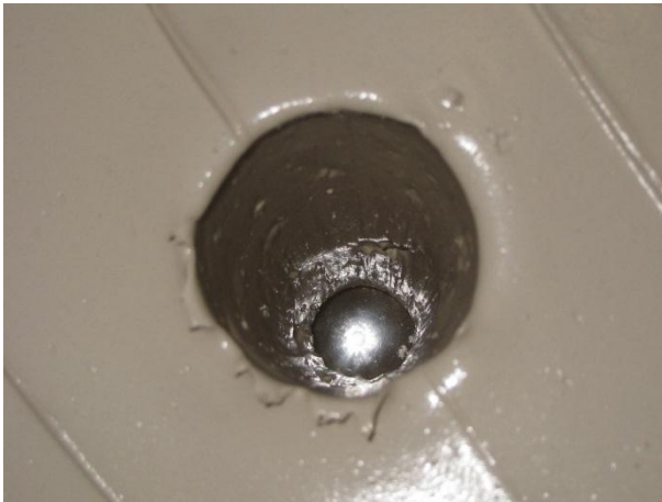
Figure 15.22: Particle penetration \Delta = 0.107 m ( D_s = 30 mm, \rho_s = 7821 kg/m 3 , v_{imp} = 4.0 m/s)
