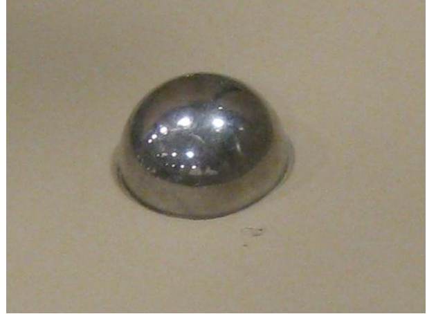
Figure 15.31: Particle penetration \Delta = 0.014 m ( D_s = 30 mm, \rho_s = 7821 kg/m 3 , v_{imp} = 3.0 m/s)
