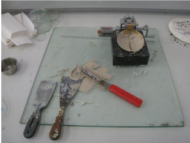
Figure 15.12: Atterberg limit determination using the Casagrande cup
