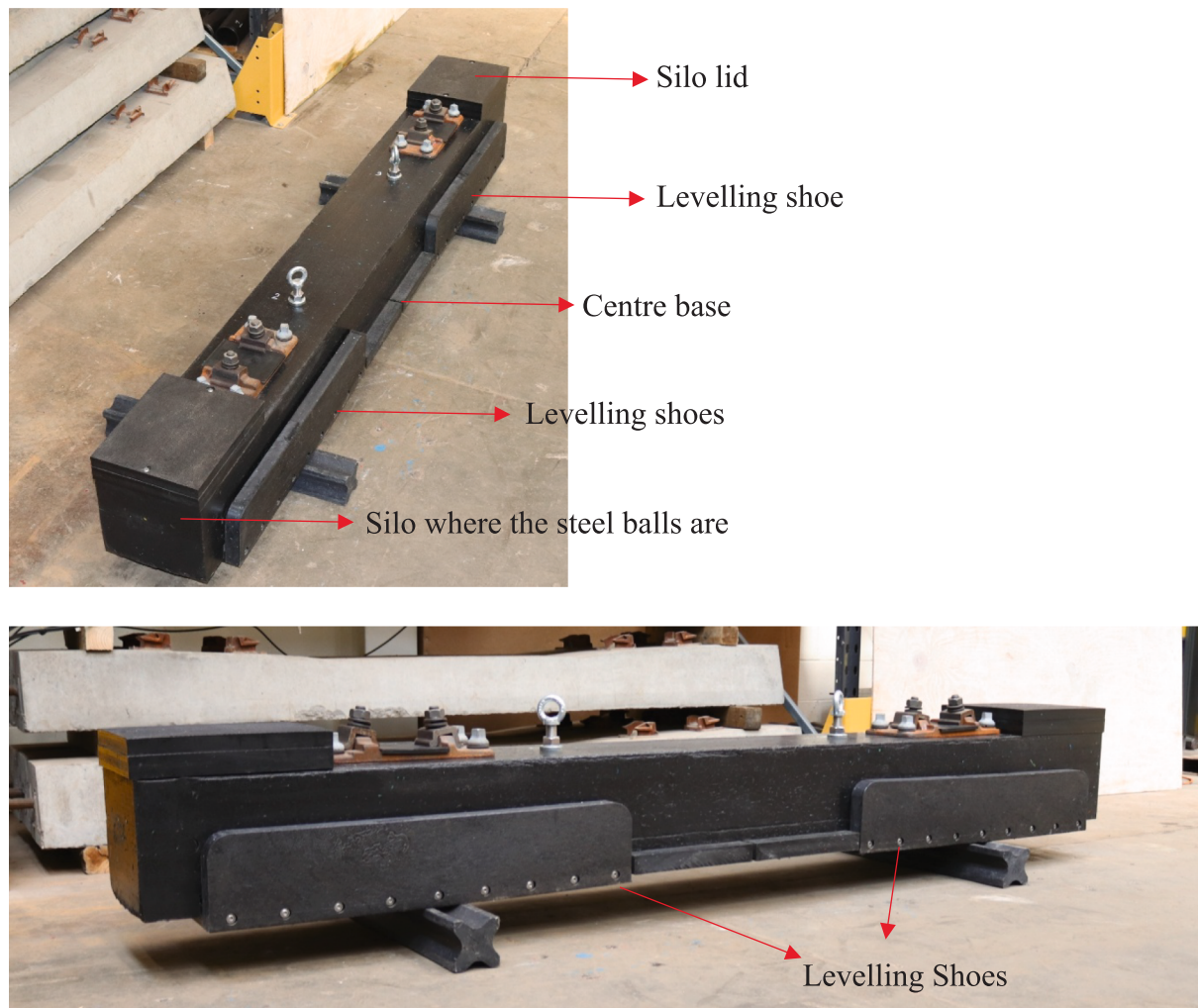
Fig. 15. Full-scale prototype of self-levelling sleeper – granular principle (SLS-G) .
