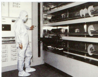
Fig.9. Ovenbelader in cleanroom
