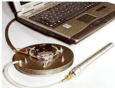
Fig. 14. Lap top met fuel cell (Bron: Fraunhofer Inst.)
