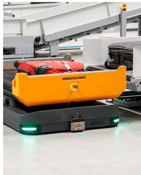
Figure 2.2: A FLEET AGV with a small conveyor on top to deliver and retrieve bags to/from a fixed conveyor [2].
