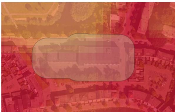
Figure 5.7: Heat stress is modeled through the use of a urban heat island layer. The average increase in temperature for the buffered area is used to construct  $r_G$ .
