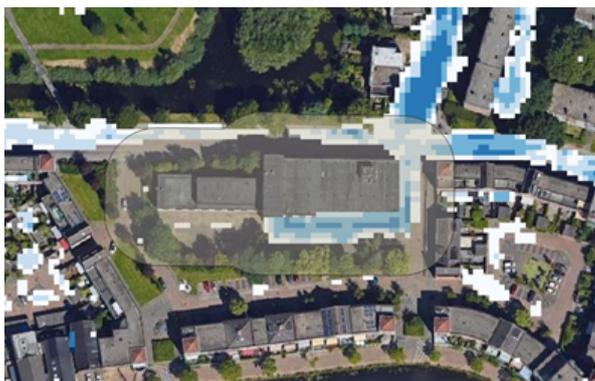
Figure 5.5: Water level during heavy rainfall event. The volume of water found in the building buffer is used to construct  $r_B$ .
