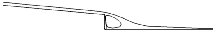
Figure 3.8: Several pathlines of the flow in the trailing edge region, for Re = 3 \times 10^5
