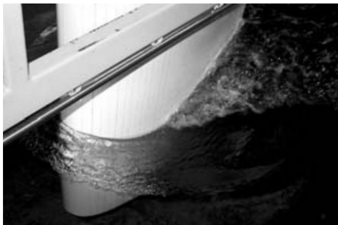
Figure 3.11: The experimental setup of the surface piercing foil. From Ref. [34] (flipped horizontal)
