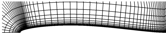
Figure 3.4: Detail of the NACA 63-010 grid
