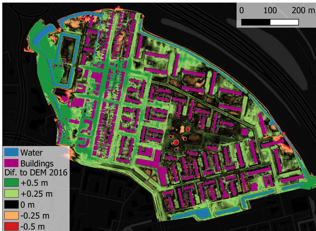
Figure 5.7: Created DEM of Tuinenhoven at design level compared to the DEM 2016. Note that green represents locations where the design DEM is higher than the 2016 DEM
