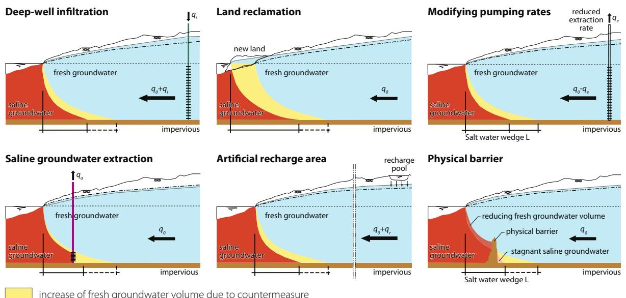
Figure 17.15. Concepts of countermeasures to control landward salt water intrusion (reprinted from Oude Essink, 2001a with permission from Elsevier). ↵
