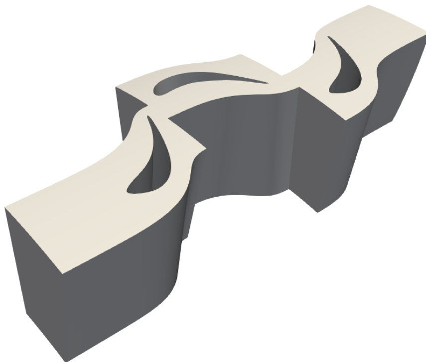
Figure 5.1: Aachen turbine flow domain
