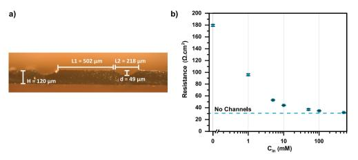
Figure 4.7: (a) Optical micrograph of ImPPO layer with channels in hydrated state. For the experiments, a thin ImPPO layer was attached (not shown) to cover the top side of the channels. (b) Ionic resistance of the membrane vs the concentration of KHCO<sub>3</sub> in the microchannels ( $C_{in}$ ). The concentration outside of the membrane was 0.1M KHCO<sub>3</sub> at either side.
