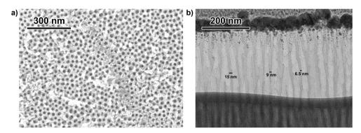
Figure 2.4: a) A SEM image of the AAO membrane surface shows a 10-nm pore at 120,000× magnification. b) A TEM image shows a cross-section of the same membrane at 150,000× magnification; nanopore morphology can be observed in the light gray area in the middle portion of the figure.
