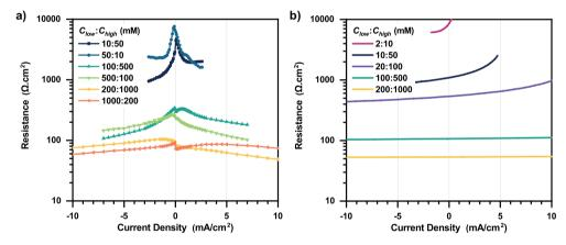
Figure 3.5: a) Ionic Resistance of 10 nm pore sized AAO membranes when placed between two compartments with different concentrations the two sides, a  $C_{high}$ : $C_{low}$  ratio of 5. The membranes were also inverted to account for non- idealities in the pore geometry. b) Simulated ionic resistance, with porosity as a fitting parameter.
