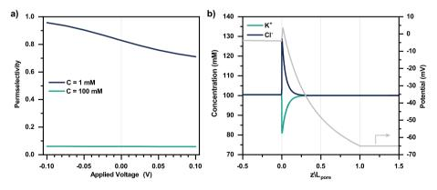
Figure S3.6: a) Permselectivity of conical nanopore with 8 nm of  $D_{p,1}$  and 50 nm of  $D_{p,2}$ , 50  $\mu$ m in length with a 40 mV  $\zeta$ -potential. Electrolyte concentration displayed in legend. b) Average ion concentration and potential (secondary axis) within a conical nanochannel with 8 nm of  $D_{p,1}$  and 20 nm of  $D_{p,2}$ , 50  $\mu$ m in length with a 40mV  $\zeta$ -potential, at approximately -5 mA/cm<sup>2</sup>. Pore placed between two compartments with 100 mM solution.
