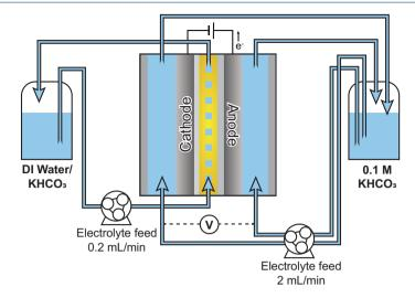
Figure S4.4: Schematic of the membrane resistance measurement. The AEM with internal microchannels (yellow) is between the anode and the cathode. KHCO3 solutions of varying concentrations were introduced into the left electrolyte reservoir, and a 0.1 M KHCO3 solution was introduced into the right reservoir.
