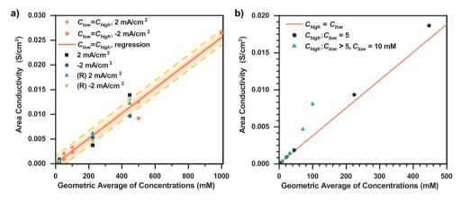
Figure 3.6: a) Ionic Resistance of 10 nm pore sized AAO membranes when placed between two compartments with different concentrations the two sides, a  $C_{high}$ : $C_{low}$  ratio of 5. The membranes were also inverted to account for non- idealities in the pore geometry. b) Simulated ionic resistance, with porosity as a fitting parameter.
