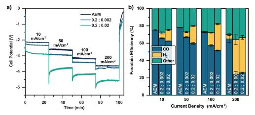
Figure 5.11:  $CO_2$  electrolysis experiments performed with a non-modified AEM, the 0.2;0.002 and 0.2;0.02 TFCMs in a zero-gap configuration. a) cell potential, with the different current densities indicated, b) FEs.
