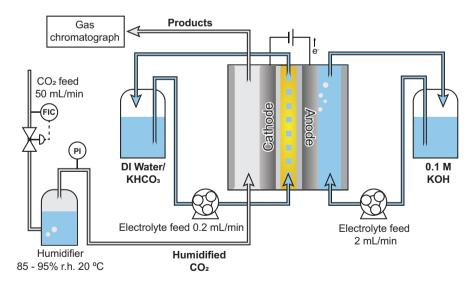
Figure S4.5: Schematic of the electrolysis setup. The AEM with internal microchannels (yellow) is between the anode and the cathode. During electrolysis, KHCO3 solutions of varying concentrations were introduced via the left electrolyte reservoir into the microchannels.
