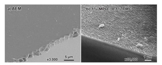
Figure 5.7: SEM images at a 45  $^{\circ}$  angle of a) a non-modified AEM and b) a TFCM made with 1  $^{\circ}$  MPD and 0.1  $^{\circ}$  w/v TMC. The magnification and the scale are indicated on the legends.
