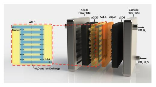
Figure 4.1: Schematic representation of an MEA cell for CO2RR that employs a bilayer AEM with internal channels to manage water fluxes. Inset (red box): Cross-section depicting internal water channels in the AEM.
