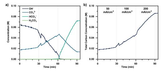
Figure S5.7: a) concentrations of  $OH^-$  and the different carbonate speciation species calculated based on the pH of the anolyte, b) calculated total carbon over time in the anolyte.
