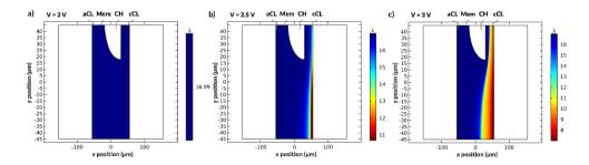
Figure S4.9: Water content distribution in the bilayer AEM with a curved internal channel with channel spacing of  $H = 90 \mu m$  for (a) 2 V, (b) 2.5 V (c) 3 V applied potentials. Note that the figures have different scales.
