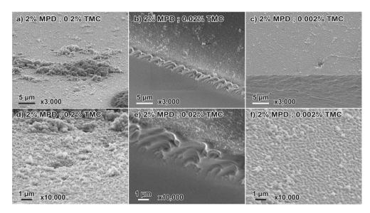
Figure 5.9: SEM images at a  $45^{\circ}$  angle of of TFCMs made with 2 w/v% MPD and: a) and d) 0.2 w/v% TMC; b) and e) 0.02 w/v TMC; c) and f) 0.002 w/v% TMC. Figures a-c) are at  $3,000 \times$  magnification, while figures d-f) show a zoom-in at  $10,000 \times$  magnification.
