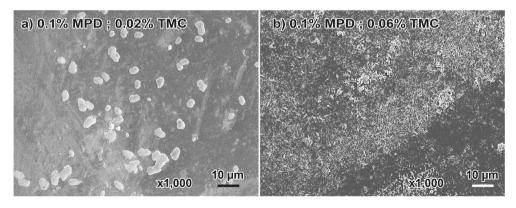
Figure 5.8: Top view SEM images at 1000 times magnification, of TFCMs made with 0.1 w/v% MPD and a) 0.02 w/v% TMC, and b) 0.06 w/v% TMC.
