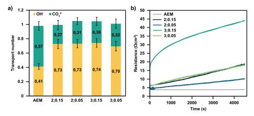
Figure 5.5: a) transport numbers of  $OH^-$  and  $CO_3{}^{2-}$  ions resulting from crossover experiments. The *x*-axis shows the monomer concentration with which the TFCM was fabricated, in MPD; TMC format, in w/v%. b) ionic resistance during the crossover experiments, with the legend indicating the monomer concentrations.
