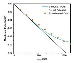
Figure S2.10: Membrane potential data fit with the ITM software, using a constant surface charge density of 0.074  $\rm C/m^2$ .
