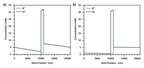
Figure S3.3: Concentration profiles for Cl<sup>-</sup> and K<sup>+</sup> along the center of the geometry (symmetry axis).  $L_p=1000$  nm,  $V_{applied}=0.1$  V. a) for  $C_{high}=C_{low}=5$  mM, b)  $C_{low}=1$  mM,  $C_{high}=5$  mM
