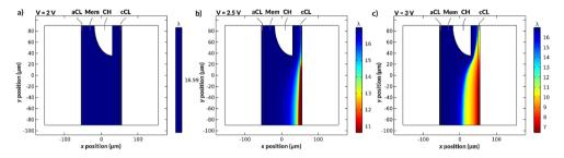
Figure S4.8: Water content distribution in the bilayer AEM with a curved internal channel with channel spacing of  $H = 180 \,\mu\text{m}$  for (a) 2 V, (b) 2.5 V (c) 3 V applied potentials. Note that the figures have different scales. Note that the figures have different scales.
