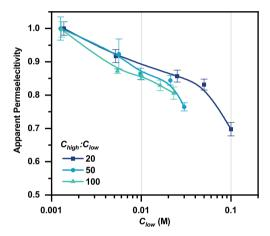
Figure S2.6: Apparent permselectivity results showcasing the effect of concentration and concentration ratio on permselectivity of the 10 nm pore sized AAO membrane, plotted against  $C_{low}$ . See vs  $C_{high}$  on Figure 2.3b.
