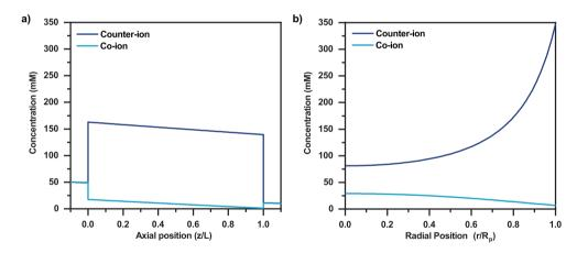
Figure 2.6: 5 Ion concentration profiles inside a pore with a 7-nm diameter (effective  $R_p=3$  nm) and a 1- $\mu$ m length are shown placed between two reservoirs with 10 mM and 50 mM of KCl. a) Longitudinal ion concentration profiles are shown with averaged concentration at each z position. b) Radial ion concentration profiles are shown at z/L=0.5, where 0 is the center of the pore and 1 is the pore wall.
