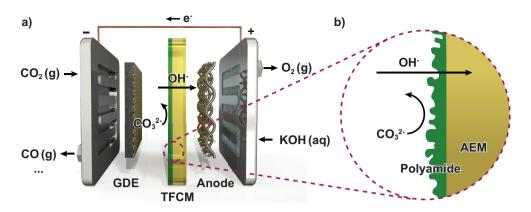
Figure 5.1: a) schematic illustration of a  $CO_2$  electrolyzer employing a TFCM. b) zoom-in into the TFCM, showing its two comprising layers.
