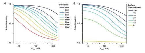
Figure S2.15: a) different pore sizes (shown in legend) vs  $C_{high}$  with 40 mV surface potential b) pore size of 7 nm but at different potentials (shown in legend) vs  $C_{high}$ .
