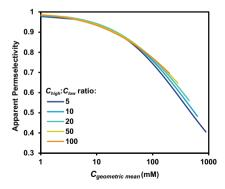
Figure S2.16: Different  $C_{high}$ :  $C_{low}$  ratios plotted vs the geometric mean of  $C_{high}$  and  $C_{low}$ .
