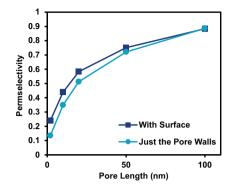
Figure S2.14: Simulated effect of presence of surface potential on the entire membrane vs pore length.
