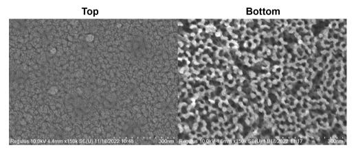
Figure S2.8: SEM pictures of the two different sides of an AAO membrane, as delivered.
