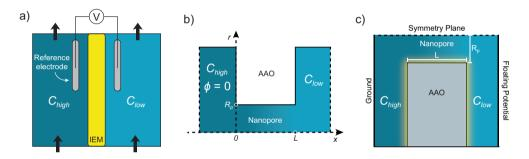
Figure 2.2: a) A schematic shows the permselectivity setup. b) The geometry modeled in the ITM software. c) The geometry modeled in COMSOL Multiphysics.
