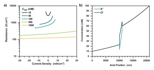
Figure S3.4: a) simulation of the real AAO nanopore, with 0.09 % porosity, 50  $\mu$ m pore length, 8 nm pore size and with fixed  $C_{low}$  at 10 mM.  $C_{high}$  varied (legend). b) concentration profiles in the entire geometry at 0.1 V and  $C_{high}$  = 100 mM
