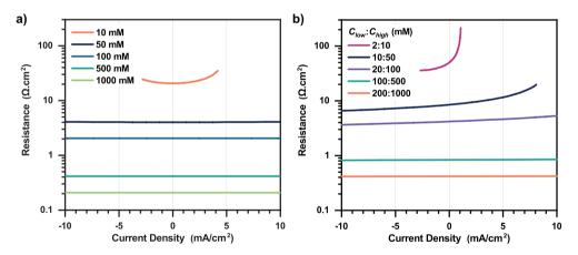
Figure S3.2: Simulation of 50  $\mu m$  long pore, with 40 mV of surface charge, and 12 % porosity at different electrolyte concentrations.
