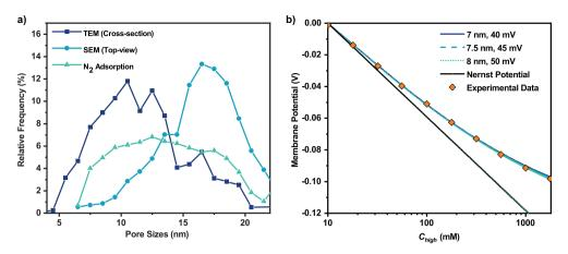
Figure 2.5: a) Pore size distributions are shown. b) Membrane potential data is fit with the ITM software. The three lines have a combination of pore sizes of 7, 7.5, and 8 nm and 40, 45, and 50 mV of  $\zeta$  potential.
