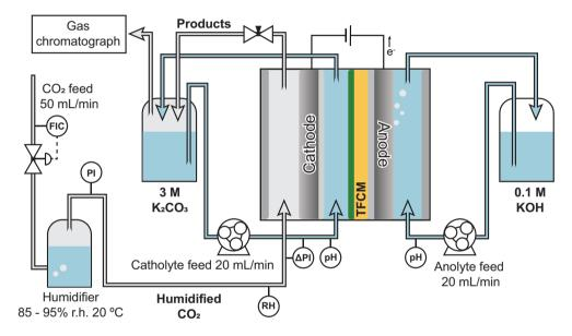
Figure 5.4: Schematic of the  $CO_2$  electrolysis setup.
