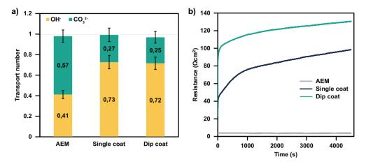
Figure 5.6: a) transport numbers of OH<sup>-</sup> and CO<sub>3</sub><sup>2-</sup> ions resulting from crossover experiments of dip-coated and single-coated TFCMs. b) ionic resistance during the crossover experiments, of non-modified AEMs, and single-coated and dip-coated TFCMs.
