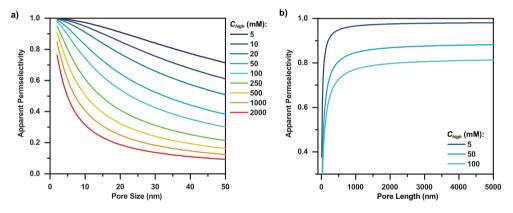
Figure 2.7: a) Effect of pore size vs. different concentrations is shown. b) Effect of pore length on apparent selectivity is shown.  $C_{high}$ : $C_{low}$  ratio is fixed at 5.
