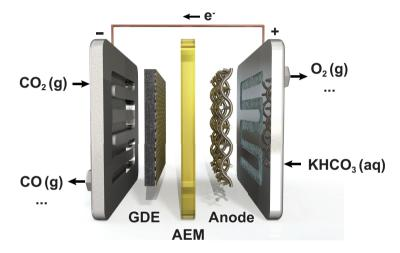
Figure 1.2: Schematic illustration of a typical laboratory scale CO<sub>2</sub> electrolyzer.
