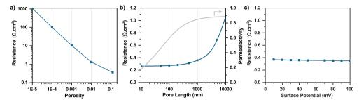
Figure 3.8: A pore of 1  $\mu$ m length, 12 % porosity 3.5 nm pore size, and with a 40 mV zeta potential was simulated between two compartments of 50 mM KCl. The figure shows the result of varying a) porosity, b) pore length and c) surface potential.
