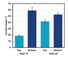
Figure S2.9: Contact angles of the two sides of AAO membranes with 10 nm and 20 nm pore sizes.
