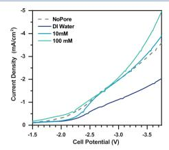
Figure S4.11: Galvanostatic linear sweep experiments with different electrolyate concentrations inside the membrane channels in full MEA configuration, with hydrated  $N_2$  gas as anolyte.
