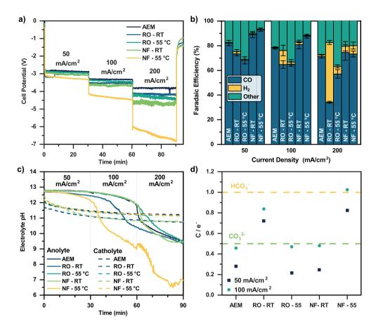
Figure 5.14:  $CO_2$  electrolysis experiments performed with a catholyte layer, displaying the result with a non-modified AEM, the RO and NF-based TFCMs cured at room temperature (marked as RT) and at 55 °C. a) cell potential, with the different current densities indicated, b) FEs, c) pH profiles of the anolyte (solid lines) and catholyte (dashed lines) during the experiment and d) the calculated carbon transport numbers per electron, for 50 and 100 mA/cm<sup>2</sup>.
