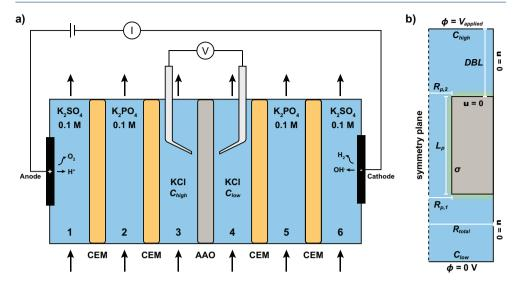
Figure 3.2: a) Schematic illustration of the 6-compartment setup used for electrical resistance measurements, b) geometry modelled in COMSOL Multiphysics
