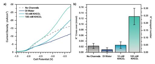
Figure 4.8: (a) galvanostatic linear sweep experiments with different electrolyte concentrations inside the AEM channels. (b) K+ crossover to the cathode side in function of the KHCO3 concentration inside the microchannels of the AEM.
