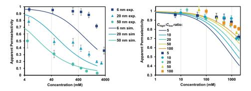
Figure S2.11: a) Comparison between pore size data and simulation. b) Comparison between concentration ratio data and simulations. Legend shows the  $C_{high}$ : $C_{low}$  ratio, with the lines corresponding to the simulation results and the markers corresponding to the experimental data.
