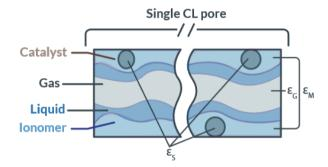
Figure S4.1: Schematic of a single pore within the porous catalyst layer in the electrochemical model. As simulated, the porous catalyst layer is assumed to be a homogeneous continuum of CL pores with volumes defined as shown above.
