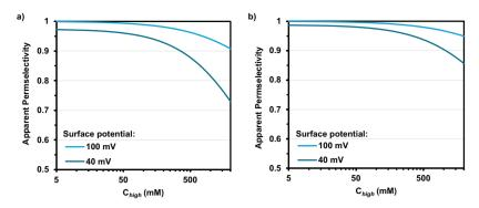
Figure S2.17: a)  $C_{high}$ : $C_{low}$  ratio = 5 b)  $C_{high}$ : $C_{low}$  ratio = 35 with different surface potentials. Pore size of 3 nm and pore length of 5  $\mu$ m.
