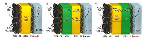
Figure 6.1: Schematic representation of cell configurations for electrochemical  $CO_2$  reduction at a gas diffusion electrode paired with oxygen evolution at the anode in a liquid analyte. The gas diffusion electrode consists of a gas diffusion layer (GDL) and a catalyst layer (CL). The three configurations highlighted here are: a) an (anion-exchange membrane-electrode assembly (AEMEA)), b) a BPM in reverse bias, and c) a bipolar membrane-electrode assembly (BPMEA) in forward bias.
