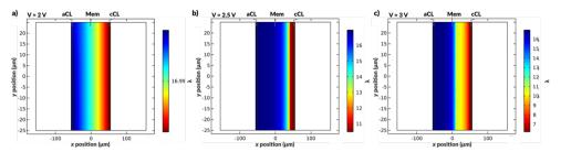
Figure S4.7: Water content distribution in the AEM with no internal microchannels for (a) 2 V, (b) 2.5 V (c) 3 V applied potentials. Note that the figures have different scales.
