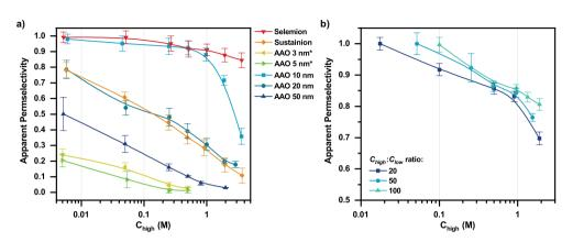
Figure 2.3: a) Apparent permselectivity of two polymeric IEMs – Selemion AMV and Sustainion X37 – and five AAO membranes with different pore sizes (3–50 nm) placed between two reservoirs with a concentration ratio of 5.\*3-nm and 5-nm pores are asymmetric membranes with only a thin selective layer. b) Apparent permselectivity results showcase the effect of concentration and concentration ratio on permselectivity of the AAO membrane with 10-nm pores. Note that the figures have different scales.
