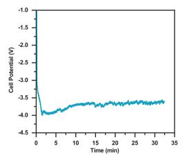
Figure S4.2: Electrolysis at 100 mA/cm<sup>2</sup>, in zero-gap configuration using a 32 μm thick ImPPO membrane
