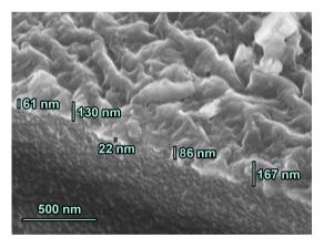
Figure S5.4: SEM image of an RO-based membrane cured at 55  $^{\circ}$ C. Image taken at 10,000 times magnification, at a 40degree angle.
