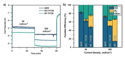
Figure 5.13:  $CO_2$  electrolysis experiments performed with a non-modified AEM, the RO and NF-based TFCMs in a zero-gap configuration. a) cell potential, with the different current densities indicated, b) FEs for different current densities.
