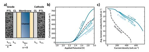
Figure 4.6: (a) Schematic of 1-D geometry modeled (channel thickness of  $50 \mu m$ ) to determine the impact of channel electrolyte concentration on cell performance. (b) Current-voltage characteristics of bilayer AEM cells with an internal channel with varying KHCO $_3$  concentration. (c) Average ionomer conductivity within the bilayer AEM with varying KHCO $_3$  concentration as a function of total cell current density.
