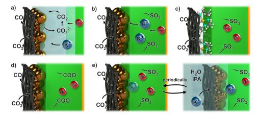
Figure 6.4: illustration of strategies to alleviate BPM-catalyst interaction: a) adding a catholyte layer, b) loading the CEL with  $K^+$ , c) employing  $CO_2R$  selective molecular catalysts, d) using CELs with weakly acidic groups or e) periodically injecting  $K^+$  from the back of the GDE.
