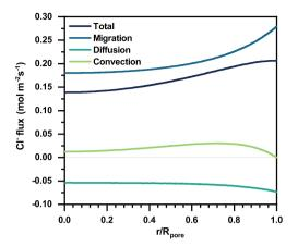
Figure S3.1: Simulations for an 8 nm in diameter and 50  $\mu$ m in length pore with a 40mV  $\zeta$ -potential at 0.05 V applied potential. The pore was placed between two compartments with 50 mM solution. Total flux, and flux contributions of migration, diffusion, and convection in the r-direction for Cl<sup>-</sup> ions. r = 0 shows the center of the pore, and at r = 1 is the pore wall. The fluxes are indicated in the middle of the pore, at  $z/L_{pore} = 0.5$
