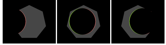
Figure 3: Example frames of a moving circle occluding a heptagonal aperture. Our progressive method can update the FT for the entire aperture by adding/subtracting only the FTs of newly discovered/occluded (green/red) quads to/from the previous calculation.
