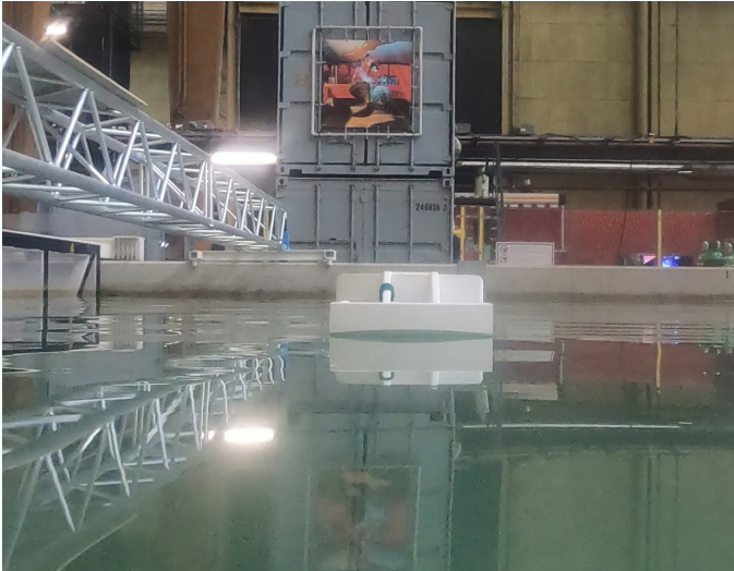
Figure 5.42: Test 1: Trimaran stable before waves
