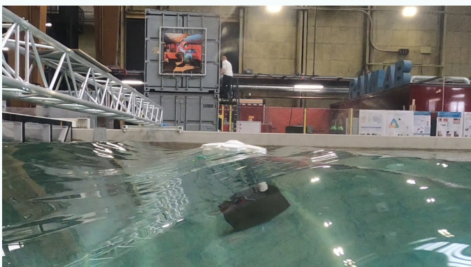
Figure 6.12 New system showing flexing in intense waves.
