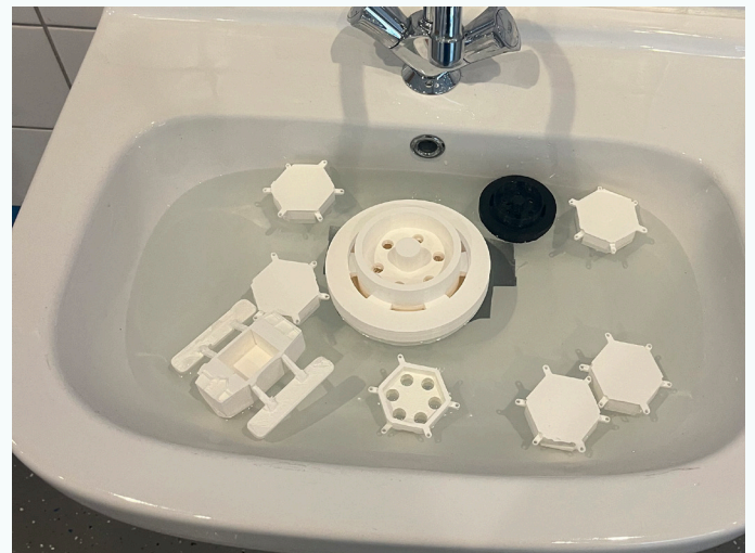
Figure 5.12: Every iteration went through a float test to get a basic idea of the performance.
