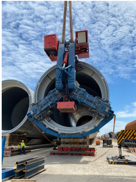
Figure 3.13: Monopile upending and lifting tool of SpanSet Axzion [76]
