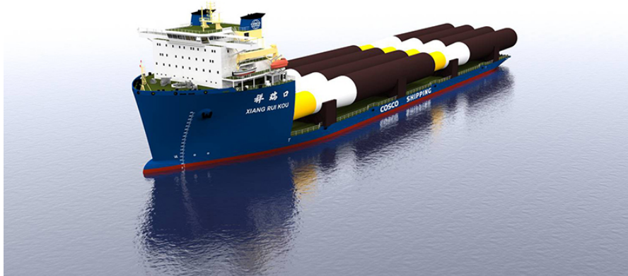
Figure 3.11: Transport vessel with longitudinal storage of monopiles [71]
