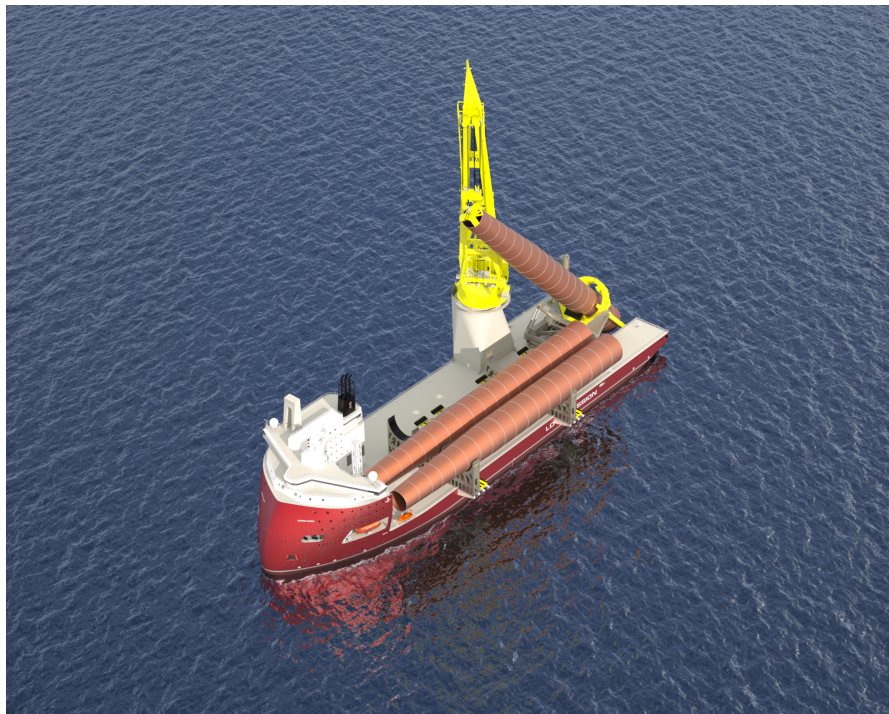
Figure 4.2: HX118 with Huisman TMC crane, upending a MP in the U-stern (Ulstein, 2023)
