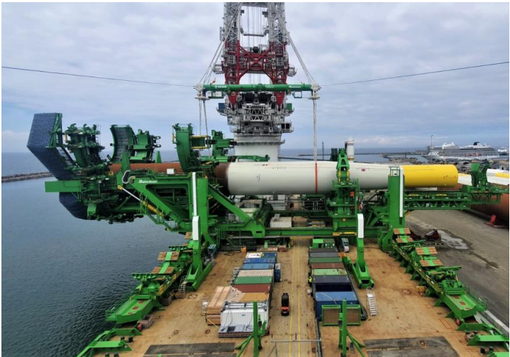
Figure 3.17: Motion compensated pile gripper [79]
