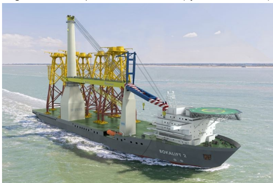
Figure 3.8: Heavy lift vessel: Bokalift 2 [66]
