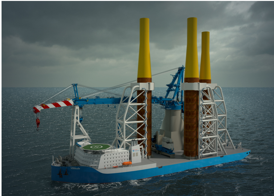
Figure 3.12: Concept design of a foundation installation vessel with vertical storage [72]
