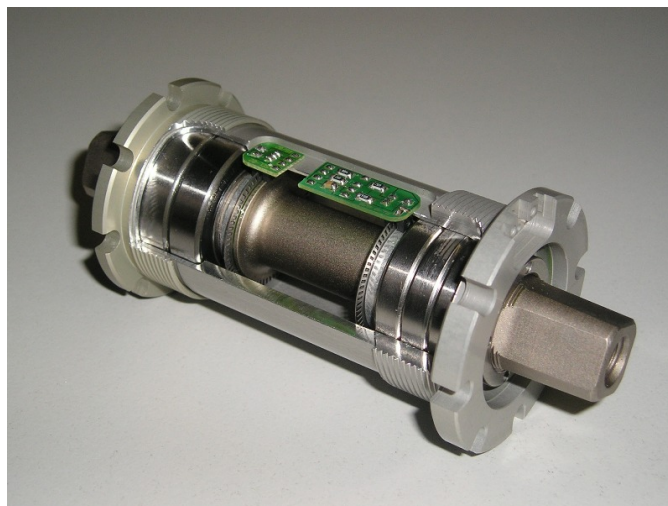
Figure 3.7: Ergomo bottom bracket sensor with slotted disks for optical measurement. [14]
