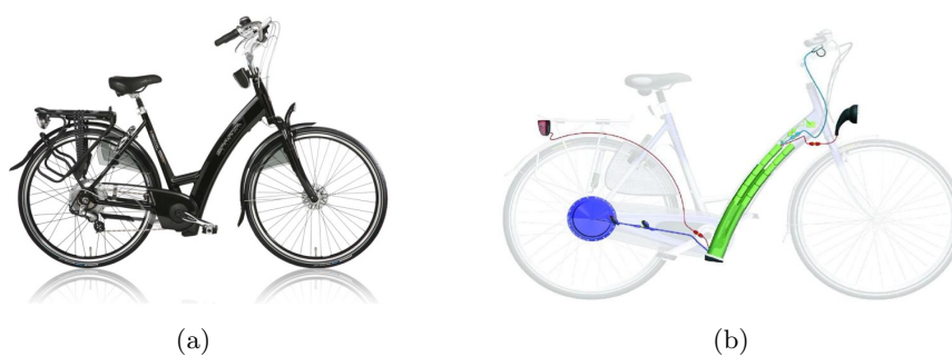
Figure 1.2: (a) Example of an e-bike with ION technology from Sparta [Sparta] (b) schematic view of the ION technology with a rear wheel hub motor and battery pack integrated into the frame. [5]
