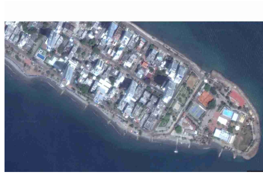
(b) Groynes fully sedimentated
