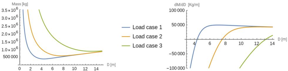
Figure 4.10: Mass vs. diameter (left) and first derivative(right) per load case.
