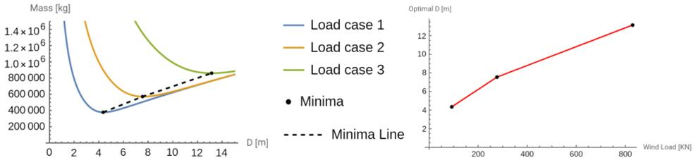
Figure 4.11: Line of the optima (left) and optimal diameter per load case (right).
