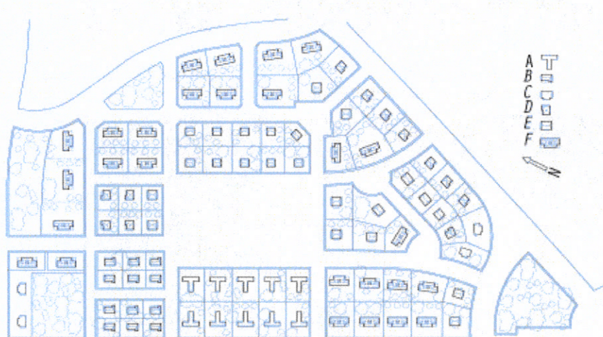
Figure 15: INCIS Technical Office's lot division plan of 1936 with plots of different residential typologies for the Italian residential area.
