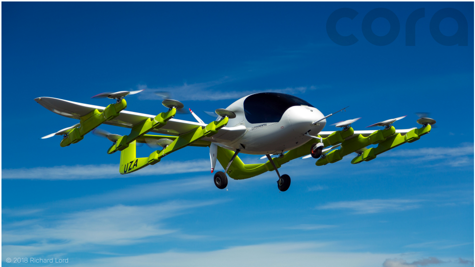
Figure 1.9: Test flight of the Cora eVTOL concept, equipped with 12 propellers for lift during vertical take-off and a pusher-propeller at the aft fuselage for thrust in forward flight. Photo courtesy of Cora Aero. © 2018 Richard Lord.
