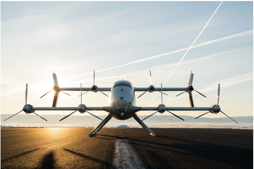
Figure 1.10: Front view of the Airbus A 3 Vahana eVTOL vehicle, using tiltwings with 8 propellers for lift during vertical take-off and thrust in forward flight. © 2019 A 3 by Airbus. All rights reserved.
