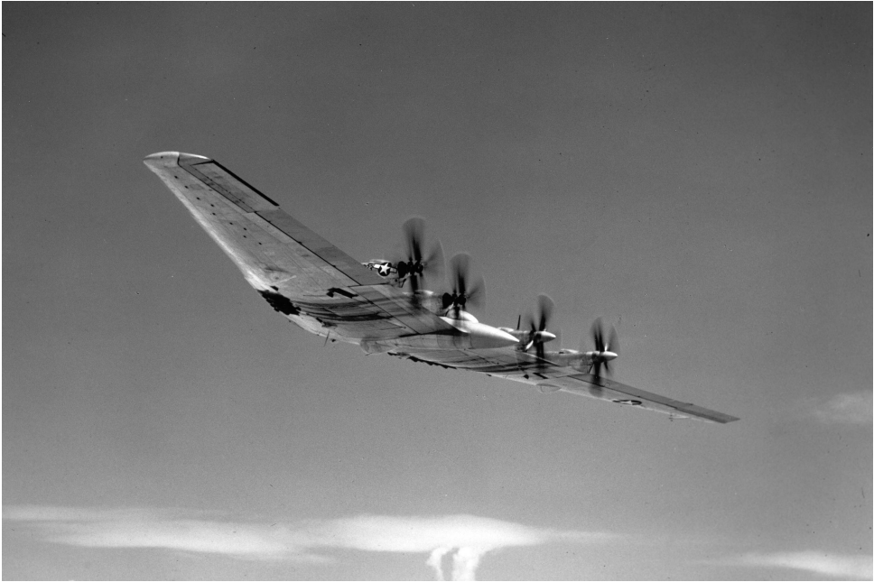
Figure 1.3: Northrop XB-35 flying wing, propelled by four wing-mounted contra-rotating propellers in pusher configuration. Credits: U.S. Air Force.
