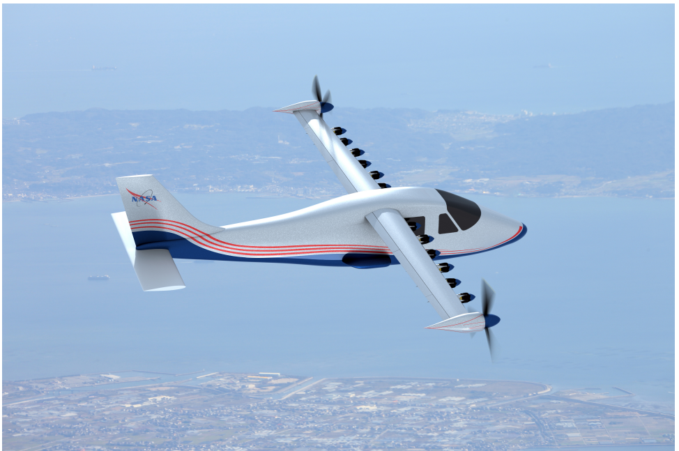
Figure 1.6: NASA X-57 Maxwell render, using wingtip-mounted tractor-propellers to improve cruise performance and distributed electric propulsion propellers to blow the wing during take-off and landing. Credits: NASA Langley/Advanced Concepts Lab, AMA, Inc.
