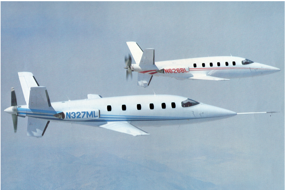
Figure 1.2: LearAvia Lear Fan 2100, following the principle of the XB-42 with a single propeller at the aft fuselage. © 2019 The Museum of Flight Foundation. All rights reserved.
