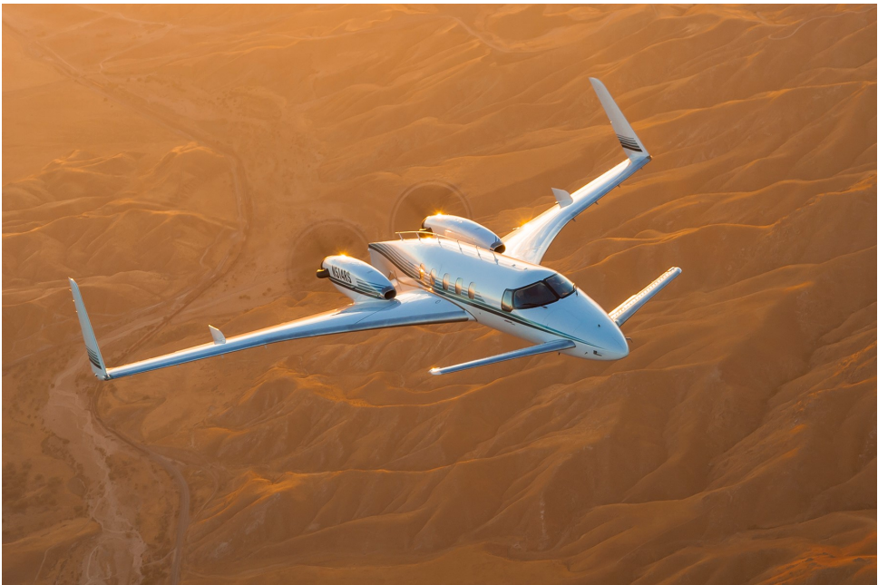
Figure 1.4: One of the few still flying Beech Starship, featuring two wing-mounted propellers in pusher configuration. © Chad Slattery. All Rights Reserved.
