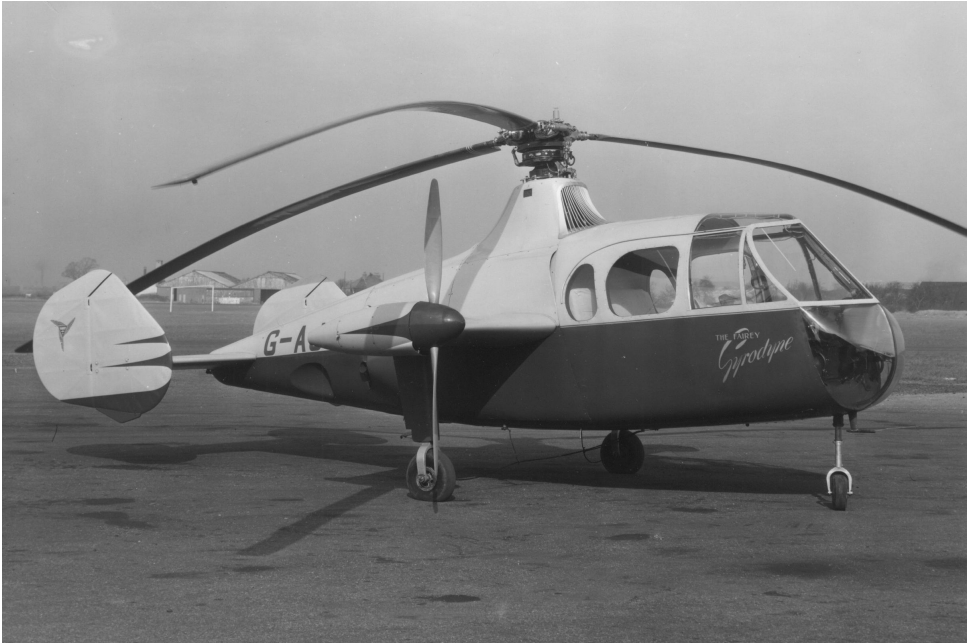
Figure 1.7: Fairey Gyrodyne, utilizing a single wingtip-mounted tractor-propeller to counter the main rotor torque and provide thrust. Credits: Ray Watkins Collection.
