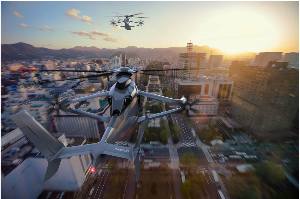
Figure 1.8: Render of the Airbus RACER compound helicopter, featuring a box-wing design for additional lift with two wingtip-mounted pusher-propellers or lateral rotors for thrust and counter torque. © Production Autrement Dit.
