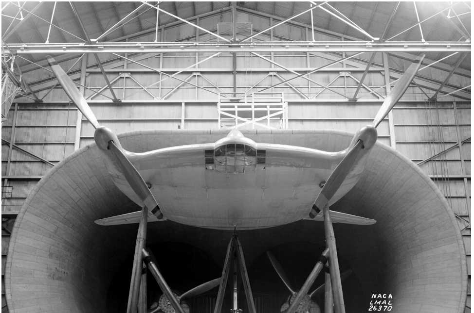
Figure 1.5: Vought V-173 in a wind-tunnel, a flying wing with wingtip-mounted tractor-propellers. Credits: NASA.
