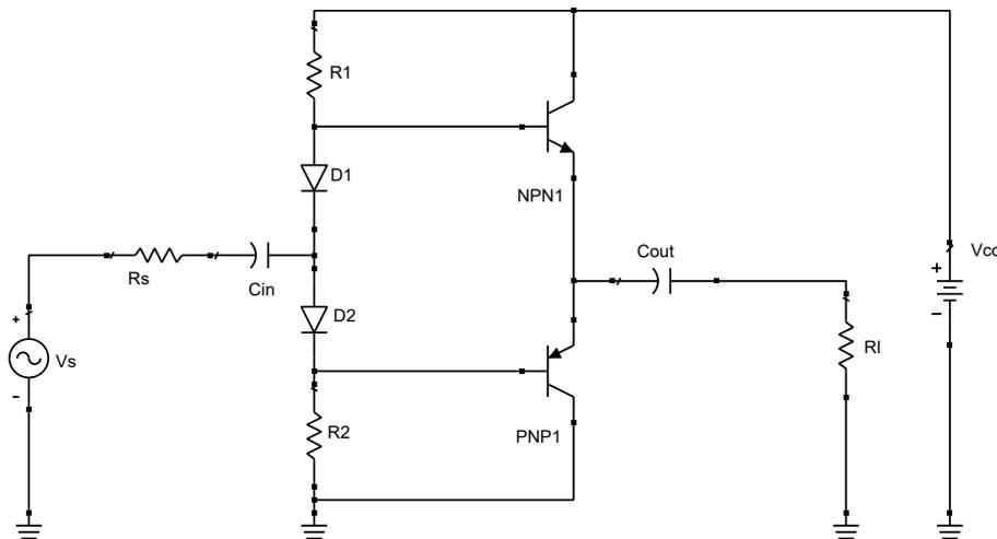
Figure 8.1: Topology of the class-AB amplifier with diode biasing
