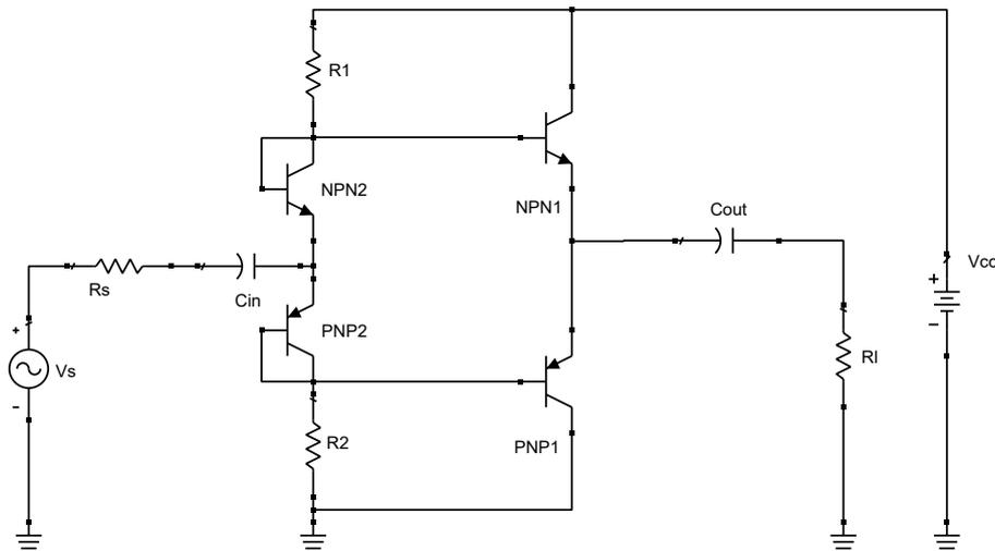
Figure 8.5: Topology of the class-AB amplifier with transistor biasing
