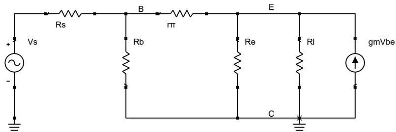
Figure 4.3: Circuit diagram used for small signal analysis of the voltage buffer.
