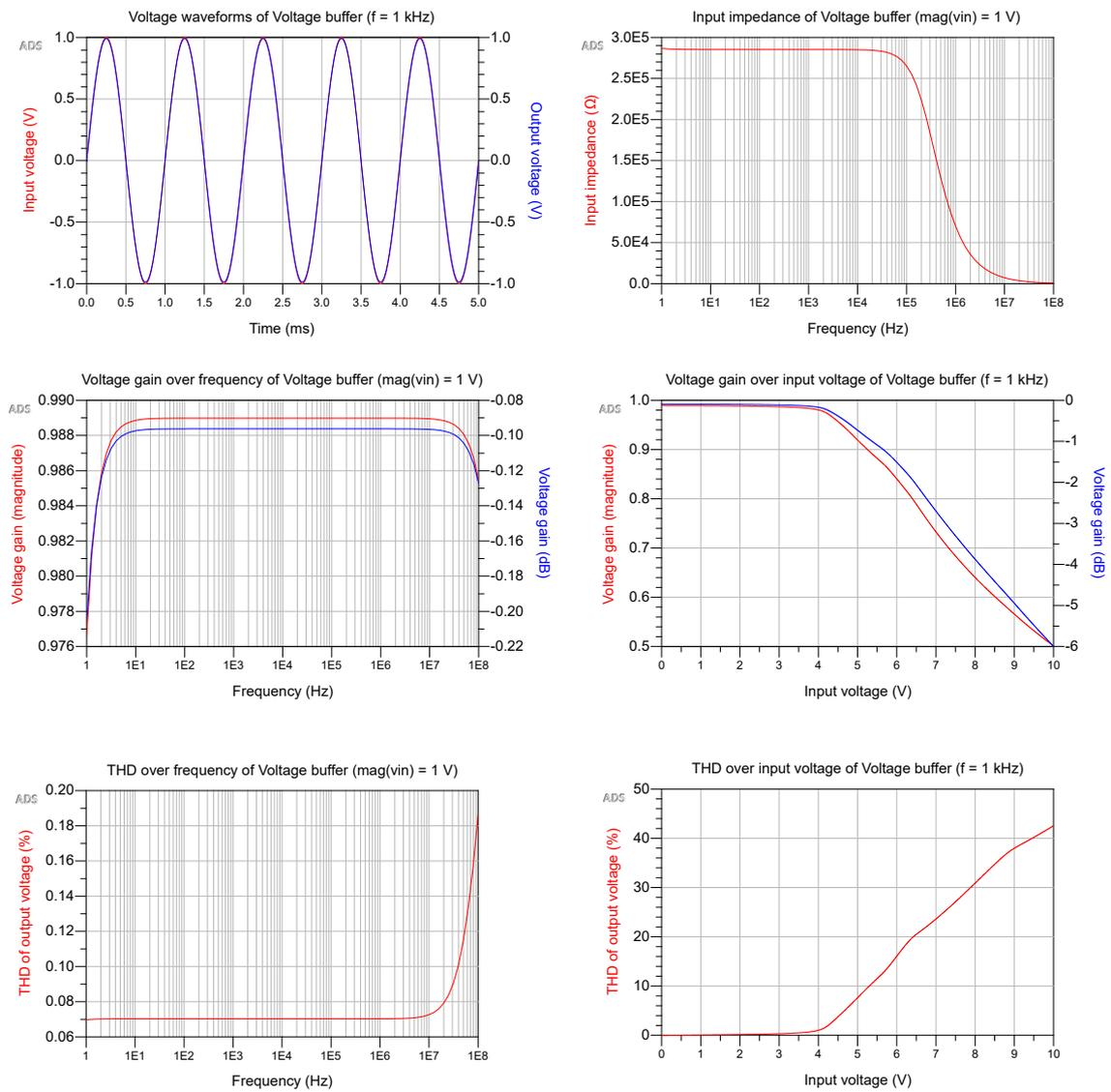
Figure 9.1: Simulation results of the Voltage buffer.
