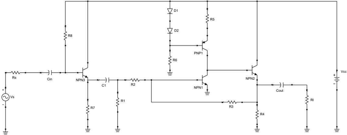
Figure 7.1: Circuit feedback amplifier with buffer
