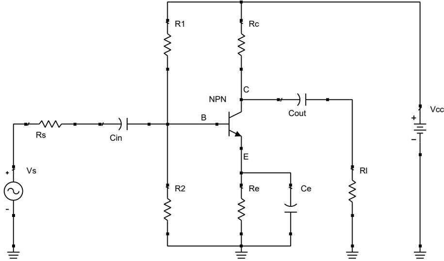
Figure 5.1: Circuit diagram of the microphone amplifier.
