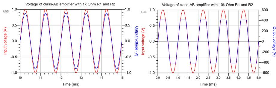
Figure 8.6: Voltage characteristics of the class-AB design
