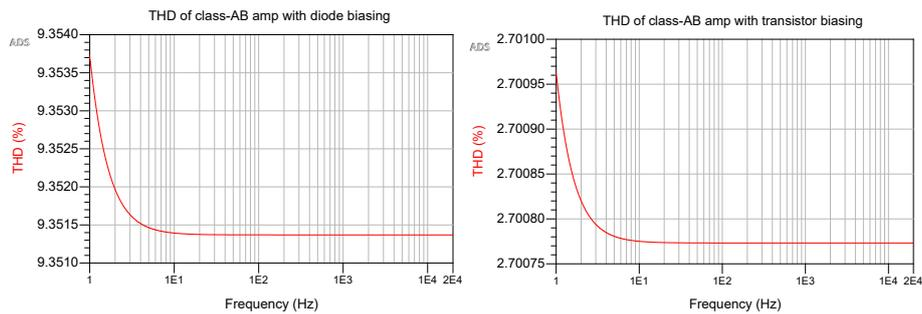
Figure 8.3: Total harmonic distortion of two class-AB designs
