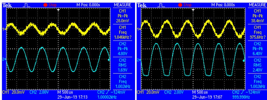
Figure 10.3: Input voltage (yellow) and output voltage (blue) during microphone amplifier voltage sweep (left 18 mV pk-pk input, right 30 mV pk-pk input)
