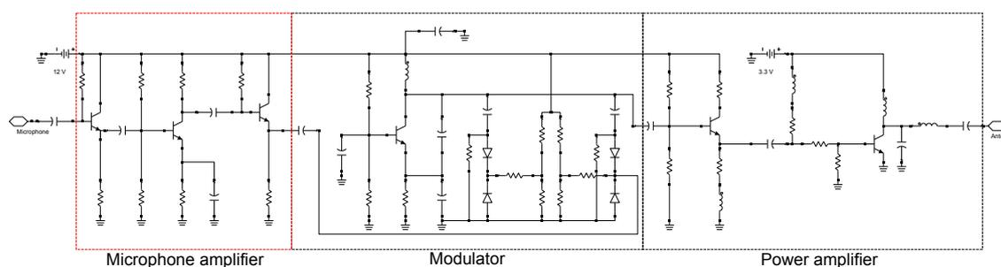
Figure 11.1: The final transmitter circuit
