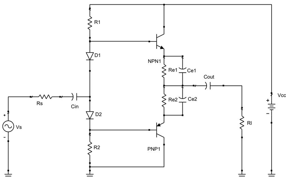
Figure 8.4: Topology of the class-AB amplifier with emitter resistance and capacitance
