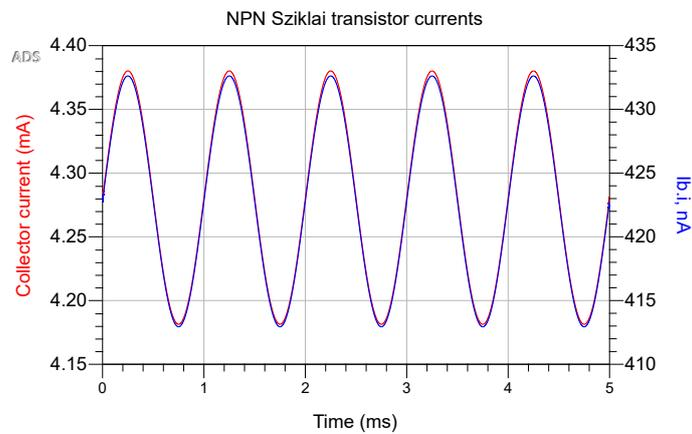
Figure 2.14: Typical currents of a NPN Sziklai transistor
