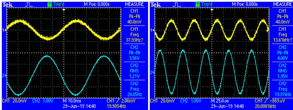
Figure 10.5: Bandwidth measurements for feedback amplifier prototype
