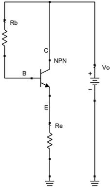
Figure 4.2: Circuit diagram used for large signal analysis of the voltage buffer.
