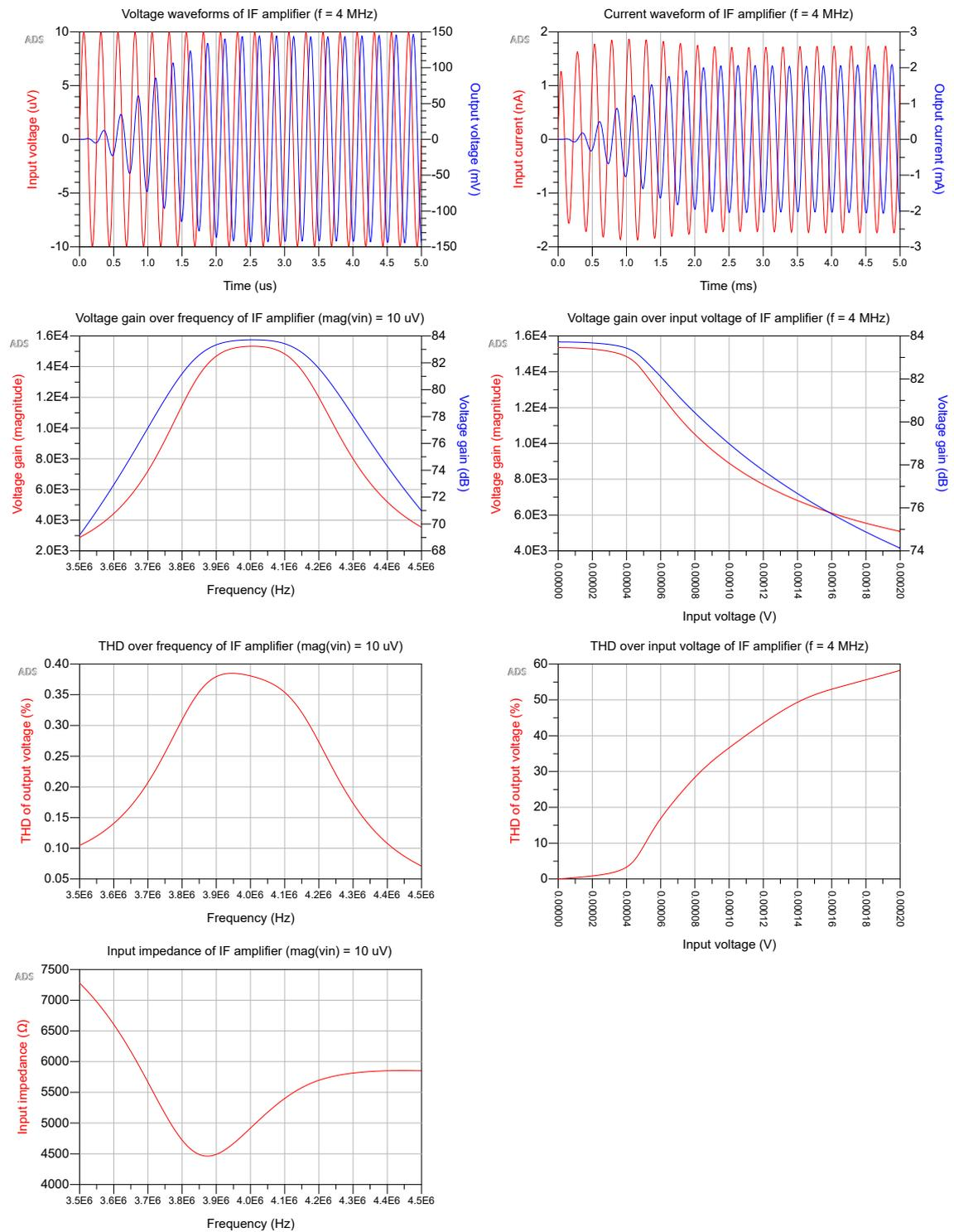
Figure 9.3: Simulations results of the IF amplifier.
