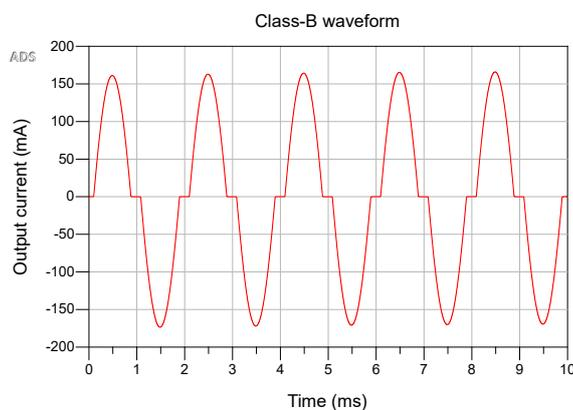
Figure 3.2: Class-B amplifier waveform
