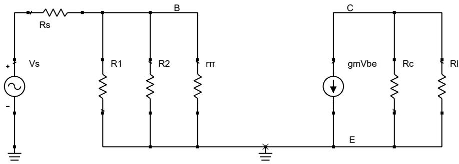
Figure 5.3: Circuit diagram used for small signal analysis of the microphone amplifier.
