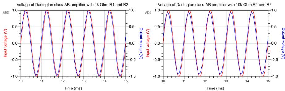
Figure 8.7: Voltage characteristics of the Darlington class-AB design
