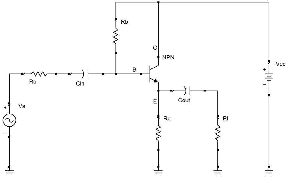
Figure 4.1: Circuit diagram of the voltage buffer.
