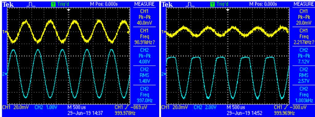
Figure 10.6: Gain measurements for feedback amplifier prototype
