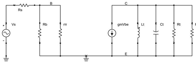
Figure 6.3: Circuit diagram used for small signal analysis of the bandpass amplifier.
