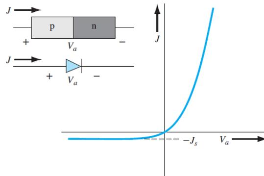
Figure 2.2: Ideal I-V characteristic of a PN junction diode. [4]
