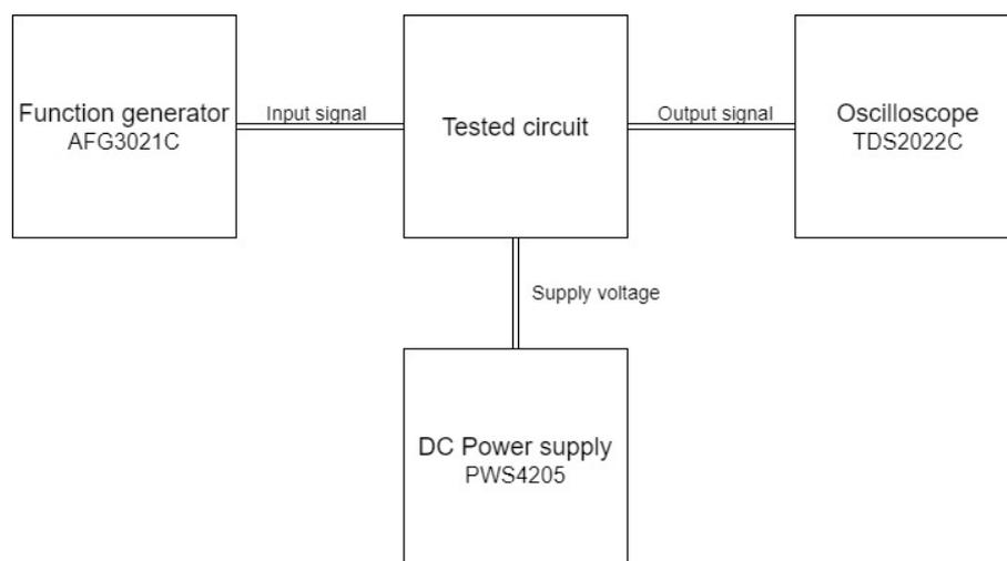
Figure 10.1: Setup for prototype testing
