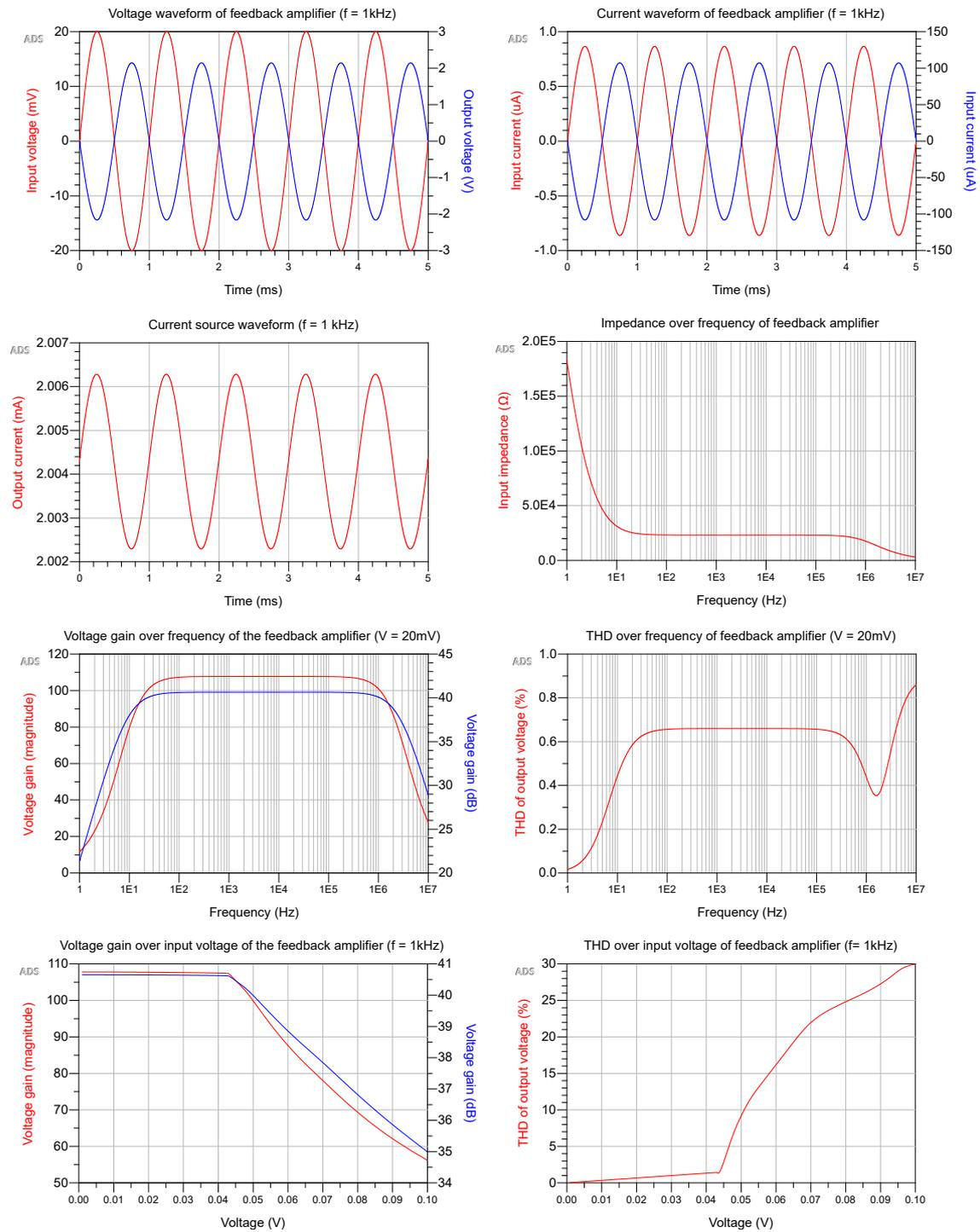
Figure 9.4: Simulations of the feedback amplifier
