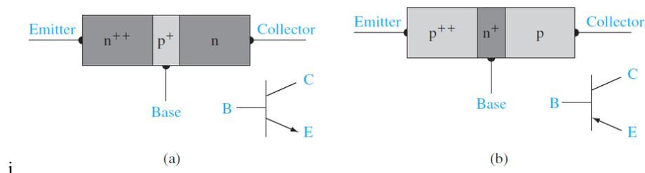
Figure 2.1: Block diagrams and circuit symbols of (a) NPN and (b) PNP bipolar transistors. [4]
