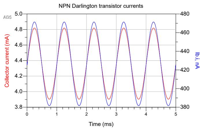
Figure 2.11: Typical currents of a NPN Darlington transistor
