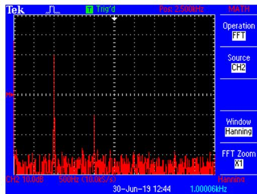
Figure 10.4: Fast Fourier Transform of output signal with 1 kHz input signal and pk-pk voltage of 10 mV
