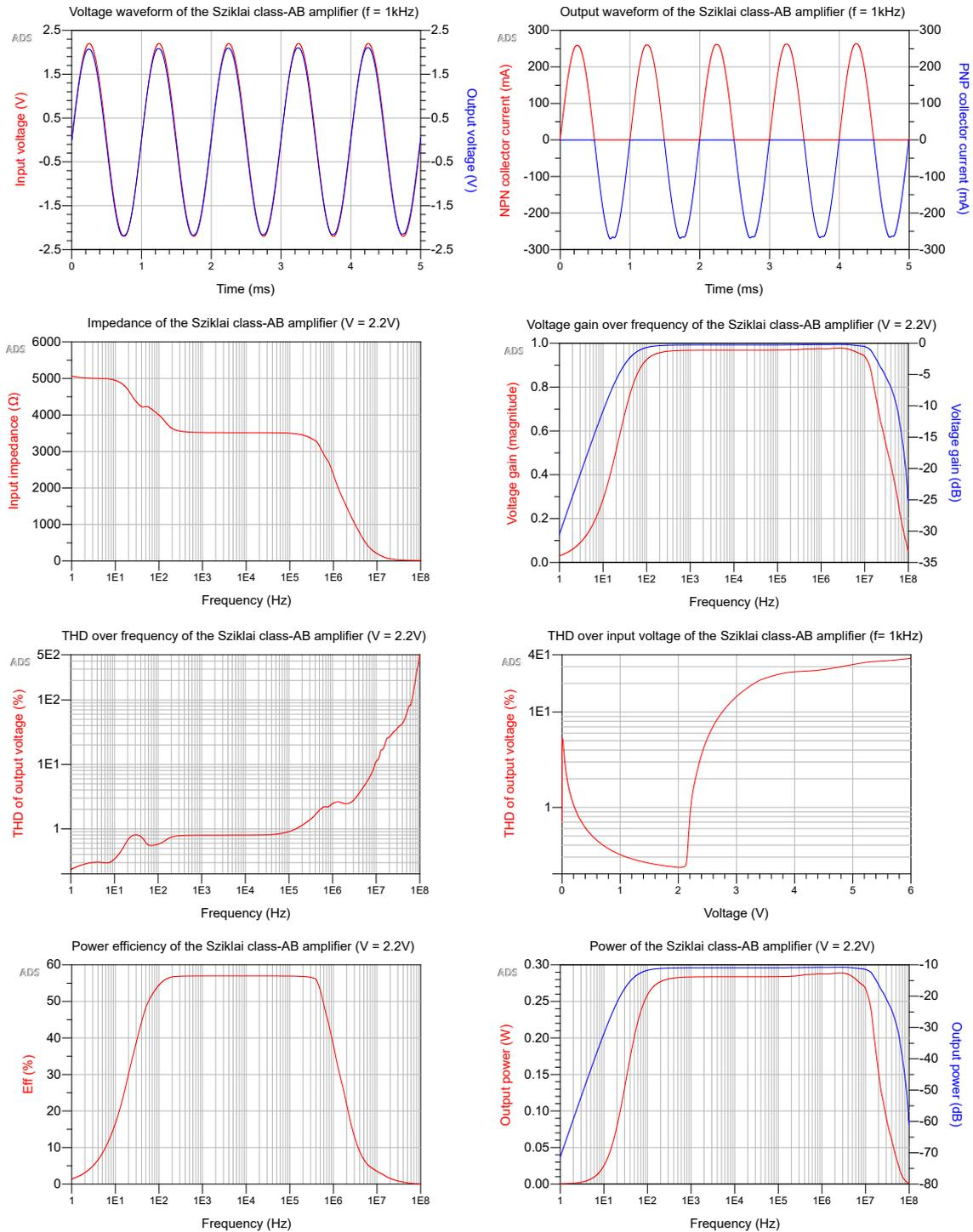
Figure 9.5: Simulations of the Sziklai class-AB amplifier
