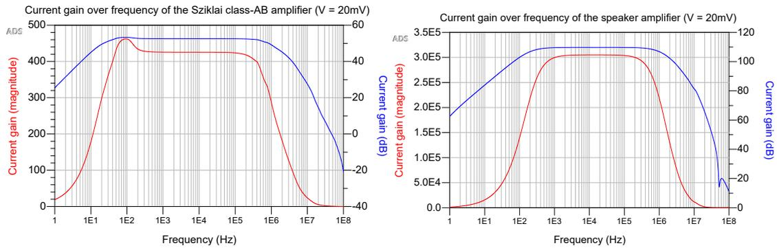
Figure 9.8: Current gain of the Sziklai class-AB and speaker amplifier
