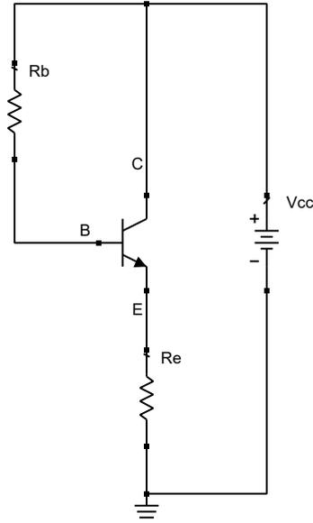
Figure 6.2: Circuit diagram used for large signal analysis of the bandpass amplifier.
