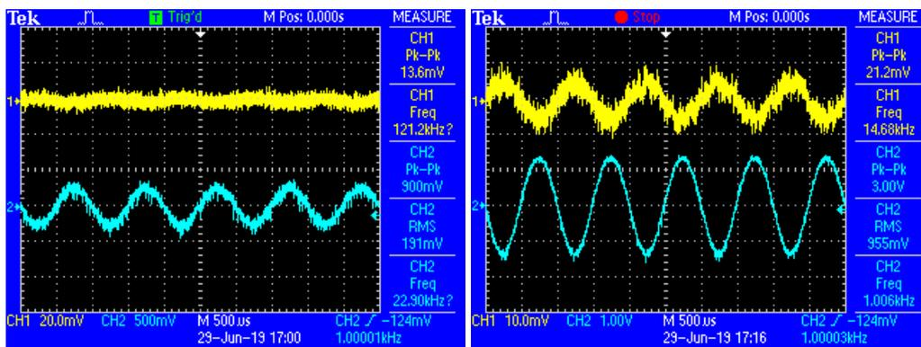
Figure 10.2: Input voltage (yellow) and output voltage (blue) during microphone amplifier voltage sweep (left 2 mV pk-pk input, right 10 mV pk-pk input)
