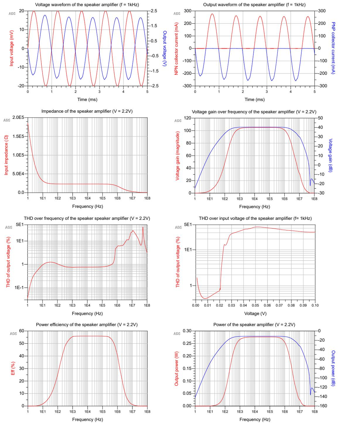
Figure 9.6: Simulations of the speaker amplifier
