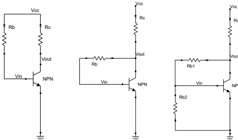
Figure 2.7: Fixed base (left), collector feedback (middle) and dual feedback (right) BJT biasing.
