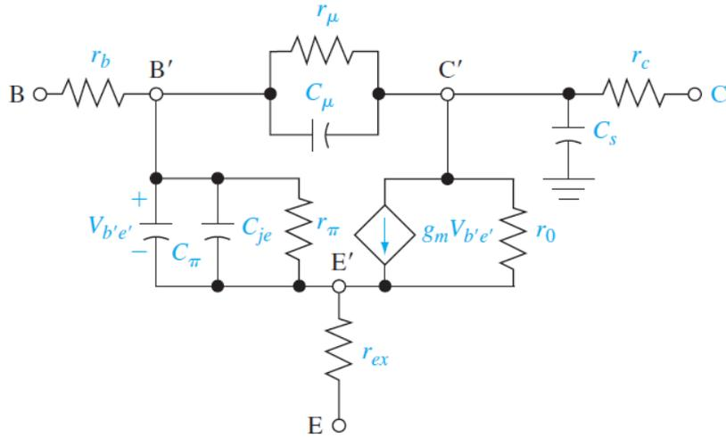
Figure 2.4: Hybrid-Pi equivalent circuit. [4]
