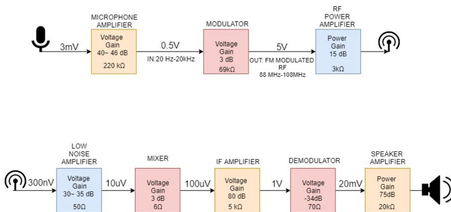
Figure 1.1: Block diagram of the transceiver system with signal levels, input impedances and gain indicated per block.
