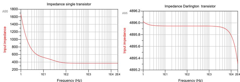
Figure 8.8: Input impedance of different topologies
