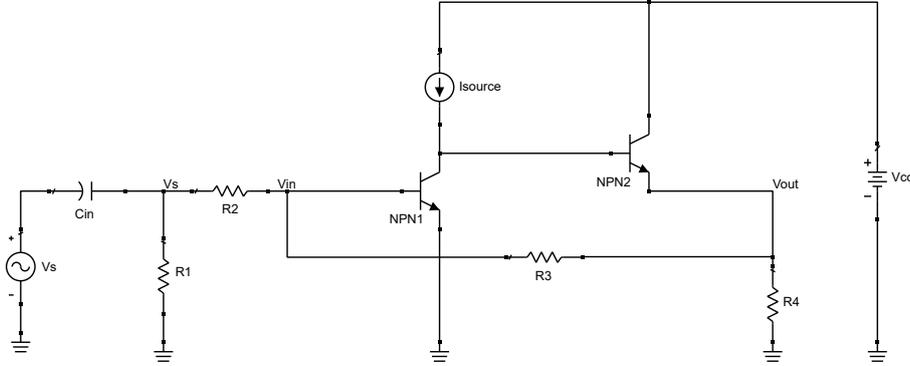
Figure 7.4: Simplified feedback amplifier circuit
