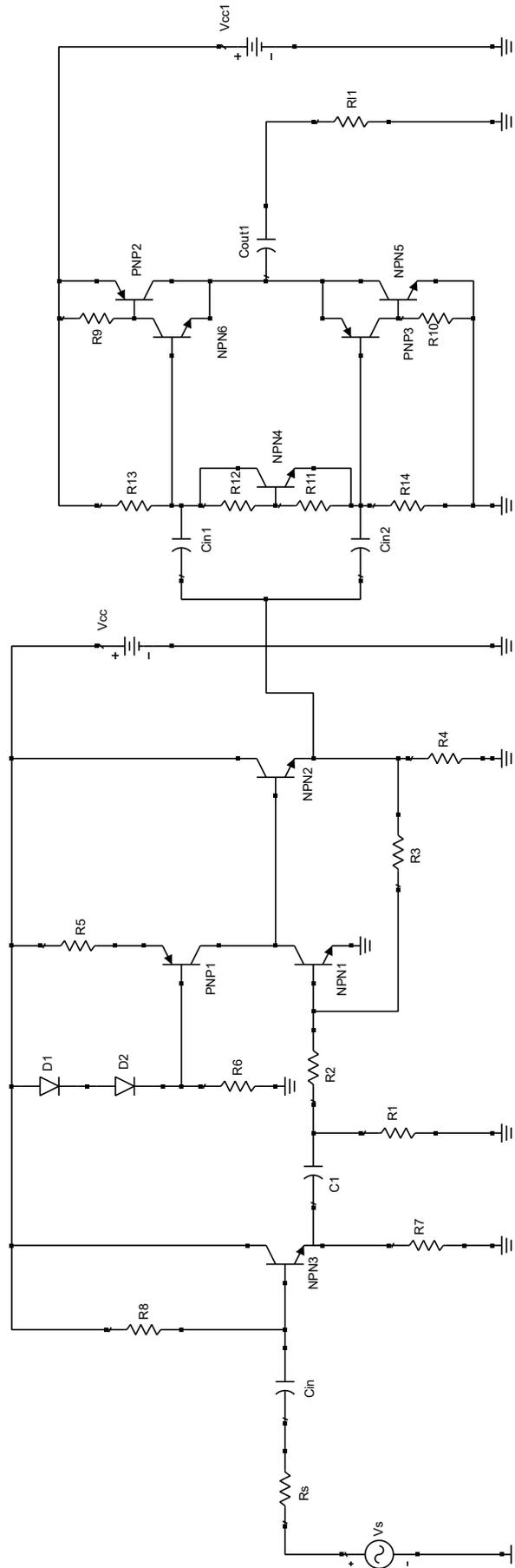
Figure 8.11: Topology of complete speaker amplifier
