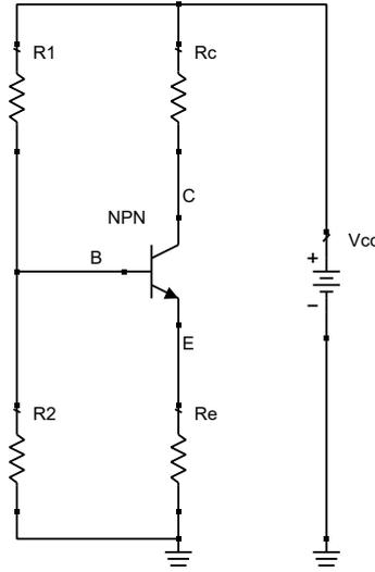
Figure 5.2: Circuit diagram used for large signal analysis of the microphone amplifier.
