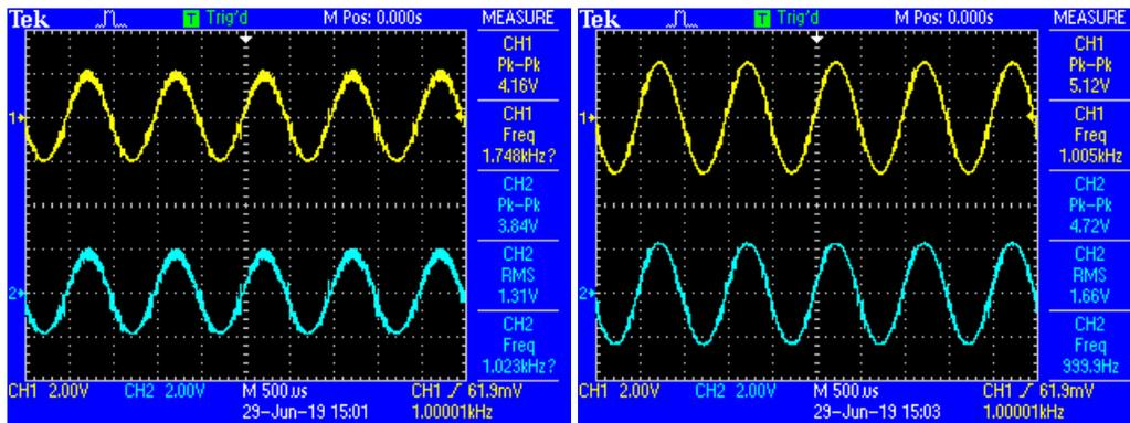
Figure 10.8: Gain measurements for class-AB amplifier prototype
