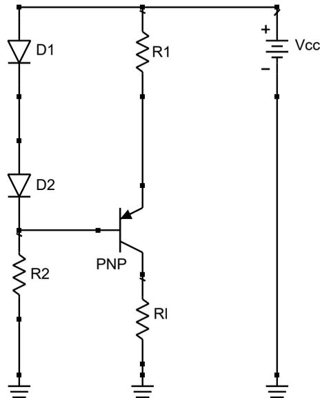
Figure 7.2: Circuit of the current source
