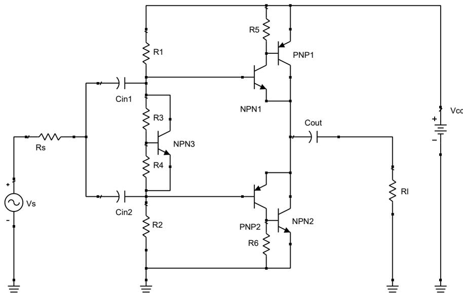
Figure 8.10: Topology of the Sziklai AB-Class amplifier
