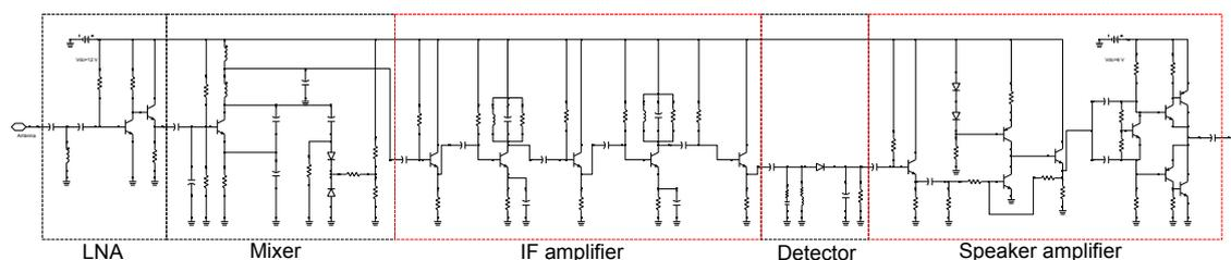
Figure 11.2: The final receiver circuit
