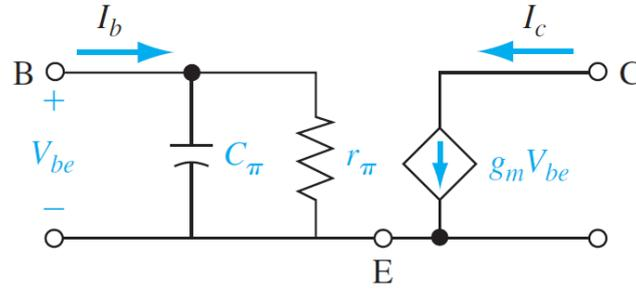
Figure 2.5: Simplified Hybrid-Pi equivalent circuit. [4]
