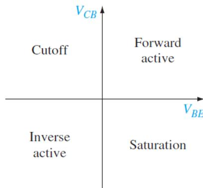
Figure 2.3: Four junction conditions for the four operating modes of a BJT. [4]
