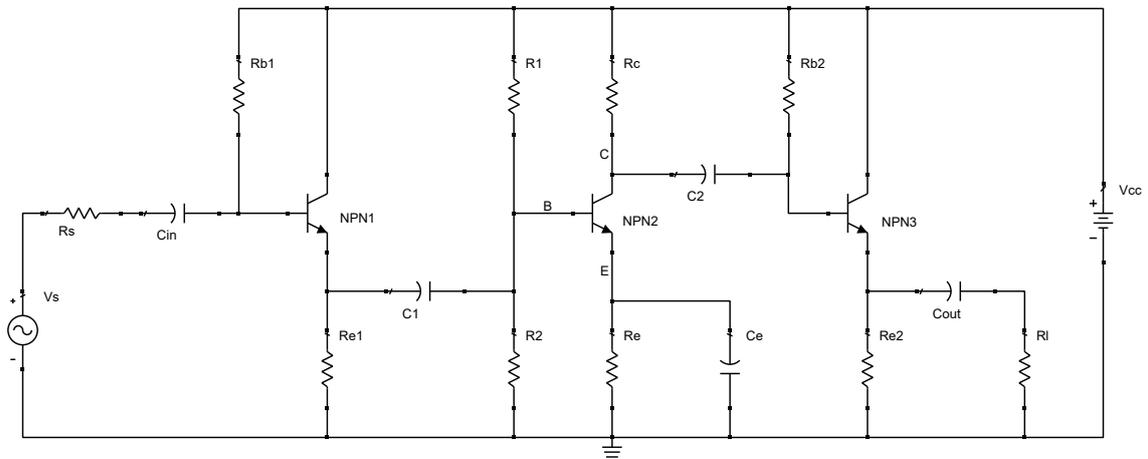
Figure 5.4: Improved design circuit diagram of the microphone amplifier.
