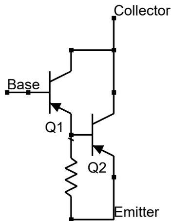
Figure 2.10: Circuit diagrams of a PNP Darlington transistor
