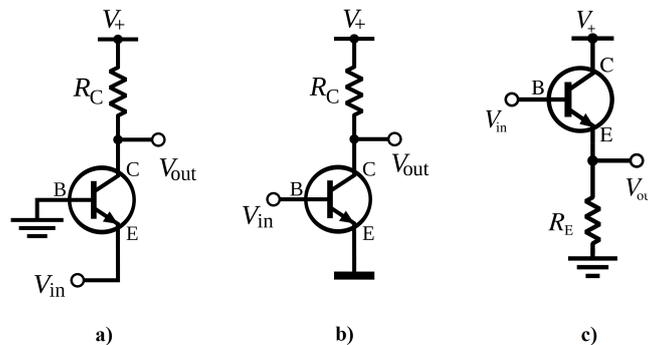
Figure 2.6: Circuit diagrams of (a) common base, (b) common emitter and (c) common collector configurations. (This vector image was created with Inkscape by userOmegatron. This W3C-unspecified circuit diagram was created with the Electrical Symbols Library. This vector image was created with Inkscape, and then manually replaced., CC BY-SA 3.0, <https://commons.wikimedia.org/w/index.php?curid=2802630>)
