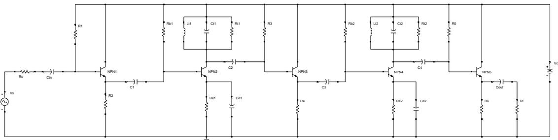
Figure 6.4: Circuit diagram of the IF amplifier.
