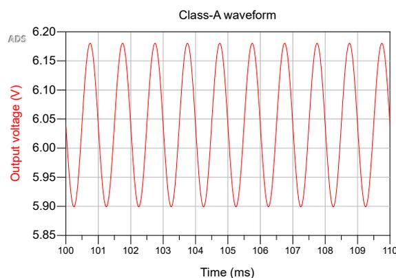
Figure 3.1: Class-A amplifier waveform
