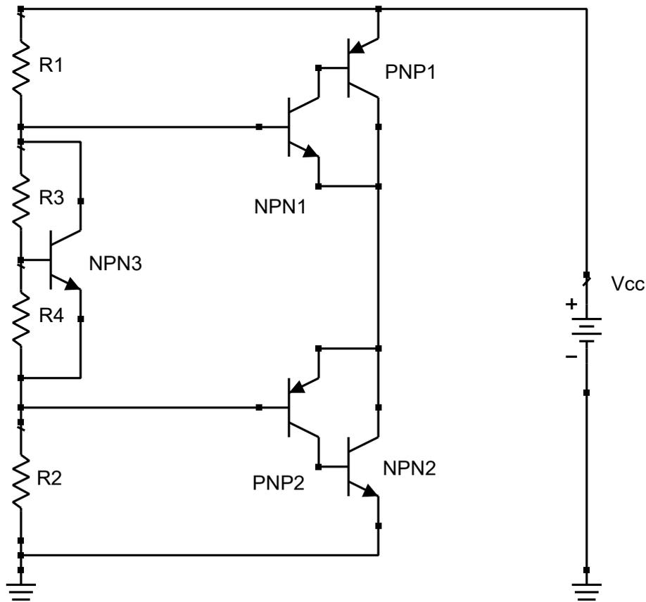
Figure 8.12: DC model of the class-AB amplifier
