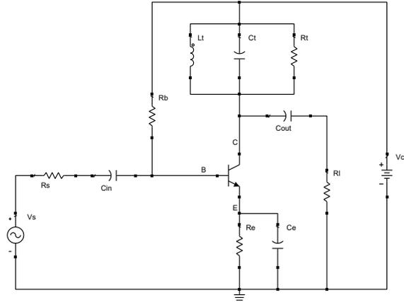
Figure 6.1: Circuit diagram of the bandpass amplifier.
