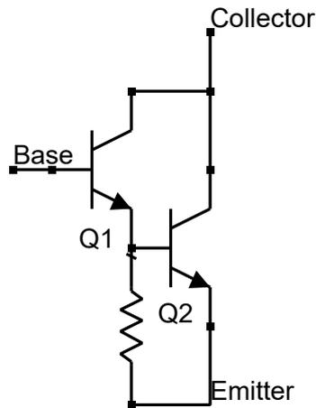
Figure 2.9: Circuit diagrams of a NPN Darlington transistor
