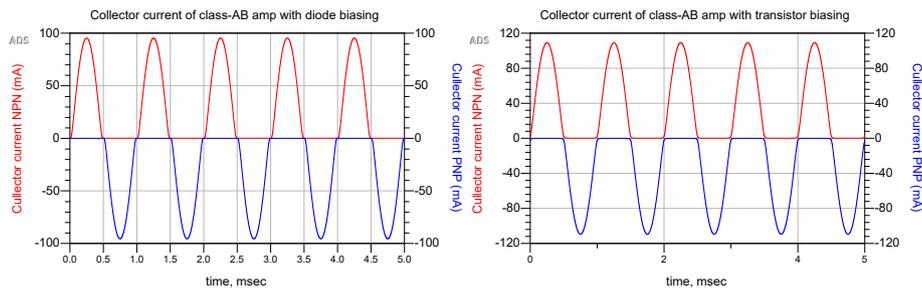
Figure 8.2: Collector currents of two class-AB designs
