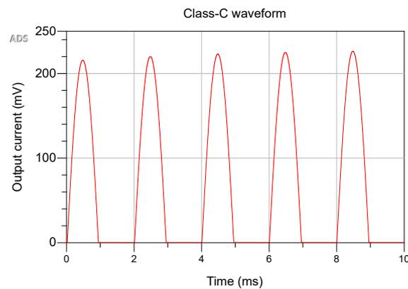
Figure 3.4: Class-C amplifier waveform
