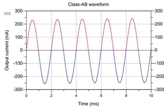
Figure 3.3: Class-AB amplifier waveform
