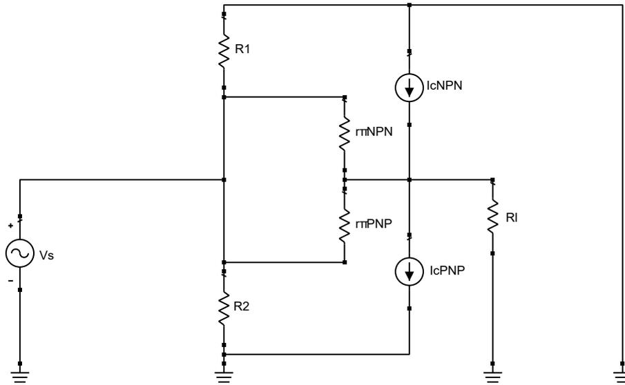
Figure 8.13: AC model of the class-AB amplifier
