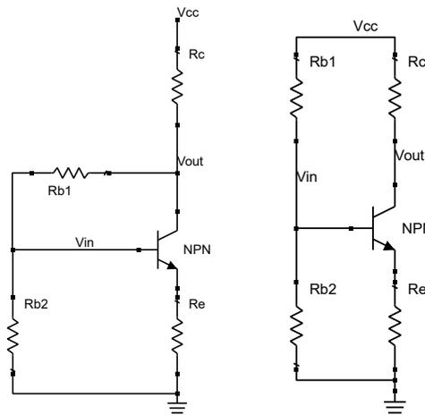
Figure 2.8: Emitter feedback (left) and voltage divider (right) BJT biasing.
