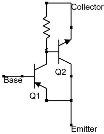
Figure 2.13: Circuit diagrams of a PNP Sziklai transistor
