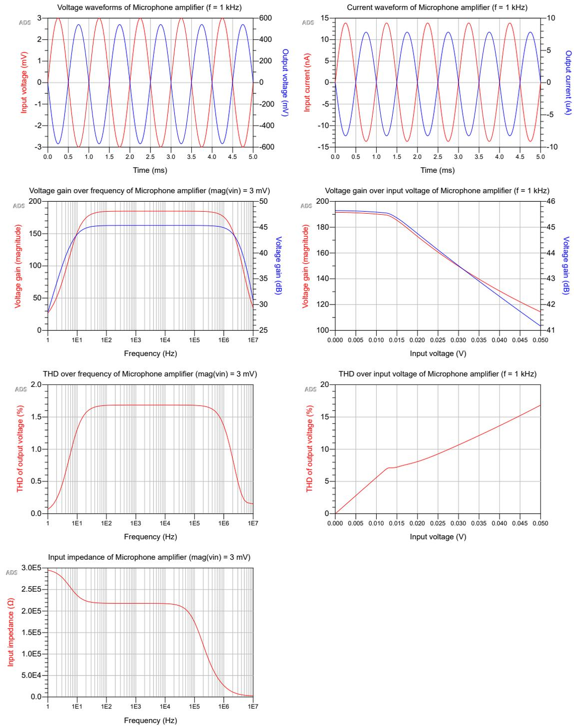
Figure 9.2: Simulation results of the Microphone amplifier.
