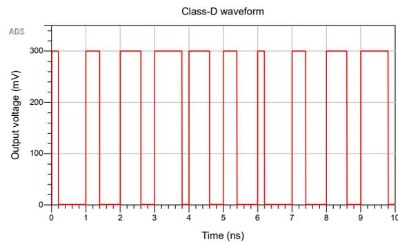
Figure 3.5: Class-D amplifier waveform
